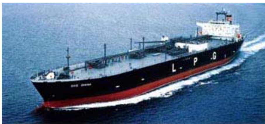
Fig.2-4 LPG carrier of 78,000m 3 capacity "GAS DIANA"
