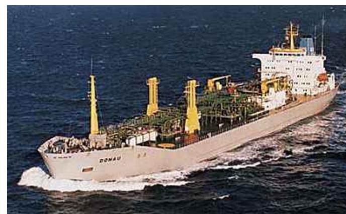
Fig.2-5 Semi Pressurized LPG carrier of 30,207m 3 capacity "DONAU"
