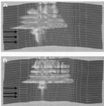
Numerical flow simulation of CO<sub>2</sub> injection at Sleipner Field, which has been history matched with time lapse 3D seismic reflection data. Two perpendicular cross-sections of a simulation result are shown (A & B). Intra-formational seals act as barriers to vertical scCO<sub>2</sub> migration (van der Meer et al., 2000).
