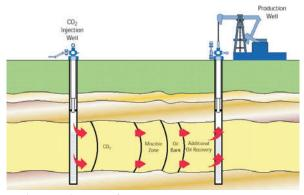
Schematic diagram of CO<sub>2</sub>-EOR
