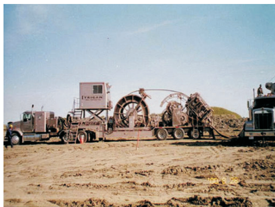
Seismic monitoring : the truck that carries the coil-tubing used to deploy the seismic instrumentation down the borehole.
