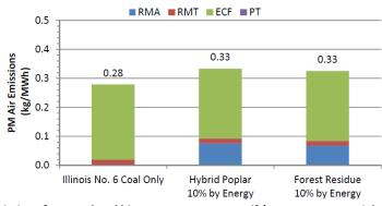
Fig. 6 Life cycle PM emissions from coal and biomass power systems<sup>13</sup> (RMA = raw materials acquisition, RMT = raw materials transport, ECF = energy conversion facility, PT = product transport)
