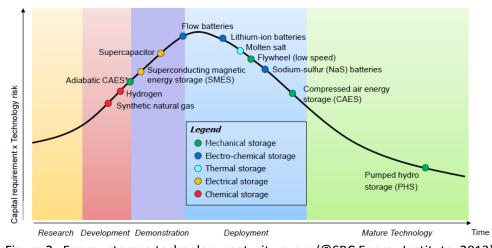
Figure 2 Energy storage technology maturity curve (©SBC Energy Institute, 2013) Over 99% of the installed grid-connected storage capacity is currently pumped storage hydro, as shown in Figure 3, but the limited availability of suitable sites is a constraint on future capacity additions in many areas.
