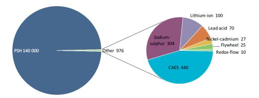
Figure 3 Current global installed grid-connected electricity storage capacity (MW), (IEA, 2014) (PSH: Pumped storage hydro, CAES: Compressed air energy storage)
