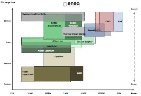
Figure 1 Energy storage according to discharge time and typical power (ENEA, 2012) (PSH: Pumped storage hydro, CAES: Compressed air energy storage, SMES: Superconducting magnetic energy storage)
