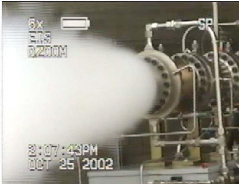
**CES 20 MW<sub>t</sub> Gas Generator – 100 bar & 850 °C**
