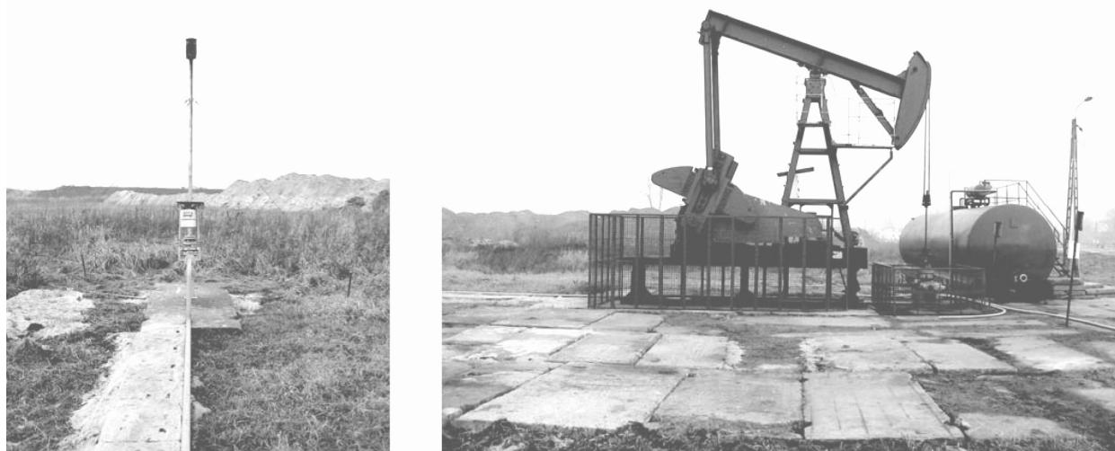
Figure 15: Picture of the MS-4 production well and pump. The gas is flared (left), while the water is transported by truck to a disposal site.
