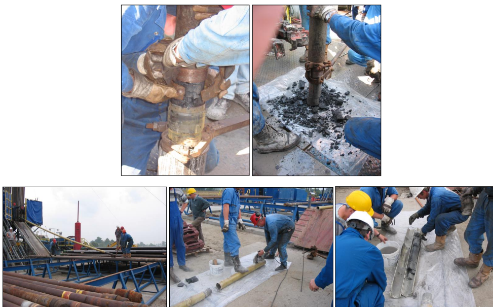
Figure 17: Pictures of coring activities. Top pictures are from the first core, which was relatively unsuccessful. Bottom pictures show the successful recovery of the 405 core by cutting the core barrel in half.
