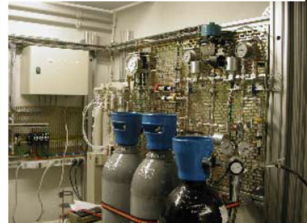
Low and High Pressure CO 2 Supply
