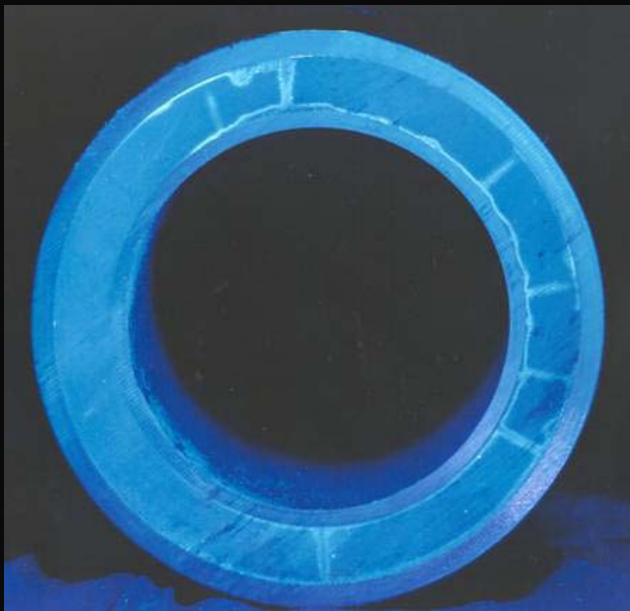
Damaged Cement Sheath
