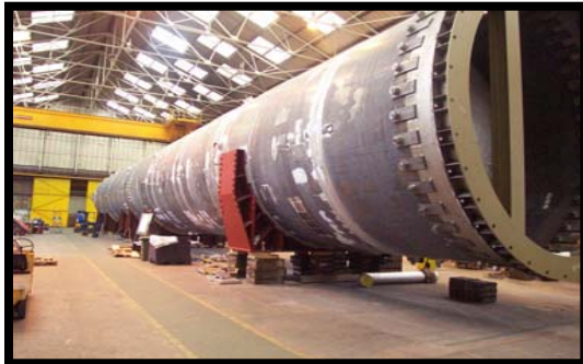
Shop manufactured distillation columns
