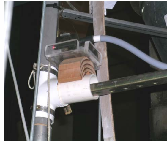
Laser Solids Velocity Probe
