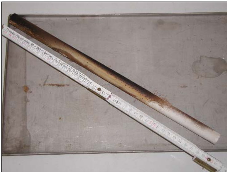
Slag deposition probe (after 3:20 hr)
