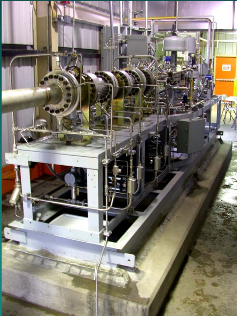
20 MW t Combustor
