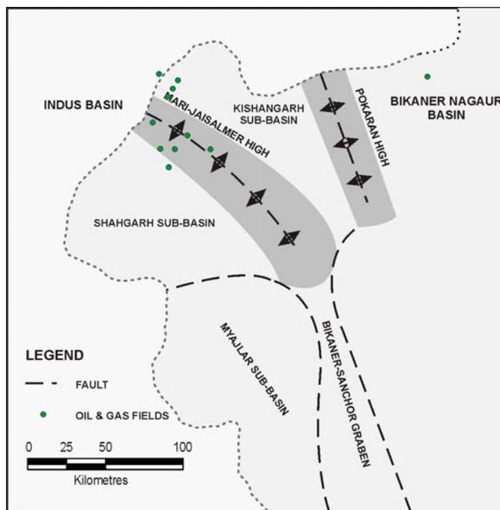
**Figure A3. 9 Structural elements of the Jaisalmer Basin (adapted from Uniyal et al. 1997, Srivasatava et al. 1995, Ministry of Petroleum and Natural Gas 1991).**
