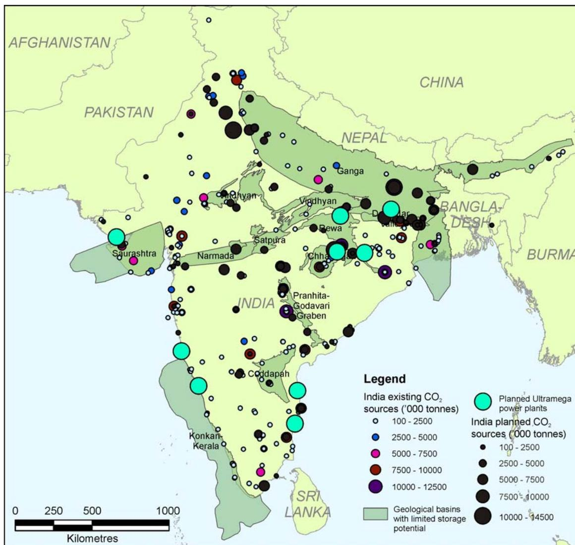
**Figure 2.8 India's existing and planned CO<sub>2</sub> sources and geological basins with limited storage potential**
