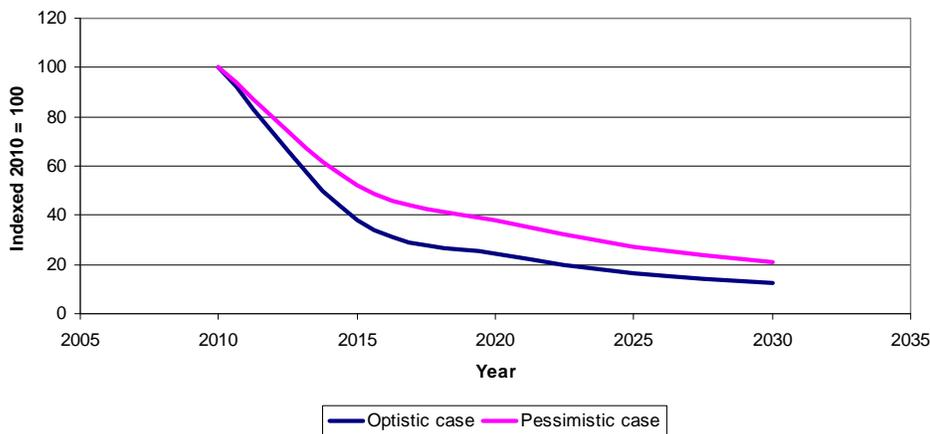
**Figure 2.12 Future cost development of fuel cell vehicles, source IEA 2005**
