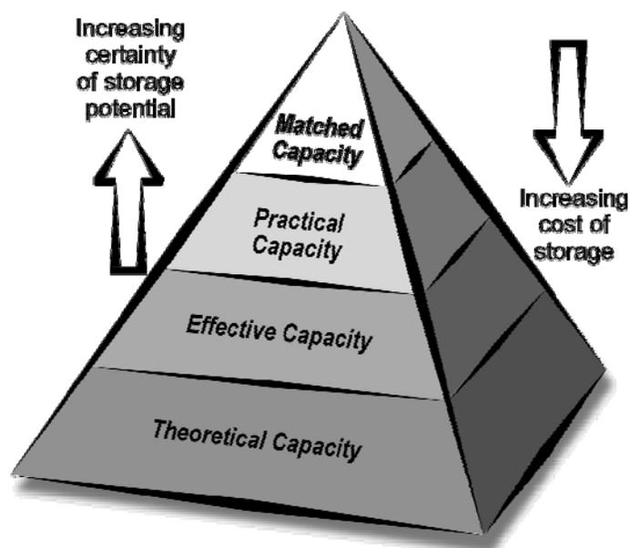
**Figure A1.1. CO<sub>2</sub> storage capacity resource pyramid (after Bachu et al. 2007)**
