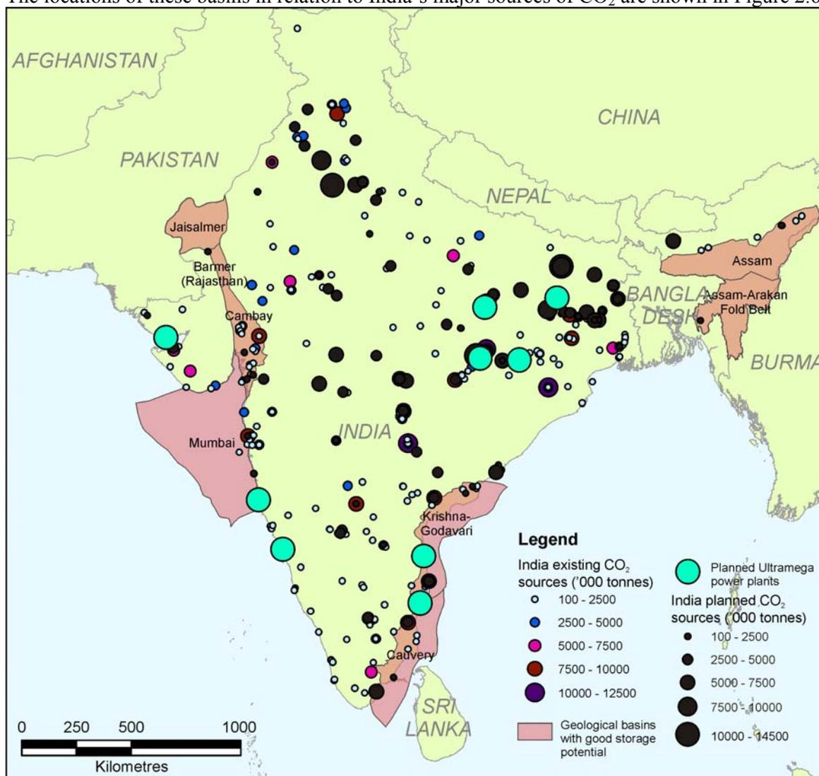
**Figure 2.6 India's existing and planned CO<sub>2</sub> sources and geological basins with good storage potential**
