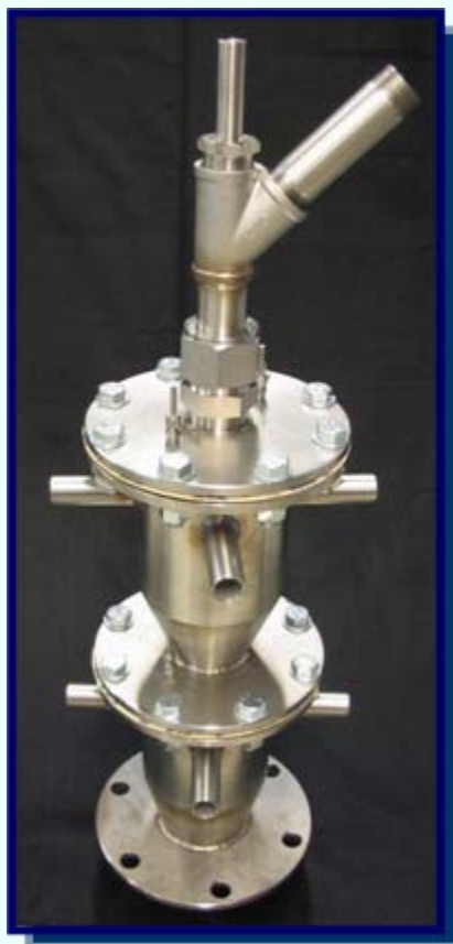
1 st Generation: Fixed-Angle Swirl Generator
