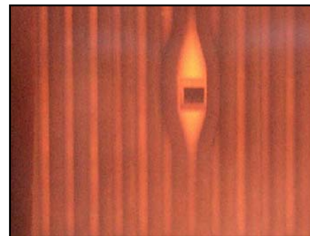
Existing measurement port
