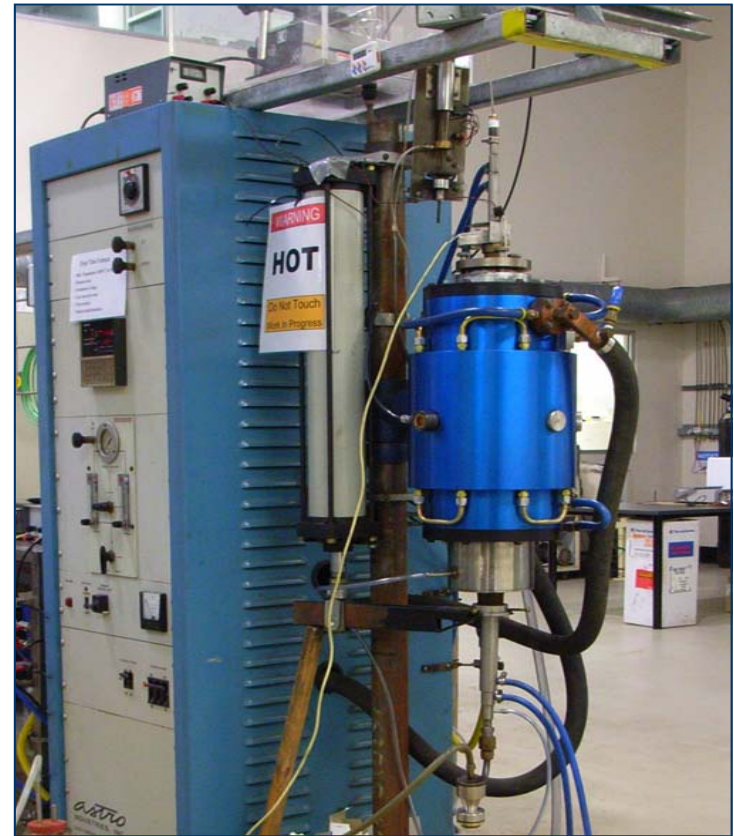
DTF – High temperature reactivity measurements
