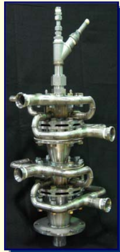
2 nd Generation: Variable-Angle Swirl Generator
