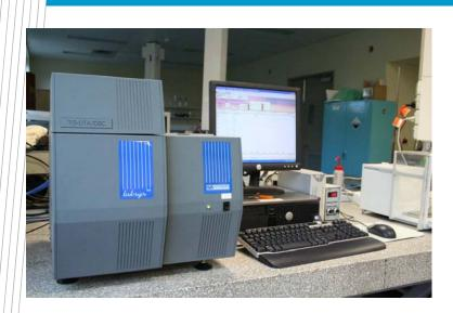
Gravimetric method used to measure  $CO_2$  absorption and initial absorption rate on  $\mu L$  scale
