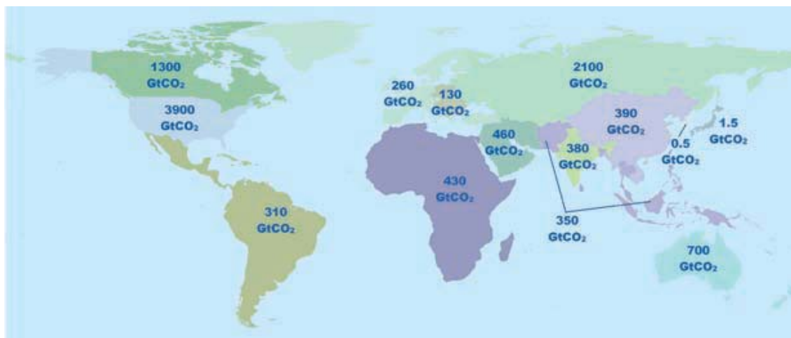
Figure 5. First-order assessment of the global theoretical CO 2 storage capacity, approximately 90 % of which is in saline formations (Dooley et al., 2006).
