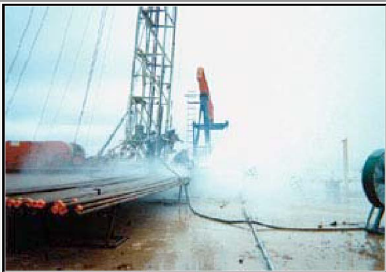
Fig. 2. Vapor cloud from water in the air condensed by cold CO 2 reduces visibility near wellbore, hindering hand-signal communications.
