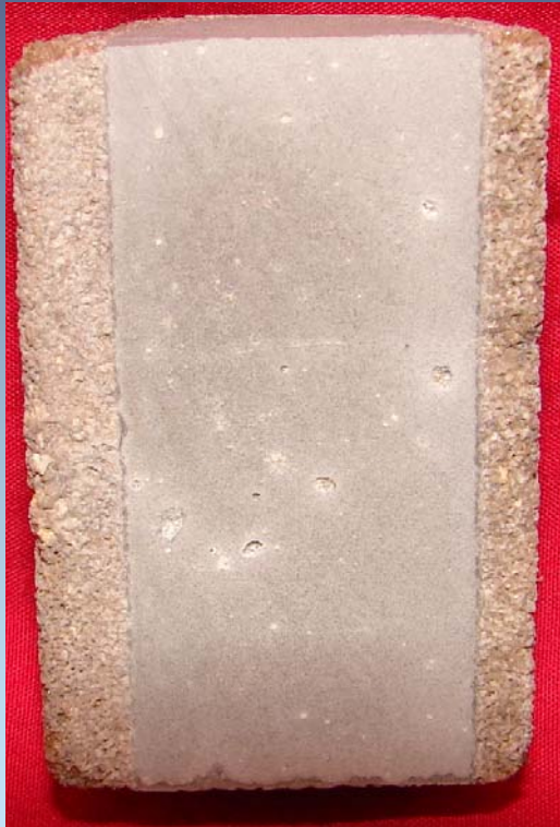
Calcium Aluminate Systems Resist Carbonic Acid Up to 600F at pH<3
