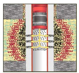
Figure 4: Demonstrating the most secure method of cased hole abandonment. This is injection of a cement into the retainer and application of pressure to squeeze the cement to form a seal at the sand face, perforations and wellbore. This ensures that the seals between the various elements of the wellbore are sealed against CO<sub>2</sub> ingress as effectively and securely as possible, without the wellbore being cemented to the surface.
