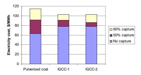
Figure 1 Costs of electricity with 90%, 50% and no CO<sub>2</sub> capture
