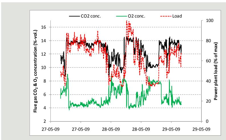
Example: 48-hours load profile at the Esbjerg coal-fired power plant
