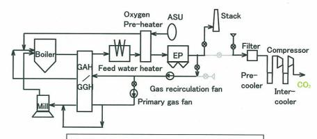
Combustion mode change: Air -> Oxy Load change: 300MW -> 600MW Fuel change: Light oil -> Coal Preparation of CO2 compression unit
