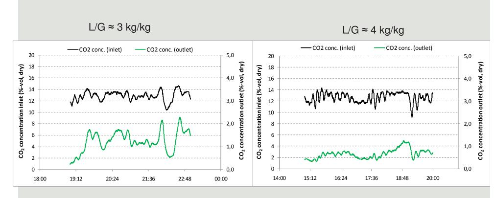
Examples: 4-hours operating period with fixed settings at the CO<sub>2</sub> capture plant
