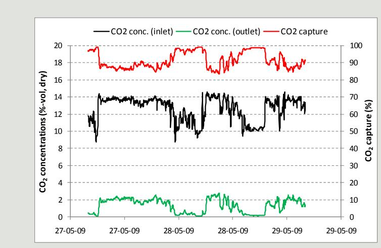
Example: 48-hours operating period with fixed settings at the CO<sub>2</sub> capture plant
