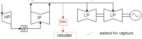
Avoids all throttling losses at design extraction rate.
