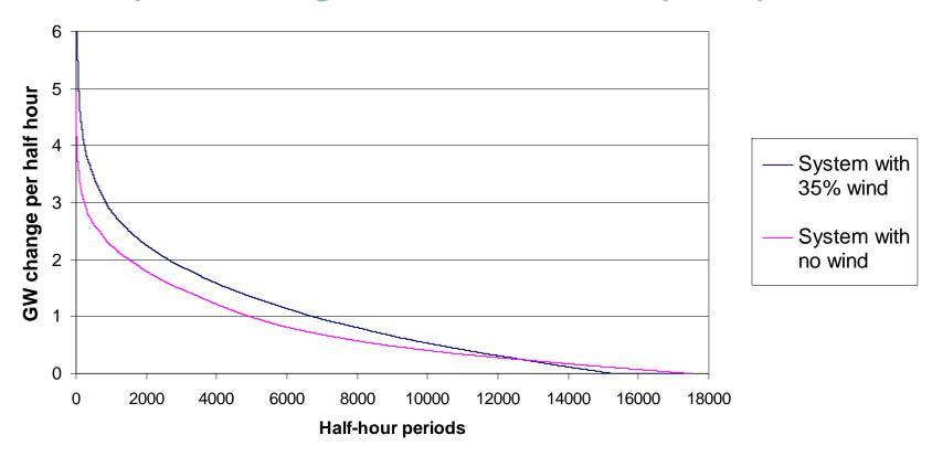
Basis: UK power demand (maximum 59GW) 22% of generation from 'inflexible' plants Wind output scaled from current system output
