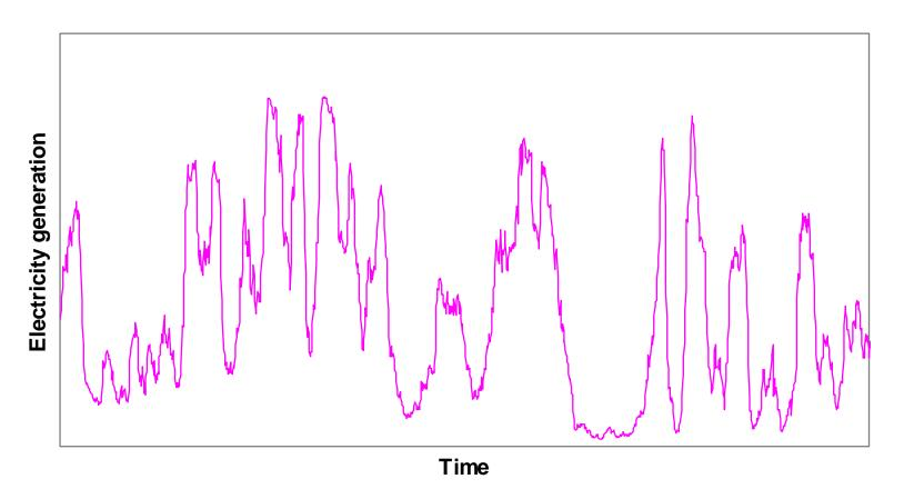
HV grid connected wind in the UK, May 2009
