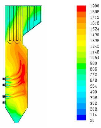
Oxyfuel Firing Furnace Temperature Profile
