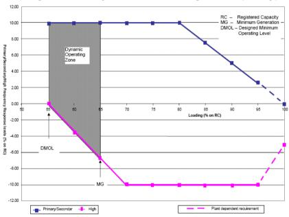
The IGCC plant should be capable to provide Primary Frequency response at least to the solid boundaries shown in the figure (NG cofiring or syngas storage are the only options)
