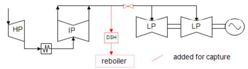
Simplest design, but losses in throttling valve. Initial pressure ~3.6 bar for amine, cannot be varied
