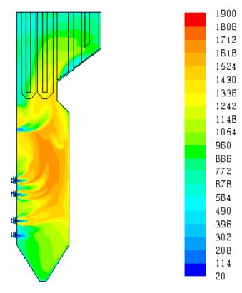
Air Firing Furnace Temperature Profile
