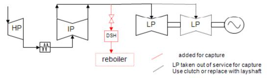
Most efficient design, but cannot vary steam extraction flow. Initial pressure ~3.6 bar for amine, cannot be varied
