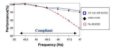
CASE 2: With Air Bleed (to vent) on Gas Turbine
