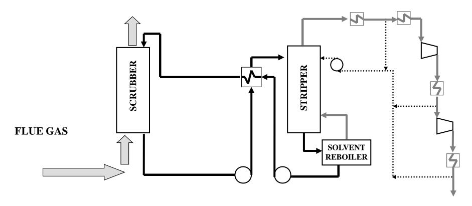
Change in flue gas flow-rate - Optimal Absorber L/G ratio? Change in solvent flow-rate - Optimal Stripper L/G ratio? Temperature of regeneration — Compressor operation  $CO_2$  output drops - Compressor operation Temperature pinch in solvent reboiler
