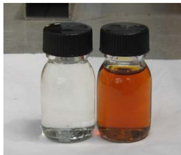
MEA at 40 wt % after 1000 h pilot test (with and without inhibitor)
