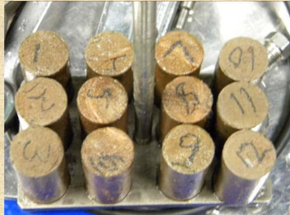
Cement cylinders (1" dia, 2" length) exposed to CO 2 for up to 6 months
