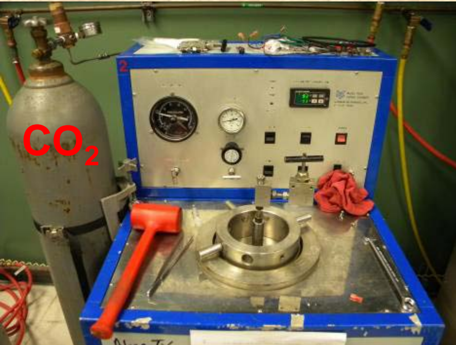
HTHP curing chamber connected to a CO 2 bottle
