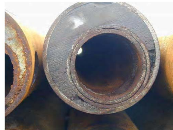
Figure 5-5: Close up of 7 and 10 3/4-in. Casing on the Rack
