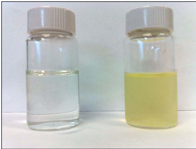
CO 2 loaded PZ solution (LHS) After exposure to synthetic flue gas (RHS)
