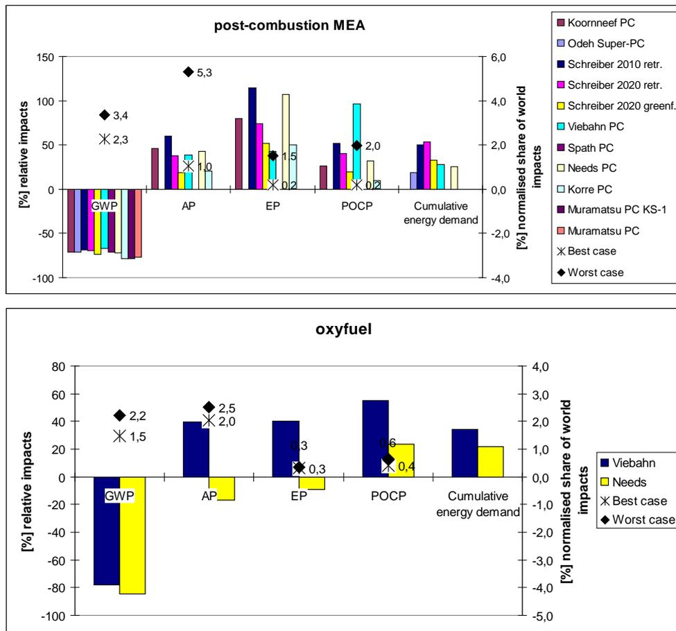
**Figure 4-10: Environmental impacts of hard coal fired pulverised coal combustion technology a) without capture and b) relative impacts for plants with post-combustion/MEA or oxyfuel capture and normalised values related to the total world production in 2000 calculated for lowest and highest impact values**
