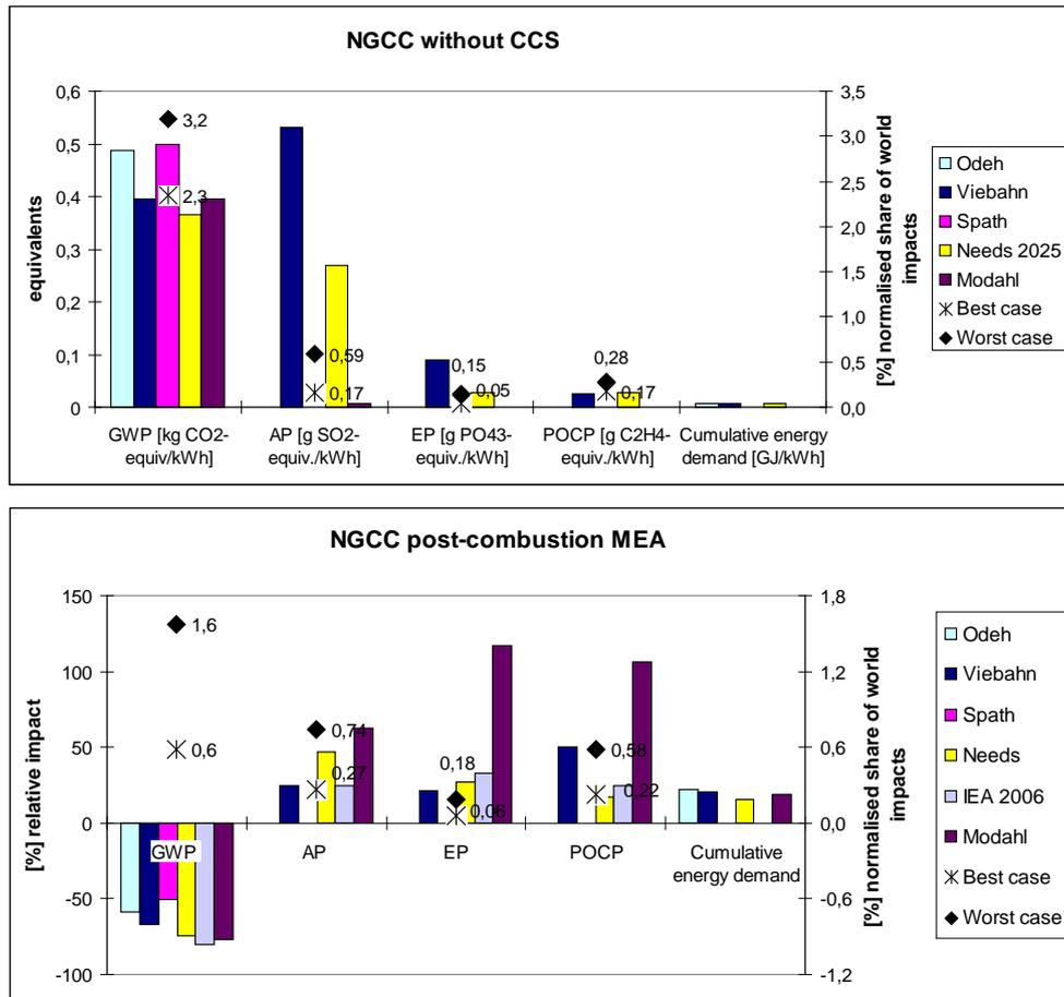
**Figure 4-14: Environmental impacts of a natural gas combined cycle without capture and relative impacts of systems with post-combustion capture and normalised values related to the total world production in 2000 calculated for lowest and highest impact values**
