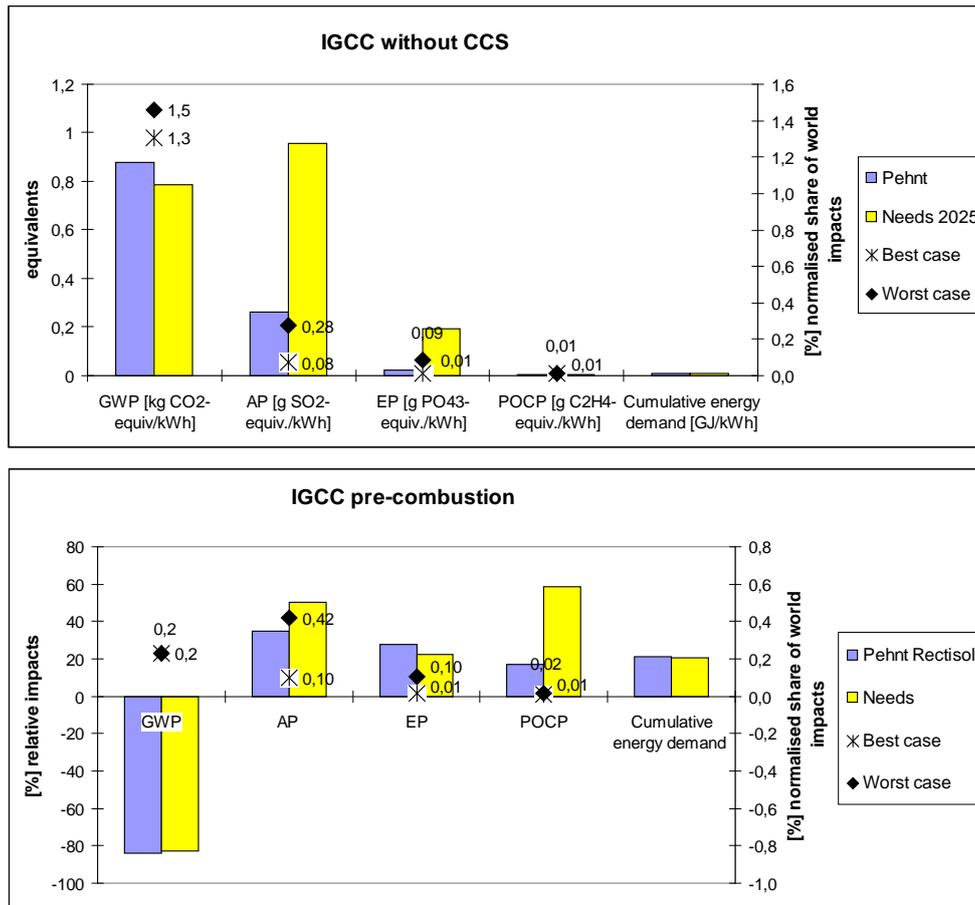
**Figure 4-13: Environmental impacts of an integrated coal gasification system without capture and relative impacts of systems with pre-combustion capture and normalised values related to the total world production in 2000 calculated for lowest and highest impact values**
