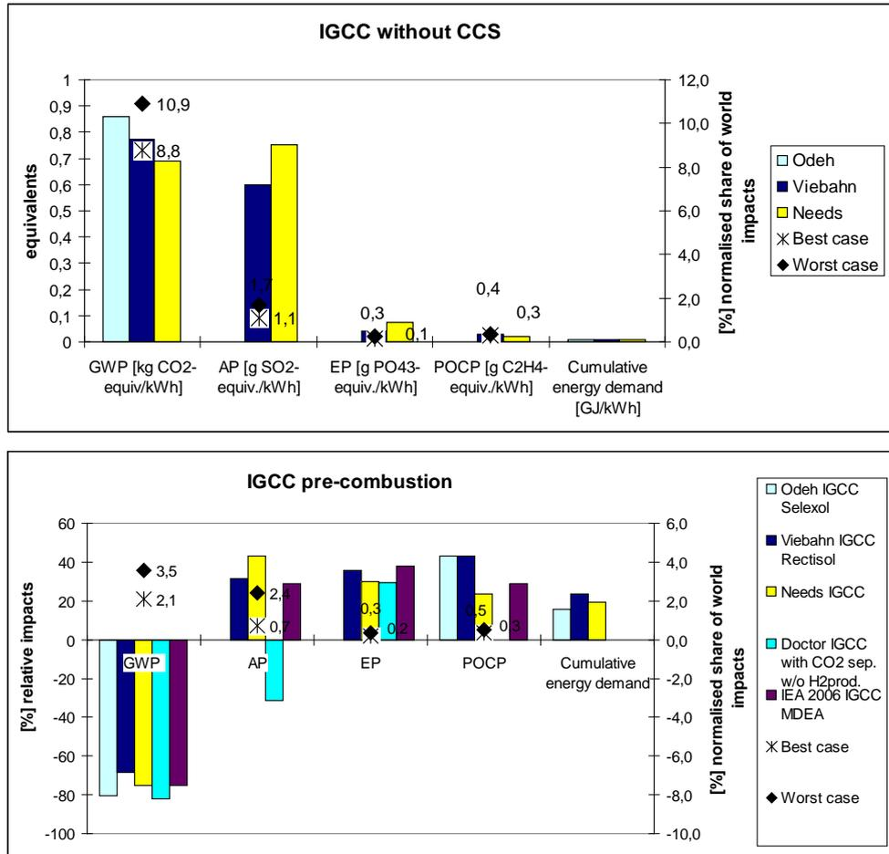
**Figure 4-11: Environmental impacts of an integrated coal gasification system without capture and relative impacts of systems with pre-combustion capture and normalised values related to the total world production in 2000 calculated for lowest and highest impact values**
