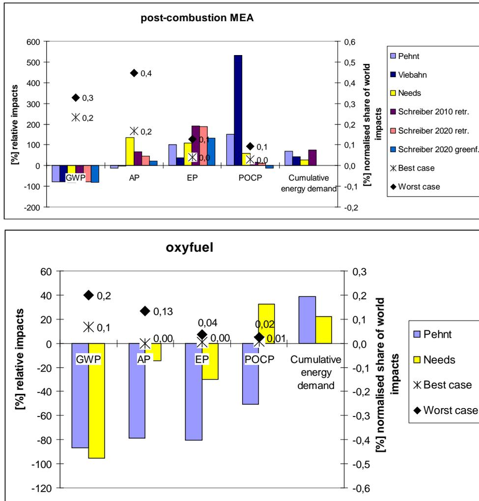
**Figure 4-12: Environmental impacts of lignite powered pulverised coal combustion technology a) without capture and b) relative impacts for plants with post-combustion/MEA or oxyfuel capture and normalised values related to the total world production in 2000 calculated for lowest and highest impact values**
