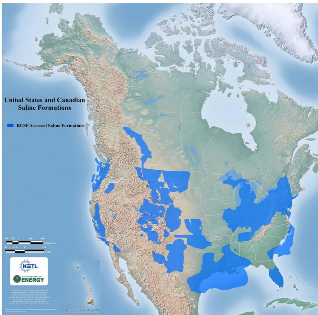
Figure 2.2: Location of assessed deep saline formations in N. America (from DOE NETL, 2010). Note that saline formation data resulting in a straight edge in the map above is indicative of an area lacking sufficient data and is subject to future investigation.
