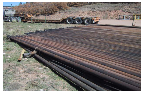
Extracted Pipes used in CO 2 Injection – showing no serious degradation despite long exposure to CO 2
