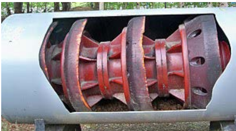
Figure 19 – An example of a (non-intelligent) pig in a pipeline
