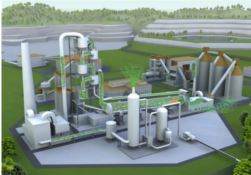
Figure 4-5 Potential design of a cement plant with chemical absorption technologies for CO 2 capture (green: nitrogen, blue: oxygen and black: CO 2 ) [ECRA website: www.ecra-online.org ]
