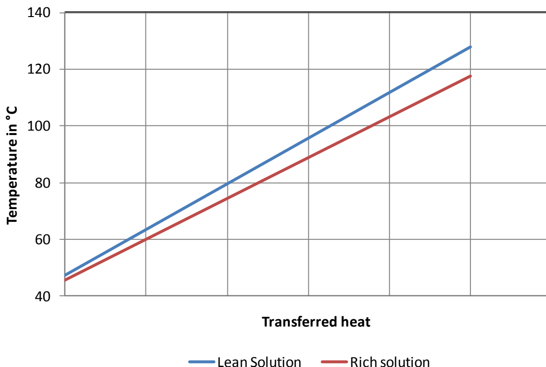
Figure 53: Simplified temperature profile in the RLHX for the base case
