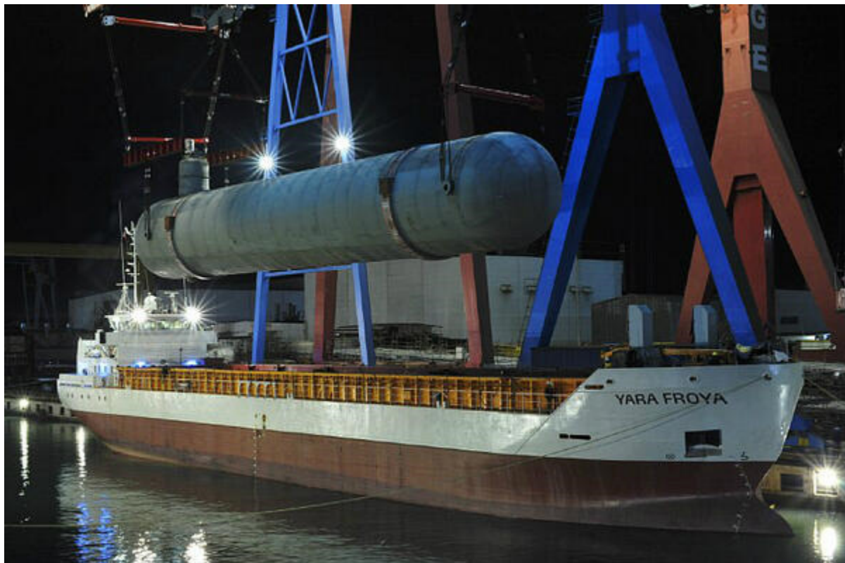
Figure 2 Yara Froya during installation of Type C cargo tank for CO2 carriage (source: Yara International)
