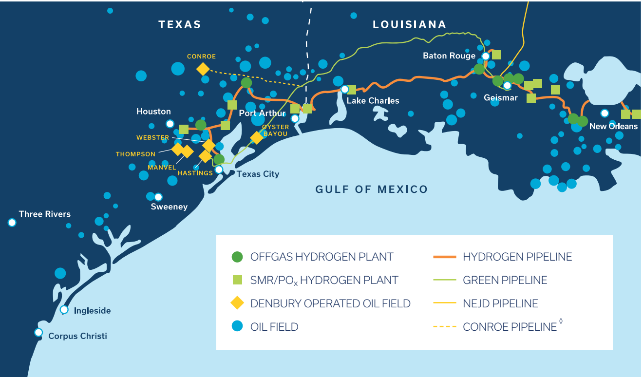
FIGURE 3 | APCI AND DENBURY RESOURCES OPERATIONS IN THE GULF COAST REGION, SHOWING THE GCCP, HYDROGEN PLANTS, CO₂ PIPELINES AND TARGET CO₂-EOR OIL FIELDS [Sources: Baade et. al., 2012 and Denbury, 2016]
