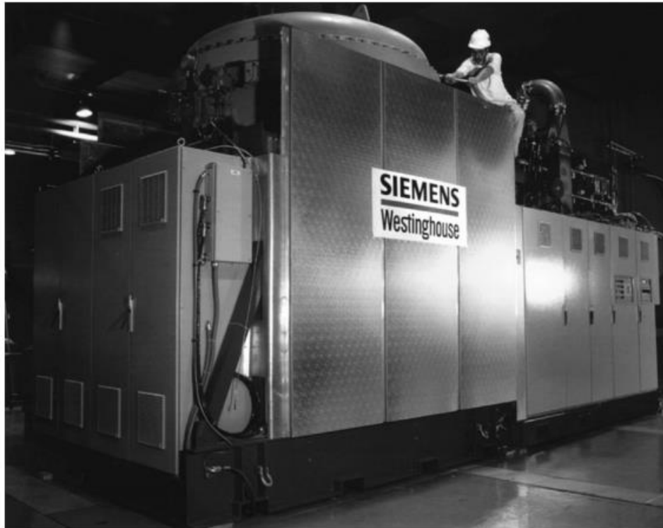
Figure 36: The hybrid SOFC – GT system developed by Siemens – Westinghouse (Maurstad, et al., 2005)
