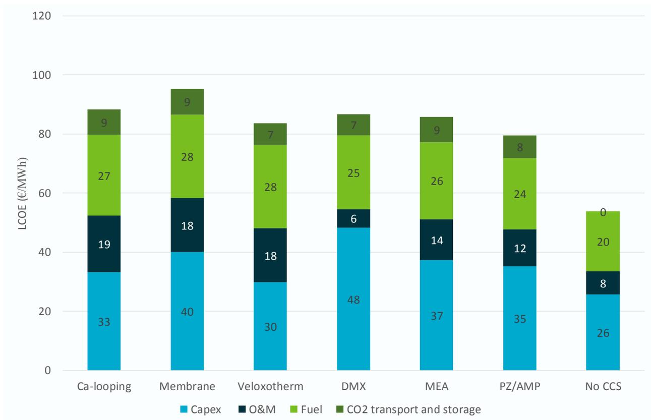
**Figure 24 Breakdown of the base case LCOEs of coal-fired technologies into components**
