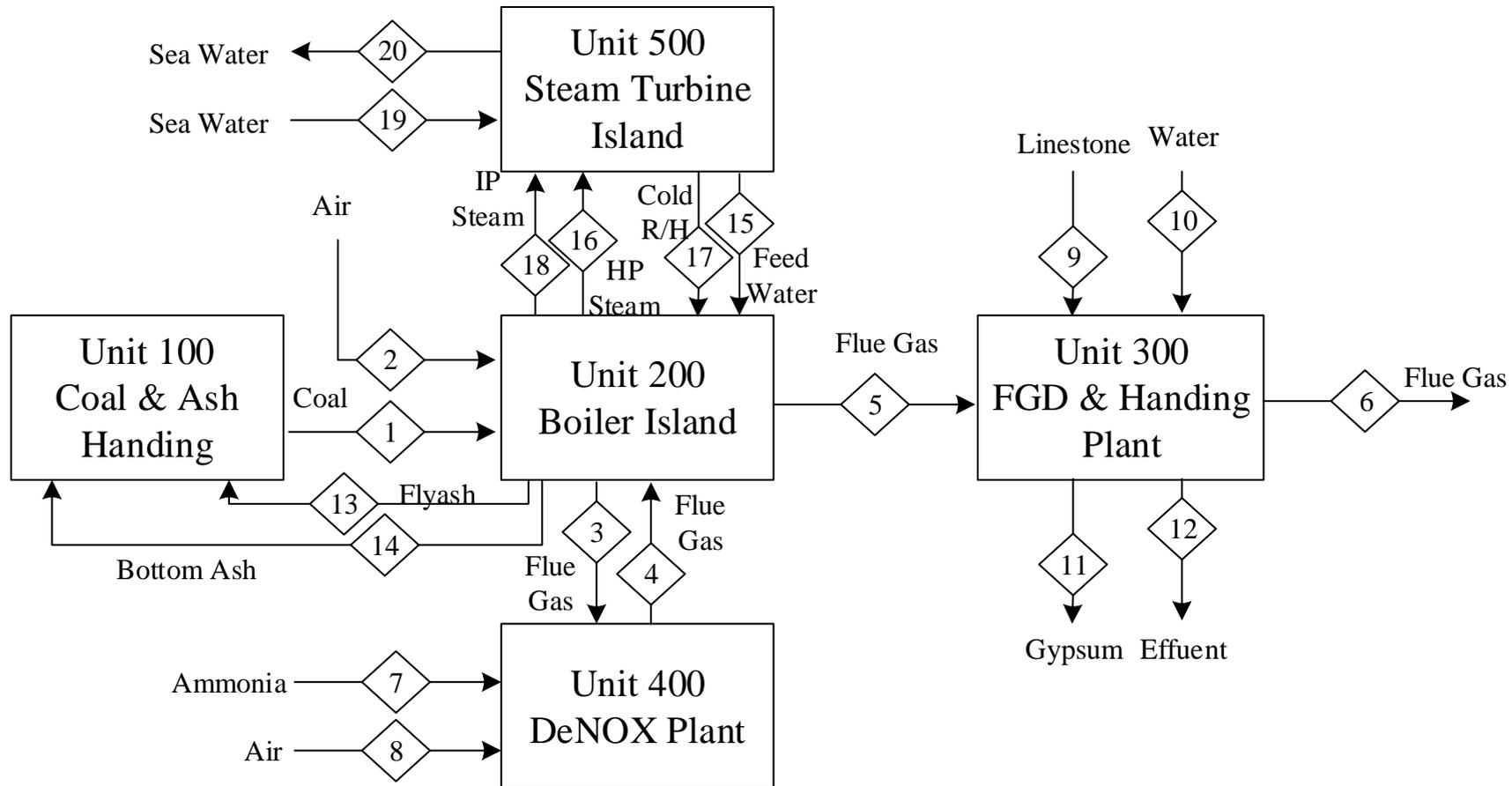
Apx Figure A.5 USCPC power plant with once-through (OT) seawater cooling (Case 1.2A: USCPC-OT)
