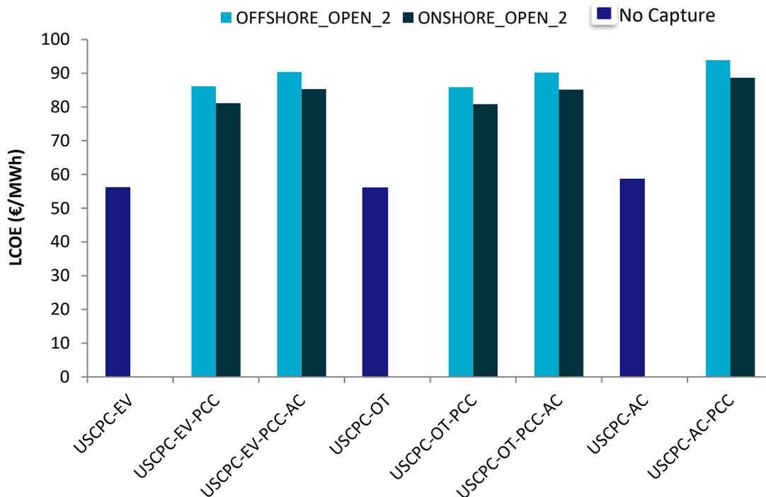
**Figure 5-1 LCOE of USCPC power plants without (USCPC-EV, USCPC-OT, USCPC-AC) and with CCS in saline formations with open reservoir boundaries onshore and offshore Netherlands**
