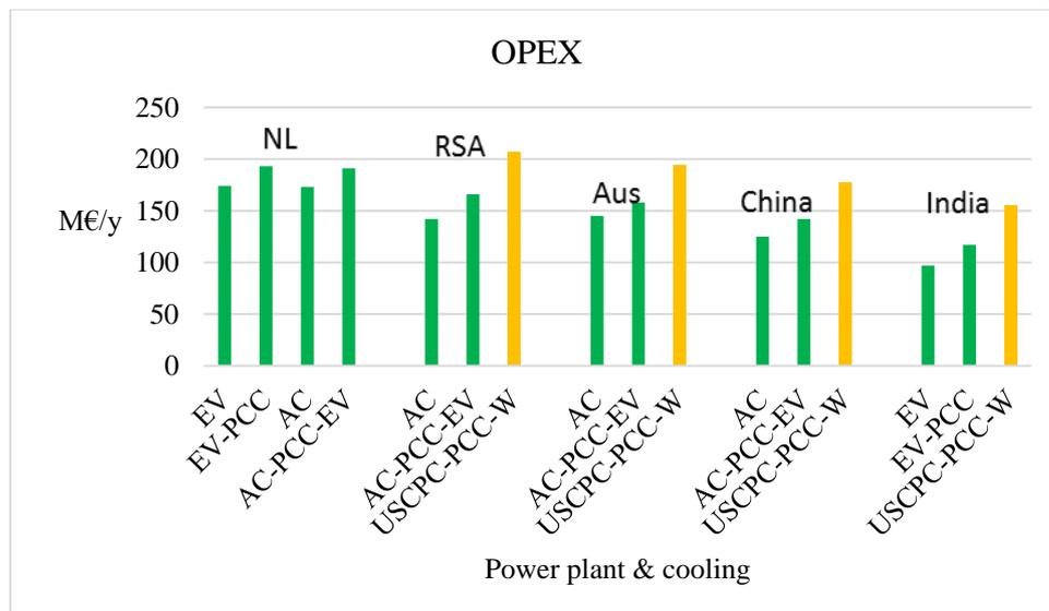
**Figure 5** Operational costs of the base case reference power plant (NL) and the four selected countries, with and without CO<sub>2</sub> capture plant and with incorporated water treatment (-W). (NL = The Netherlands, RSA = Republic of South Africa, AUS = Australia).
