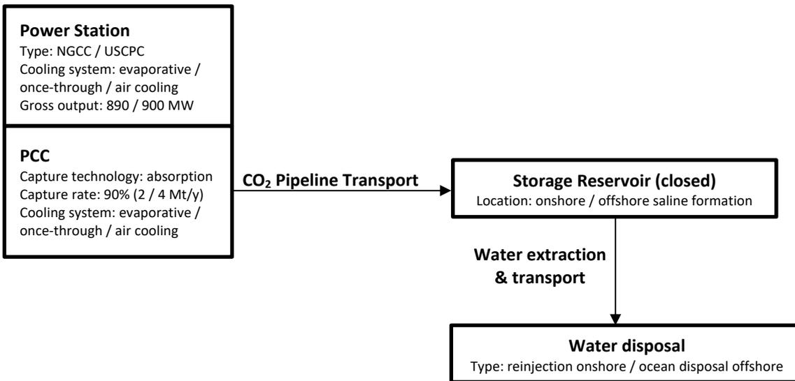
Figure 1 Flow diagram of the two cases of the Base Case CCS Scenario: a) CCS in an open formation without water extraction; b) CCS in a closed formation with water extraction and disposal
