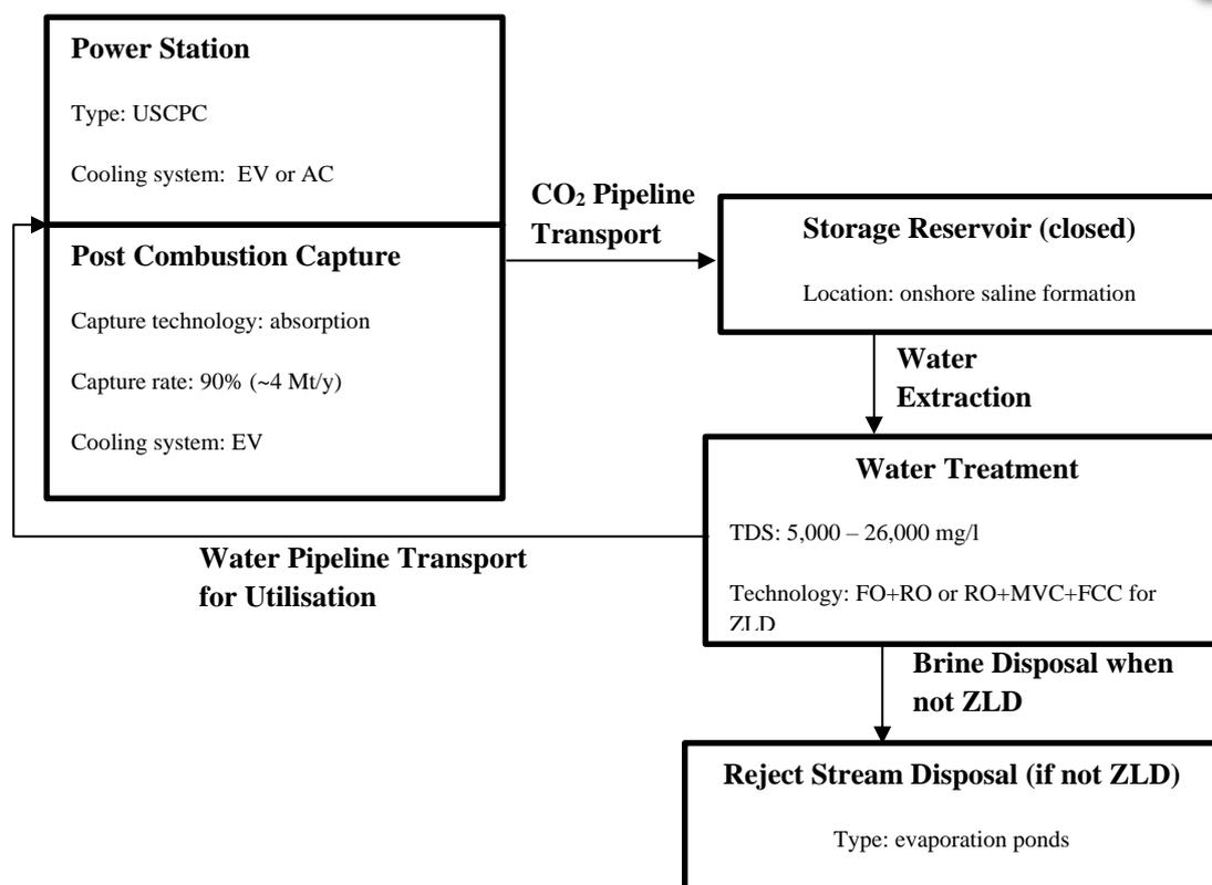
**Figure 3** Flow diagram of the Energy-Water-CCS nexus Scenario with water treatment and utilisation in the power station with capture and other beneficial use (FO = forward osmosis, RO = reverse osmosis, MVC = mechanical vapour compression, FCC = forced circulation crystallizer, ZLD = zero liquid discharge)
