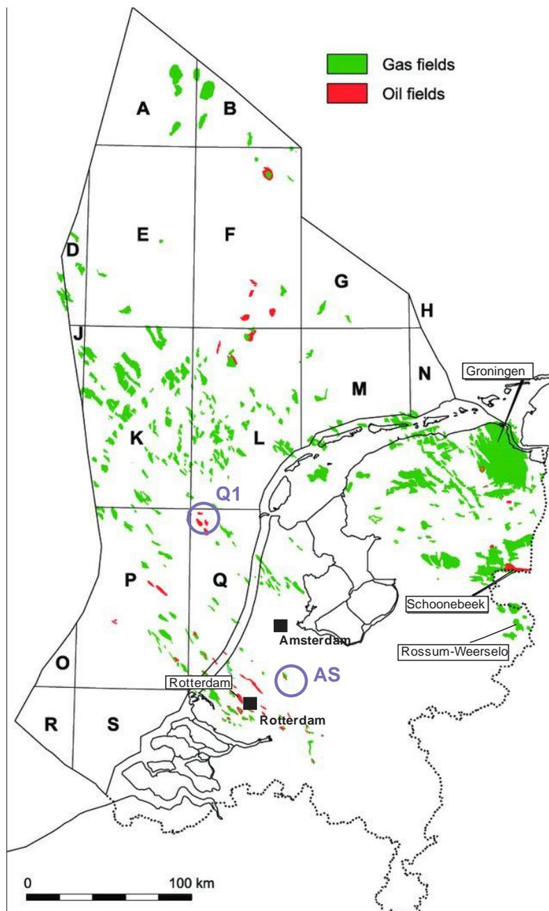
Figure 3-23 Location of oil and gas fields in the Netherlands. The four fields with the largest water injection onshore are labelled (see Table 3-9). The two potential CO<sub>2</sub> storage sites are identified by purple circles
