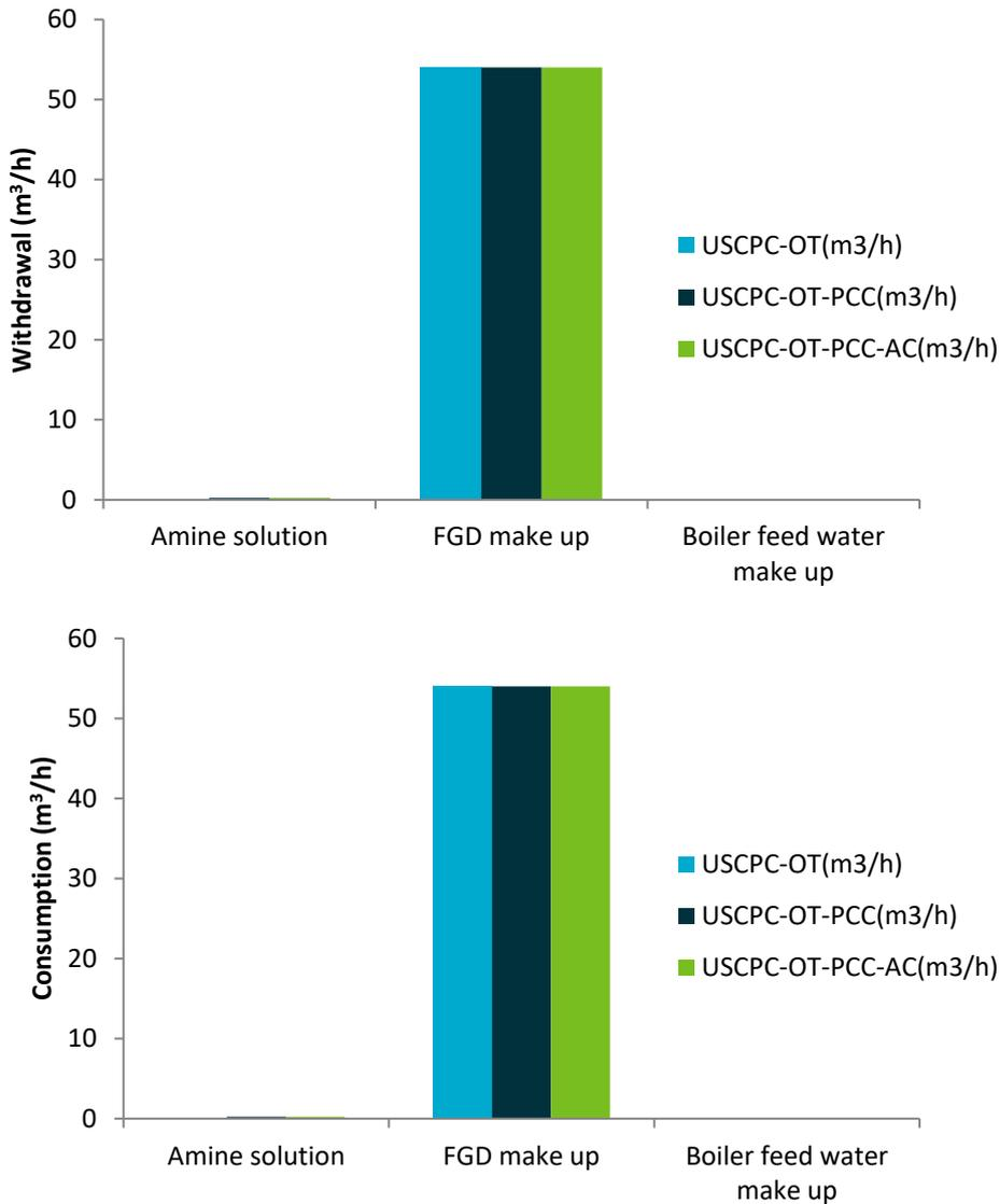
**Figure 2-7 Absolute water withdrawal and consumption rates for the USCPC using once-through seawater cooling systems comparing Case 1.2A (USCPC-OT), Case 1.2B (USCPC-OT-PCC), and Case 1.2C (USCPC-OT-PCC-AV)**
