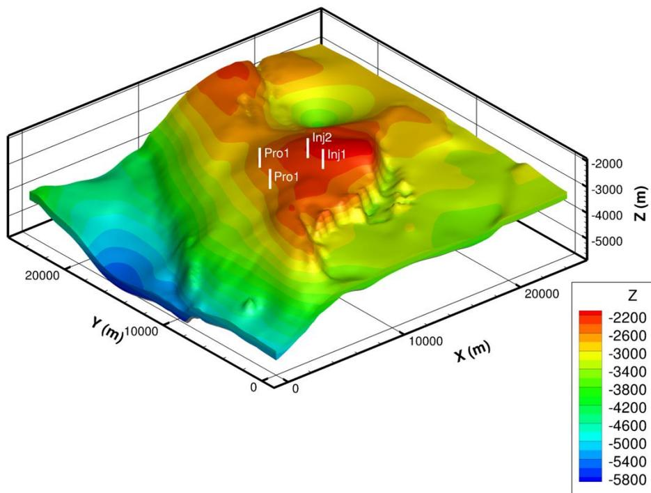
**Figure 3-2 Computational reservoir model of the offshore aquifer in the Q1 block. Contours indicate depth in metres. Injection and production well locations shown**
