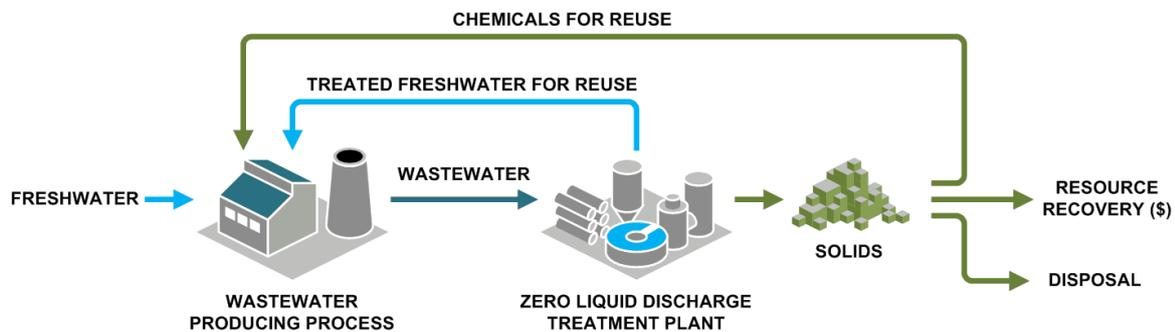
Figure 1-5 Schematic of zero liquids discharge at an industrial facility (Saltworks, 2019)
