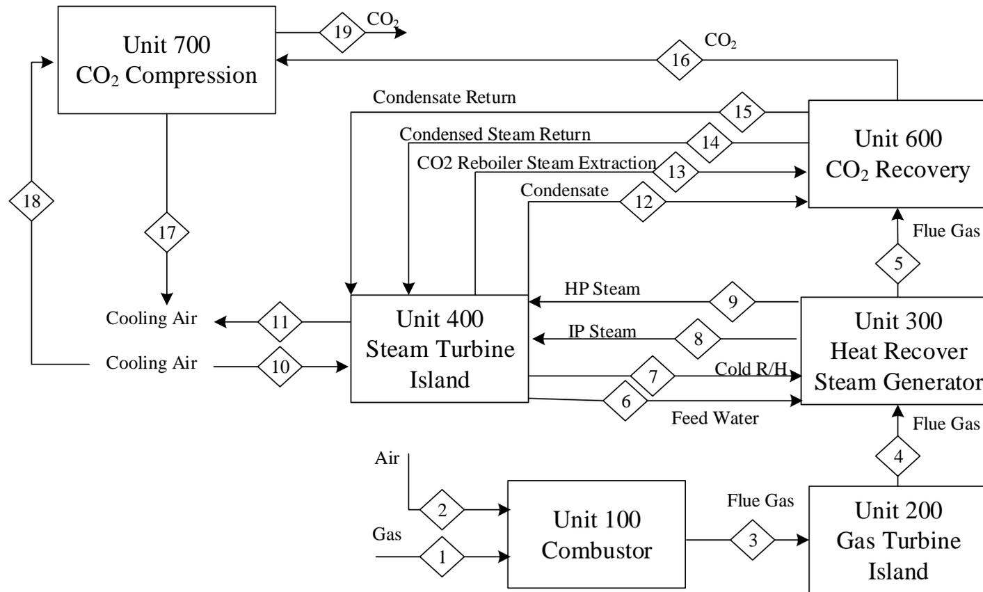
Apx Figure A.31 NGCC power plant with capture using air cooling (AC) (Case 2.3B: NGCC-AC-PCC)
