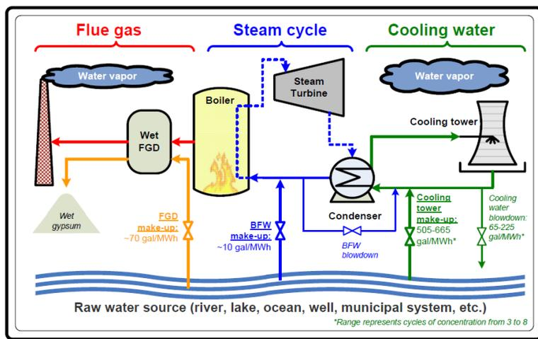
Figure 1-2 Water schematic at a coal fired plant (with wet-cooling tower) (DOE-NETL, 2009)
