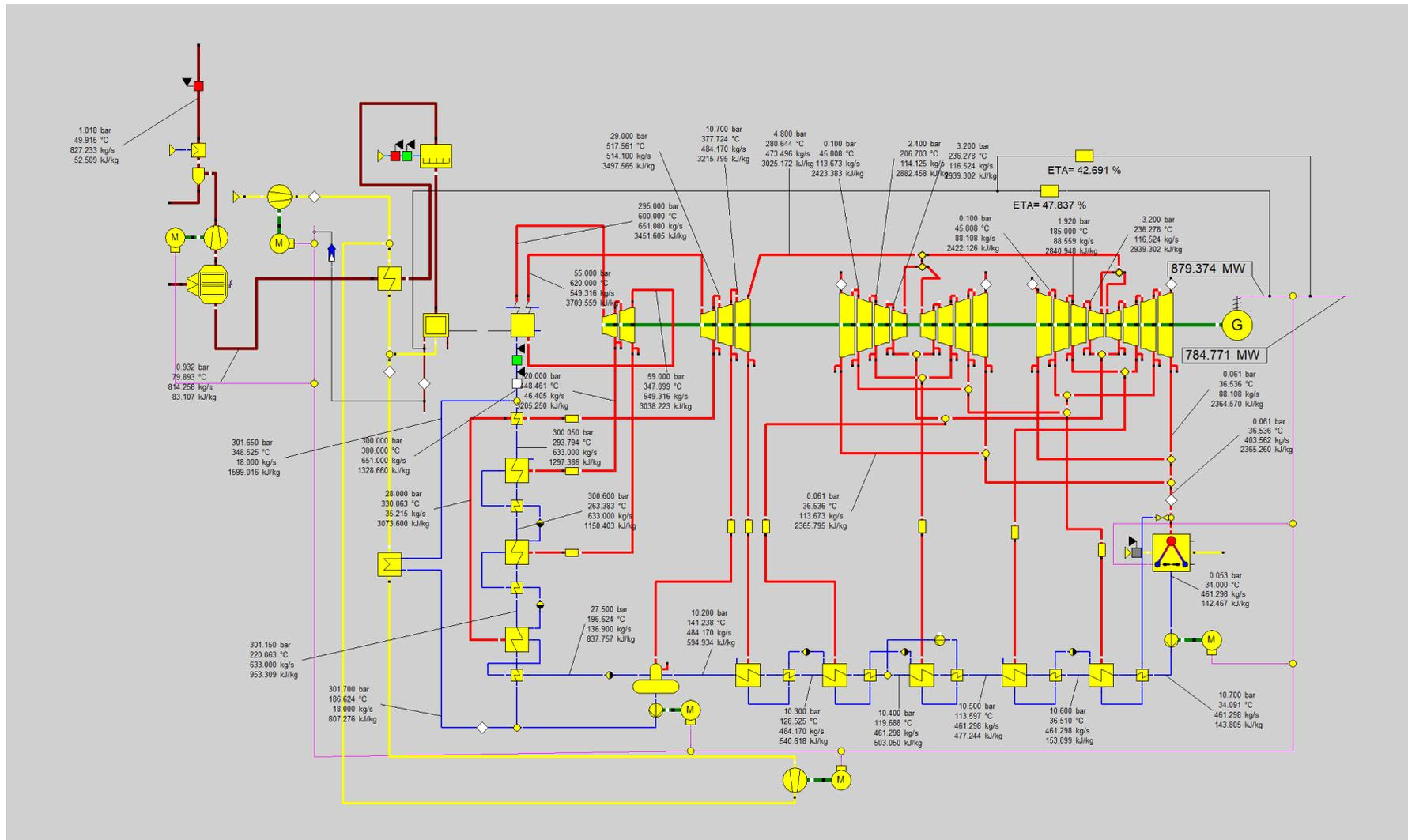
Apx Figure A.10 Flow diagram of the USCPC power plant process using air cooling (AC)
