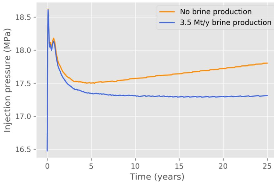
**Figure 3-19 Bottomhole pressure for the onshore model with closed boundary conditions comparing injection with brine production (injection case On-2c-1-1, blue curve) and without brine production (injection case On-2c-1, orange curve) for a CO<sub>2</sub> injection rate of 2 Mt/y**
