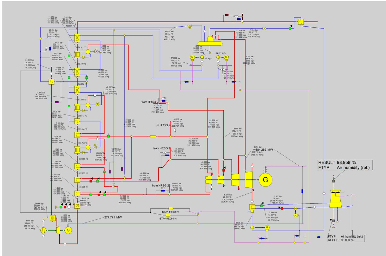
Apx Figure A.22 Flow diagram of the NGCC power plant process using evaporative (EV) cooling
