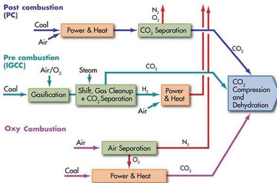
Figure 1-10 CO<sub>2</sub> capture systems: post-combustion, pre-combustion and oxy-combustion capture (Global CCS Institute, 2012)
