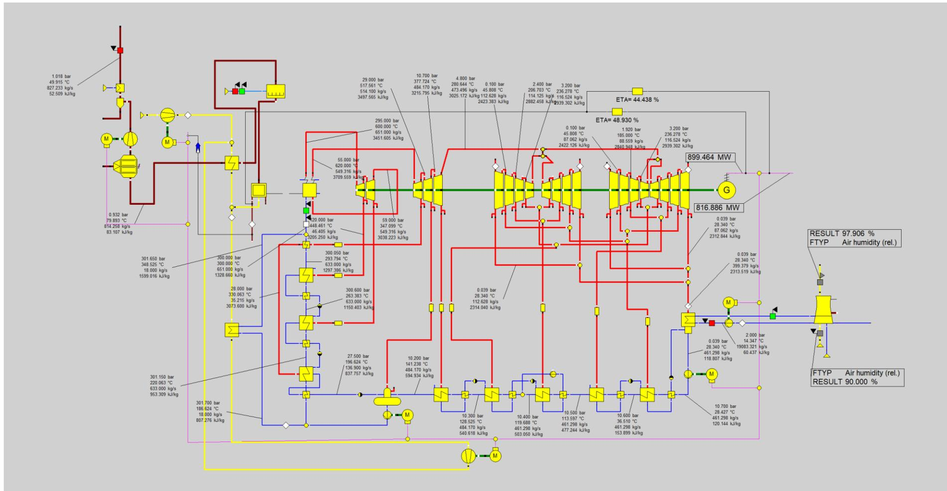
Apx Figure A.2 Flow diagram of the USCPC power plant process using evaporative (EV) cooling
