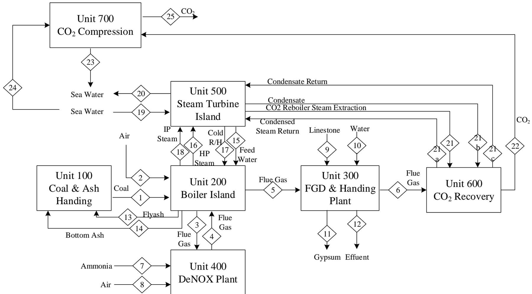
Apx Figure A.7 USCPC power plant with CO<sub>2</sub> capture with once-through (OT) seawater cooling and same or air-cooled (AC) capture plant (Case 1.2B: USCPC-OT-PCC or Case 1.2C: USCPC-OT-PCC-AC)
