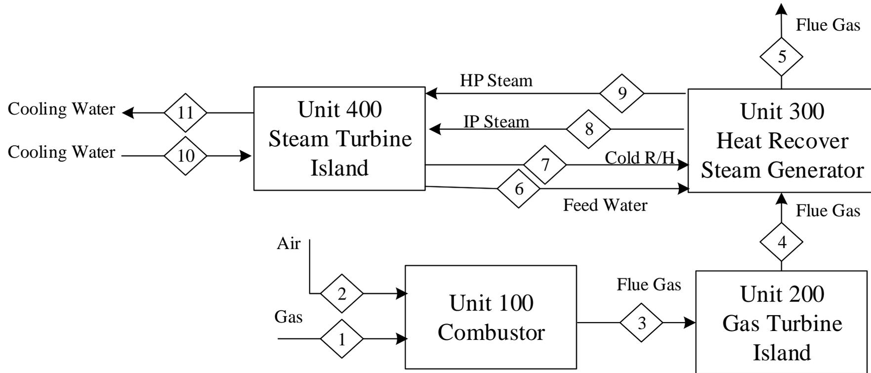
Apx Figure A.21 NGCC power plant using evaporative (EV) cooling (Case 2.1A: NGCC-EV)
