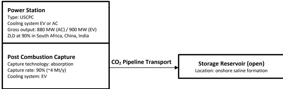
Figure 1 Flow diagram of the Base Case CCS Scenario: CCS in an open formation without water extraction (EV = evaporative cooling, AC = air cooling, ZLD = zero liquid discharge)
