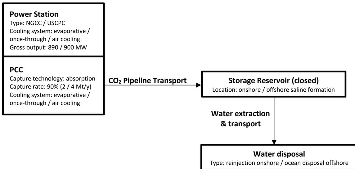
Figure 4-1 Flow diagram of the two cases of the base case scenario: a) CCS in an open formation without water extraction; b) CCS in a closed formation with water extraction and disposal
