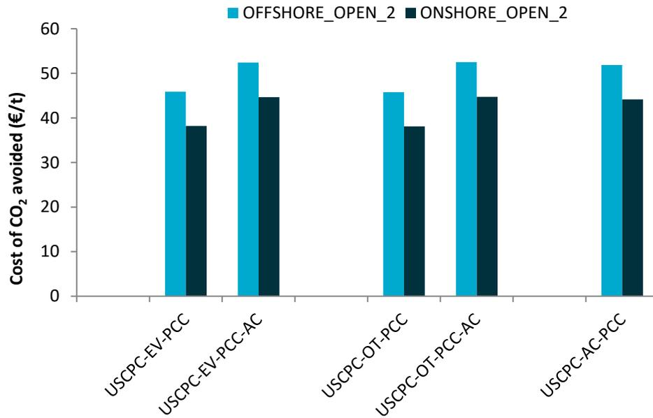
Figure 5-2 Cost of CO<sub>2</sub> avoided for USCPC power plants with CCS in saline formations with open reservoir boundaries onshore and offshore Netherlands
