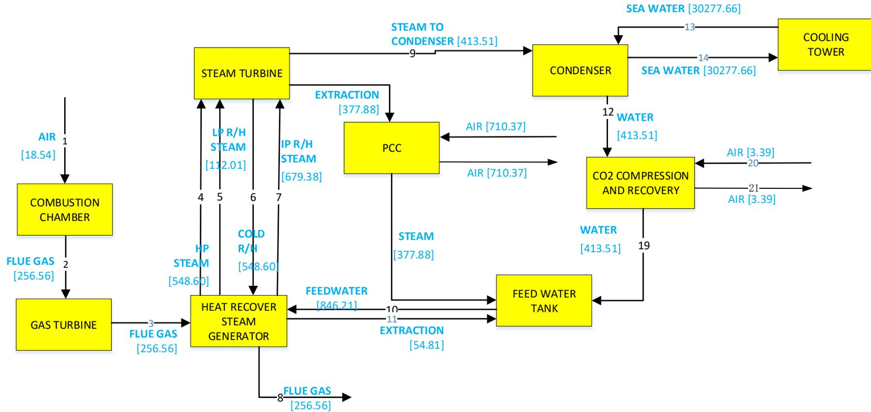
Apx Figure A.38 Water balance in tonnes/hour (t/h) for NGCC power plant using once-through (OT) cooling for the power plant and air cooling (AC) for the capture plant (Case 2.2C: NGCC-OT-PCC-AC)
