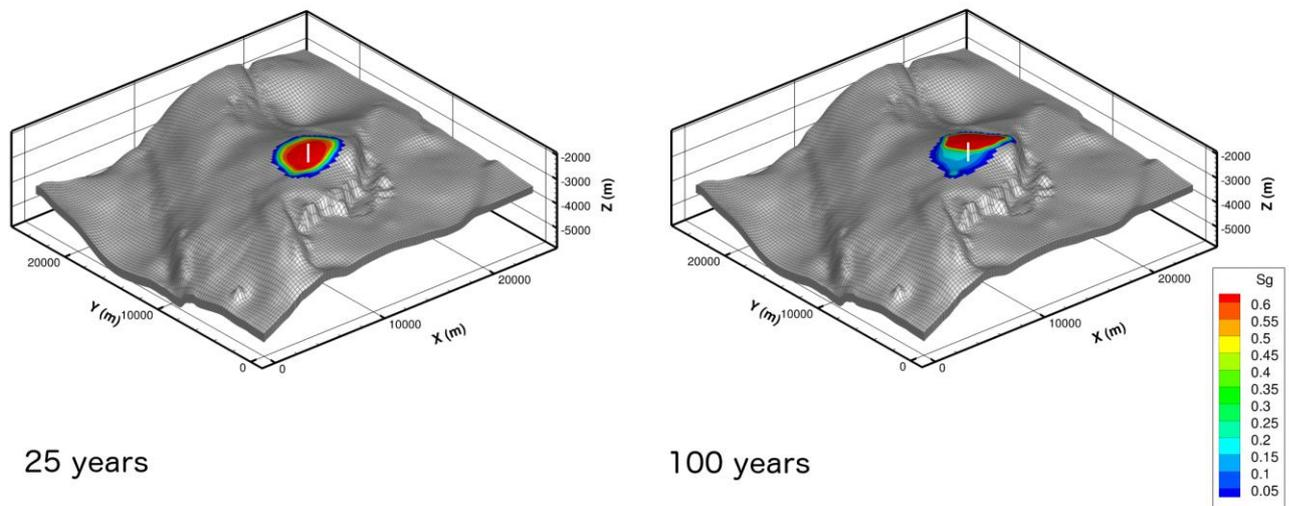
**Figure 3-8 Offshore injection of 2 Mt/y for 25 years (injection case Off-2o-1). Plume extent at 25 years (left) and 100 years (right)**
