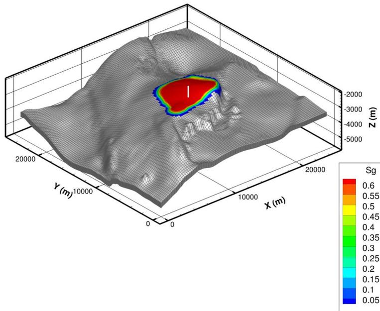
**Figure 3-13 4 Mt/y injection for 50 years in the offshore model with open boundary conditions. The plume is just about to migrate away from the main structure**
