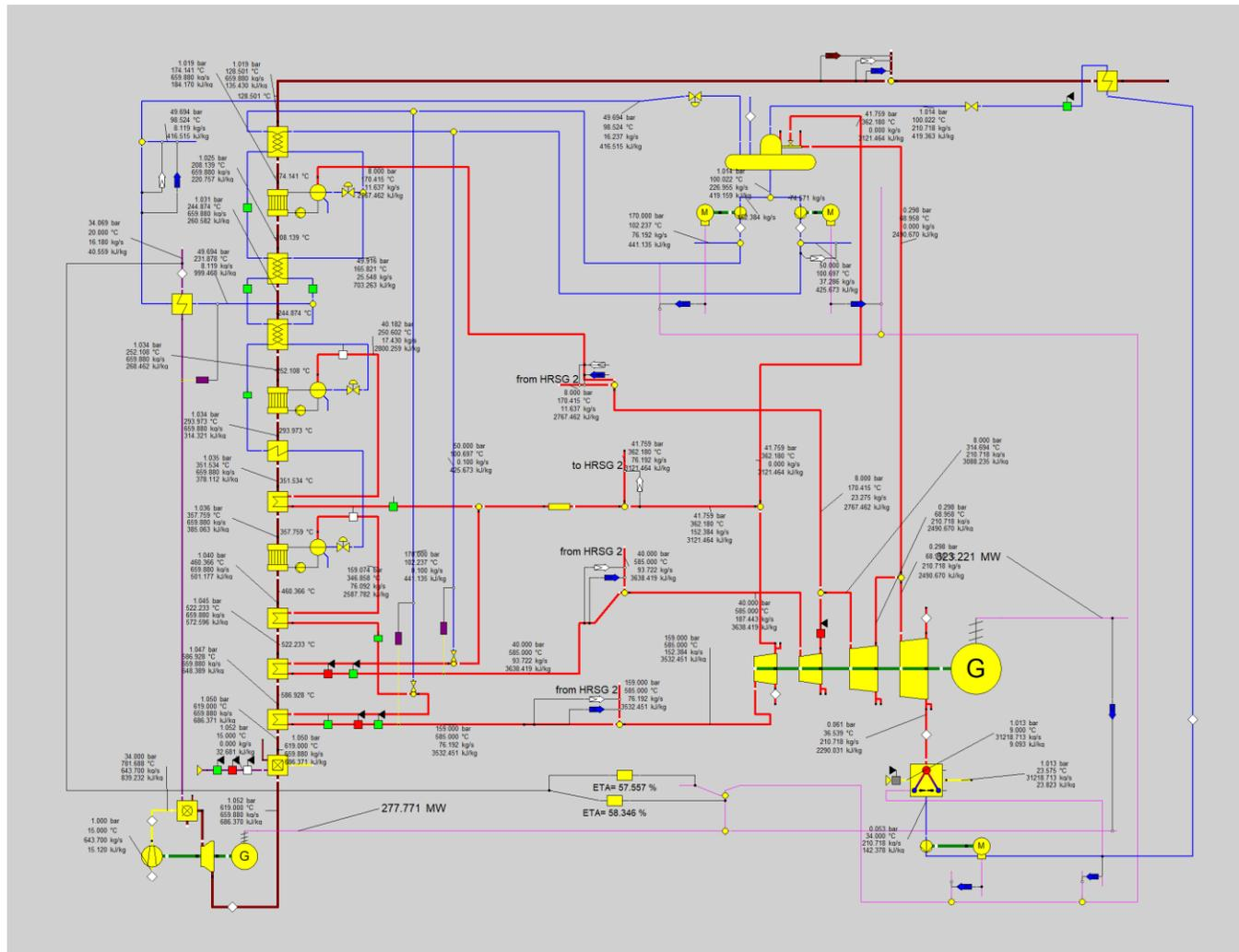
Apx Figure A.30 Flow diagram of the NGCC power plant process using air cooling (AC)
