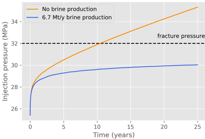
**Figure 9** Bottomhole pressure for the offshore model with closed boundary conditions comparing injection with brine production (injection case Off-4c-2-2, blue curve) and without brine production (injection case Off-4c-2, orange curve) for a CO<sub>2</sub> injection rate of 4 Mt/y
