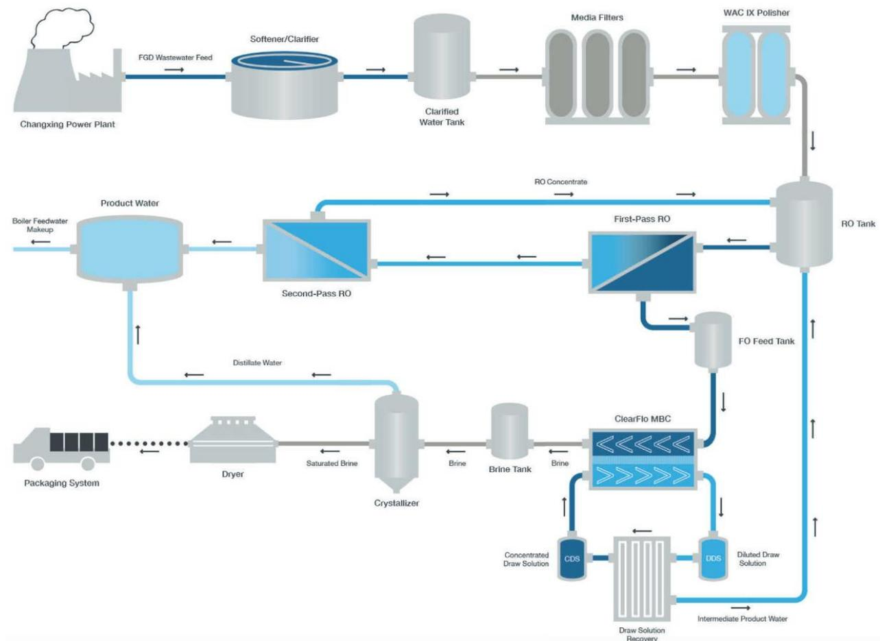
**Figure 1-7 Changxing's ZLD process flow (from Oasys Water, 2016)**
