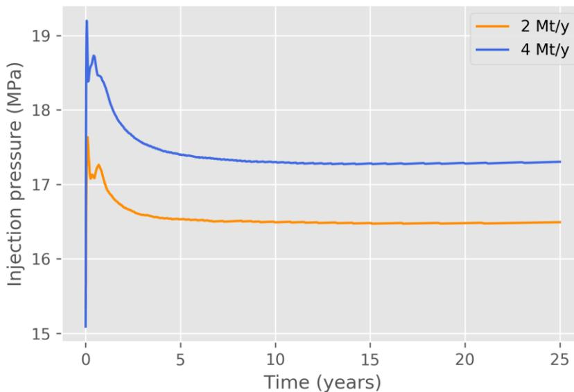
**Figure 3-18 Bottomhole pressure for the onshore model with open aquifer boundary conditions for the 2 Mt/y injection case On-2o-1 (orange curve) and the 4 Mt/y injection case On-4o-1 (blue curve)**
