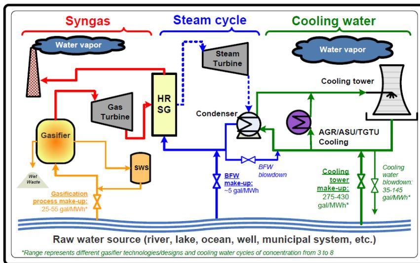
Figure 1-4 Water schematic at an IGCC plant (with wet cooling tower) (DOE-NETL, 2009)
