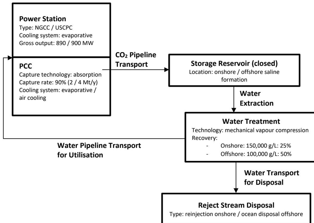
**Figure 4-2** Flow diagram of the CCS-Water-Nexus Scenario with water extraction, treatment, and utilisation in the power station with capture
