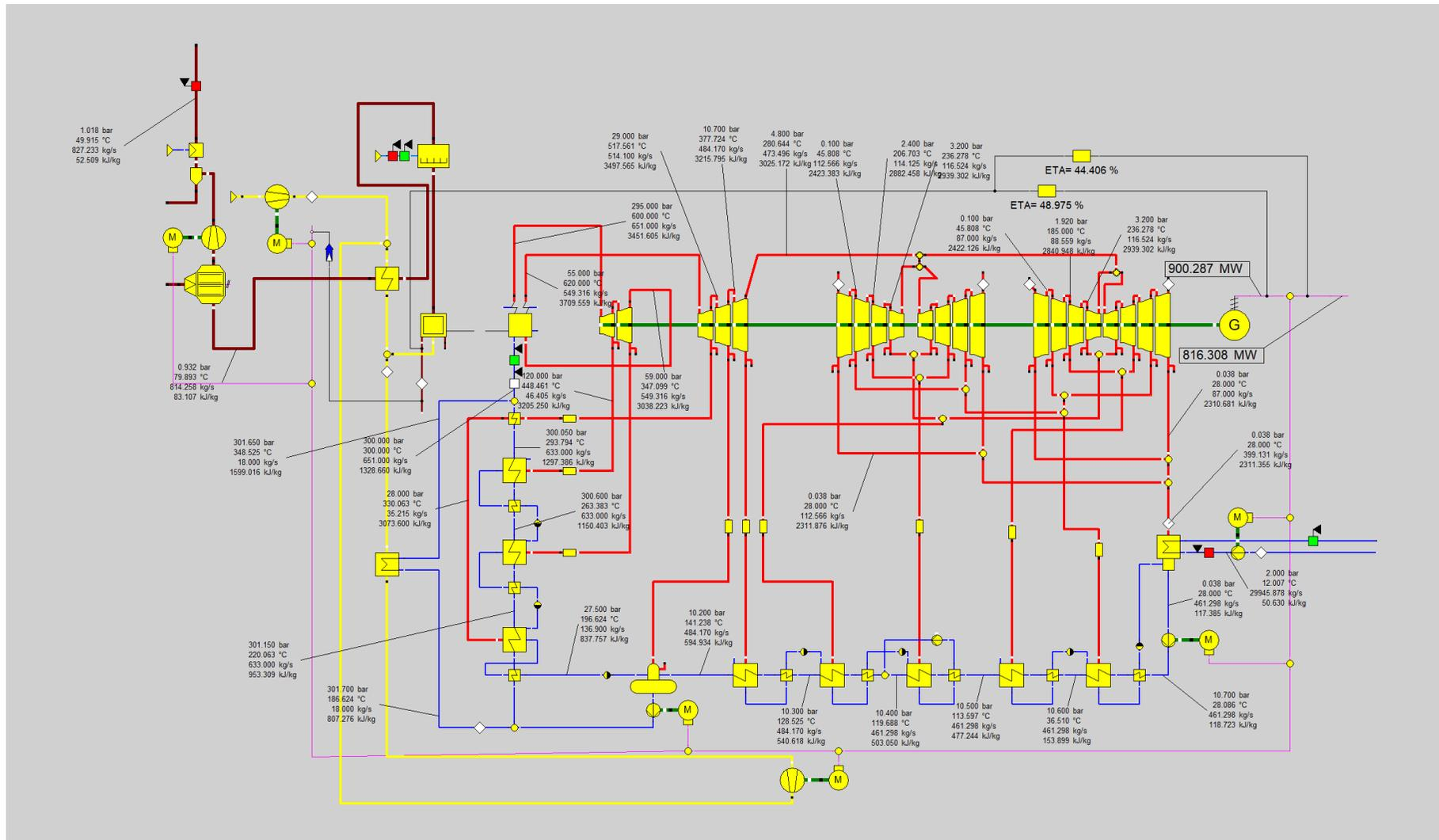
Apx Figure A.6 Flow diagram of the USCPC power plant process using once-through (OT) cooling
