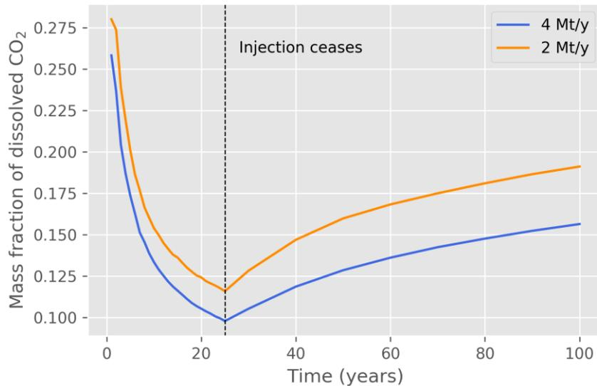
**Figure 3-9 Dissolved CO<sub>2</sub> fraction in the offshore model with open boundary conditions over time for the 2 Mt/y injection case Off-2o-1 (orange curve) and the 4 Mt/y injection case Off-4o-1 (blue curve)**
