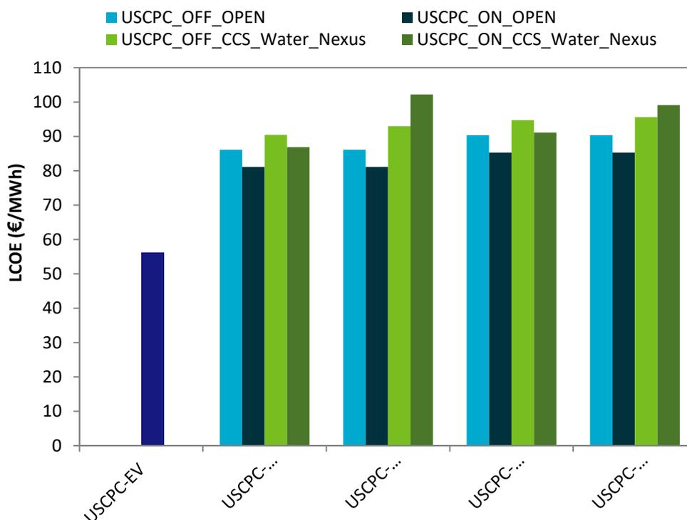
Figure 5-11 Comparison of LCOE of USCPC power plants in the CCS-Water-Nexus Scenario (onshore [ON] and offshore [OFF] with water extraction and utilisation: USCPC\_CCS\_Water\_Nexus) with i.) a power plant without capture (USCPC-EV); and ii.) USCPC with CCS in open saline formations (no water extraction and management: USCPC\_OPEN)
