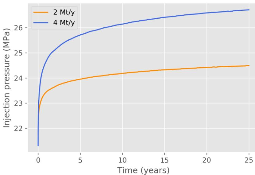
**Figure 3-10 Bottomhole pressure for the offshore model with open aquifer boundary conditions for the 2 Mt/y injection case Off-2o-1 (orange curve) and the 4 Mt/y injection case Off-4o-1 (blue curve)**
