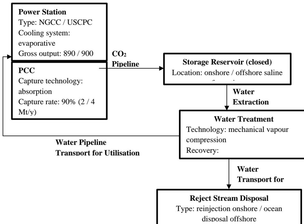
**Figure 2** Energy-Water-CCS nexus scenarios with water extraction, treatment, and utilisation in the power plant with capture
