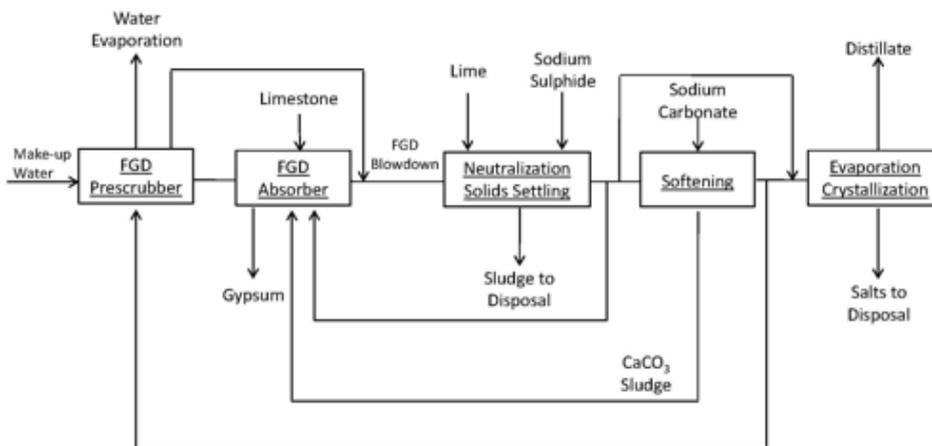
Figure 1-9 Schematic of the ZLD approach at Brindisi, Italy (from Aquatech, 2018a)
