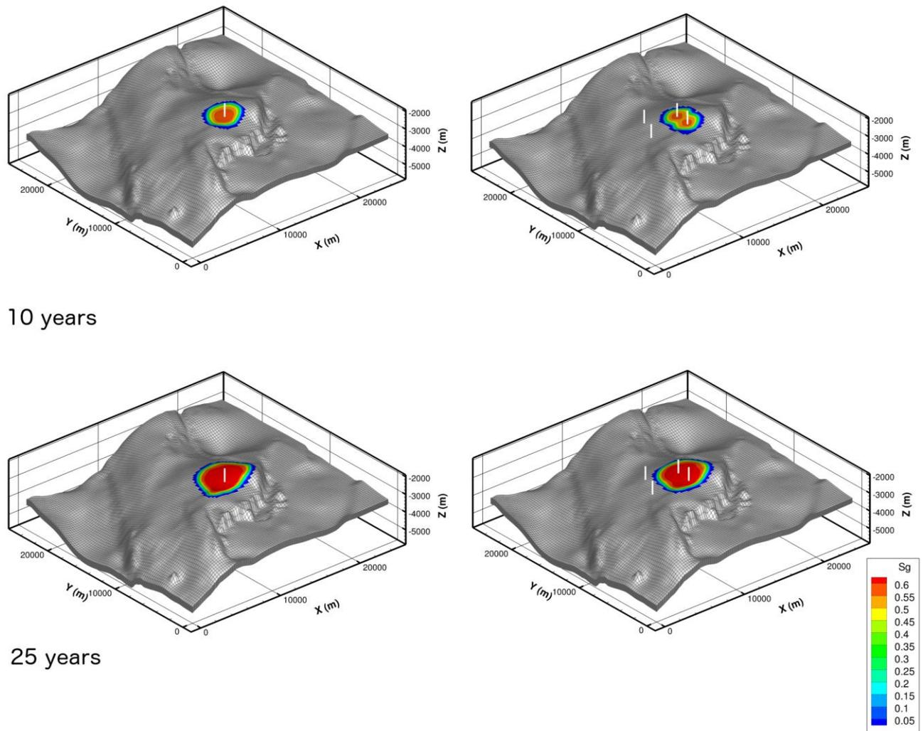
**Figure 3-7 Comparison of a single injection well and no production well (injection case Off-4c-1, left), and two injection wells and two production wells (injection case Off-4c-2-2-A, right) after 10 years (top) and 25 years (bottom)**
