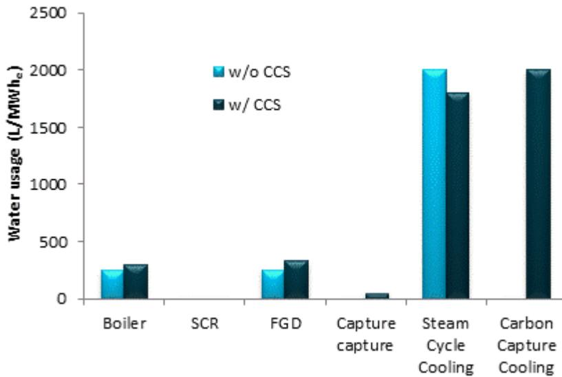
Figure 1-14 Water use distribution points for power plants with and without carbon capture (adapted from Zhai and Rubin, 2016). SCR and FGD denote selective catalytic reduction and flue gas desulphurisation respectively
