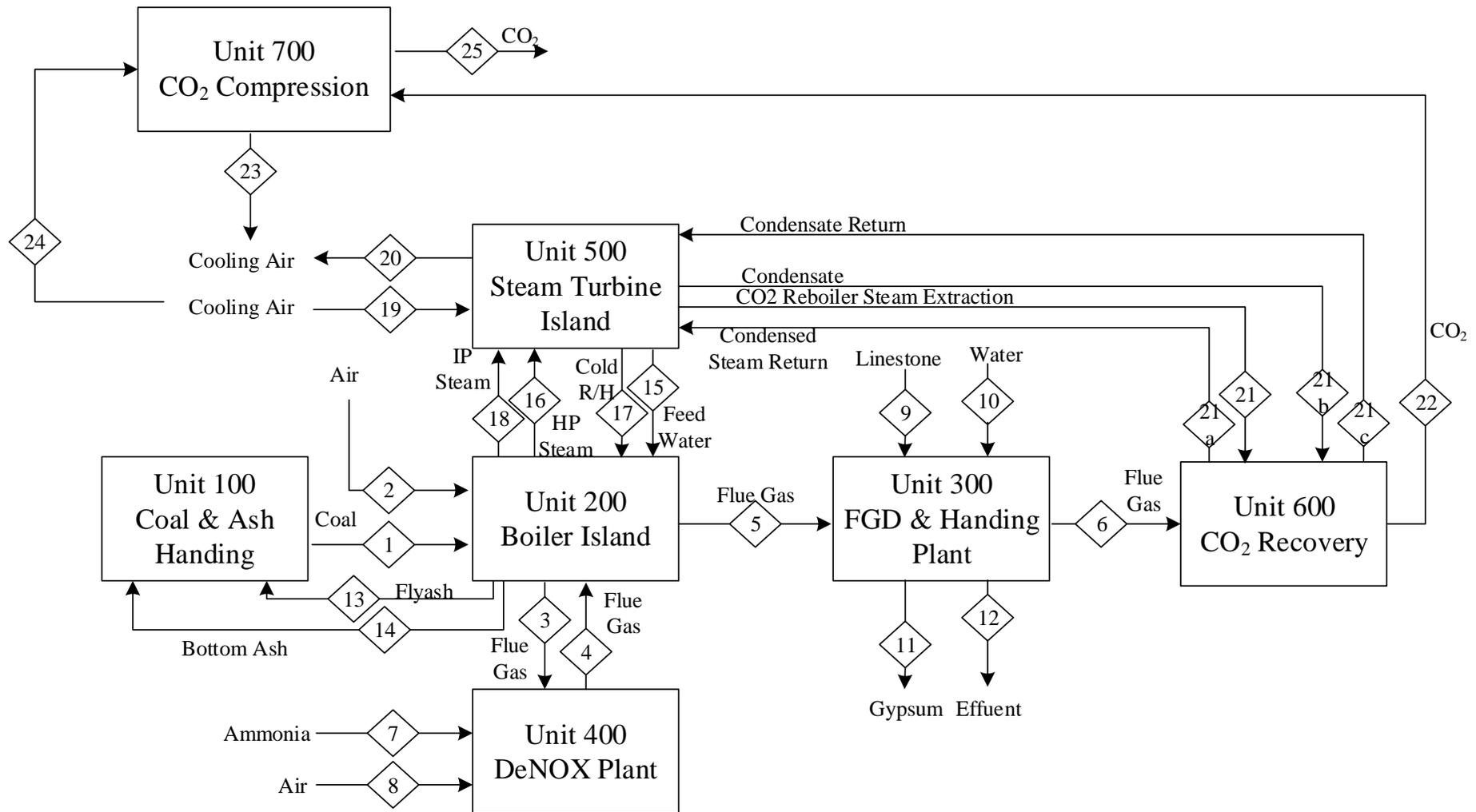
Apx Figure A.11 USCPC power plant with CO<sub>2</sub> capture with air cooling (Case 1.3A: USCPC-AC-PCC)
