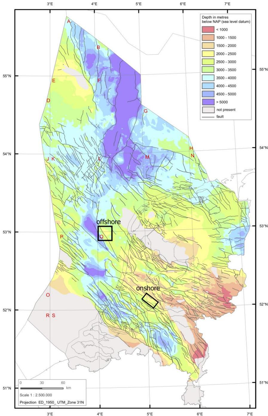
**Figure 3-1** Location of offshore and onshore models (location indicated by the black rectangles). Depths are the base of the Zechstein group, which corresponds to the top surface of the reservoir models ([www.nlog.nl](http://www.nlog.nl))
