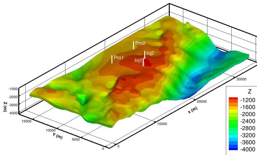
Figure 3-3 Computational reservoir model of the onshore aquifer. Contours indicate depth in metres
