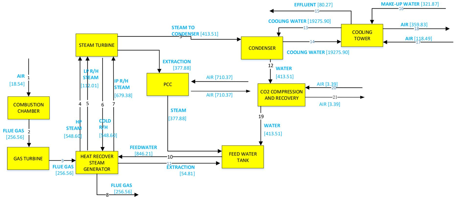
Apx Figure A.35 Water balance in tonnes/hour (t/h) for NGCC power plant with capture using evaporative (EV) cooling for the power plant and air cooling (AC) for the capture plant (Case 2.1C: NGCC-EV-PCC-AC)
