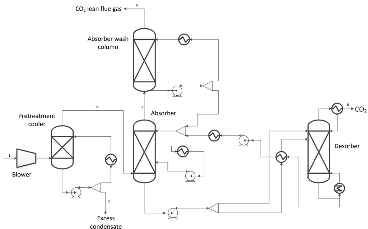
**Figure 2-10 Line diagram of CO<sub>2</sub> capture plant used in amine-based post-combustion capture simulations. The layout includes absorber intercooling and rich-split process modifications**
