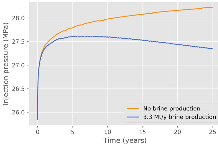
**Figure 3-11 Bottomhole pressure for the offshore model with closed boundary conditions comparing injection with brine production (injection case Off-2c-1-1, blue curve) and without brine production (injection case Off-2c-1, orange curve) for an injection rate of 2 Mt/y.**
