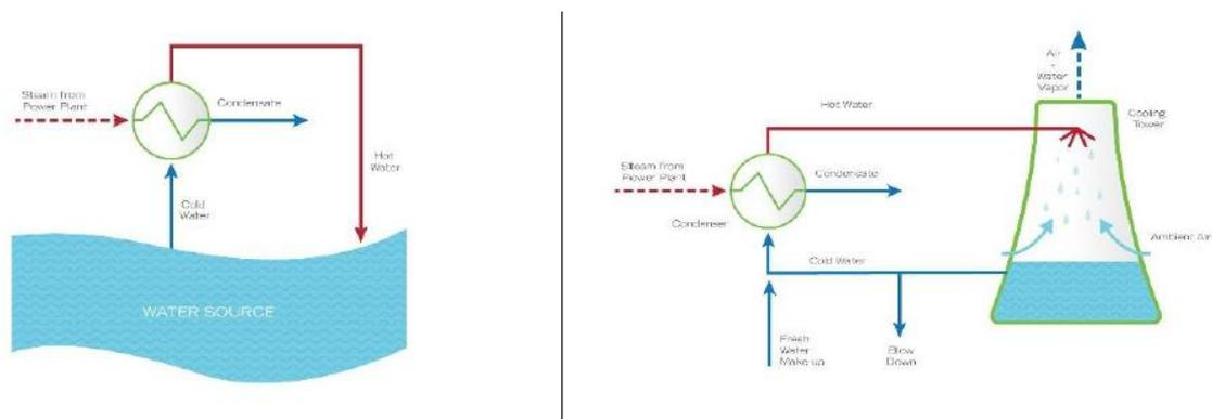
Figure 1-1 Once-through (left) and recirculating cooling systems (right) (Global CCS Institute, 2016)
