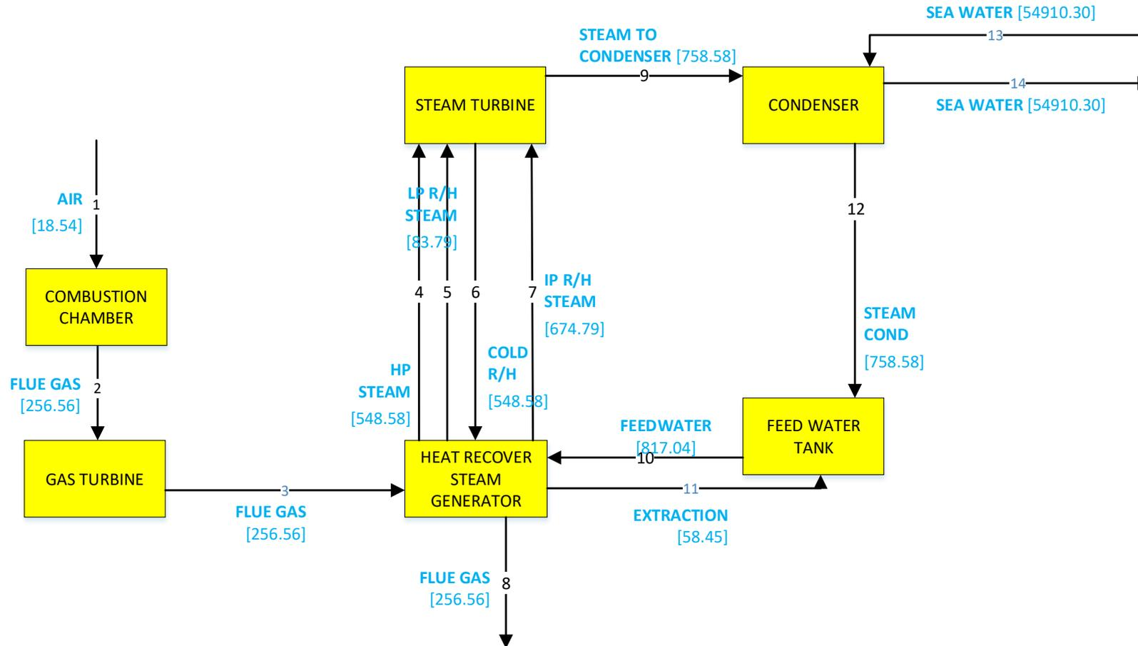
Apx Figure A.36 Water balance in tonnes/hour (t/h) for NGCC power plant without capture using once-through (OT) cooling (Case 2.2A: NGCC-OT)
