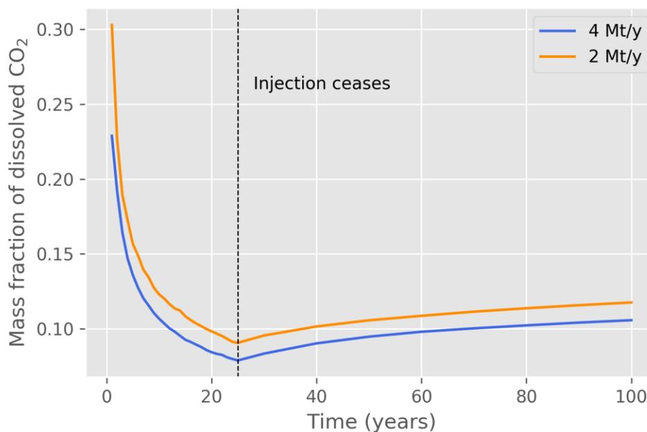
**Figure 3-17: Dissolved CO<sub>2</sub> fraction in the onshore model over time for the 2 Mt/y injection case (On-2o-1, orange curve) and the 4 Mt/y injection case (On-4o-1, blue curve)**
