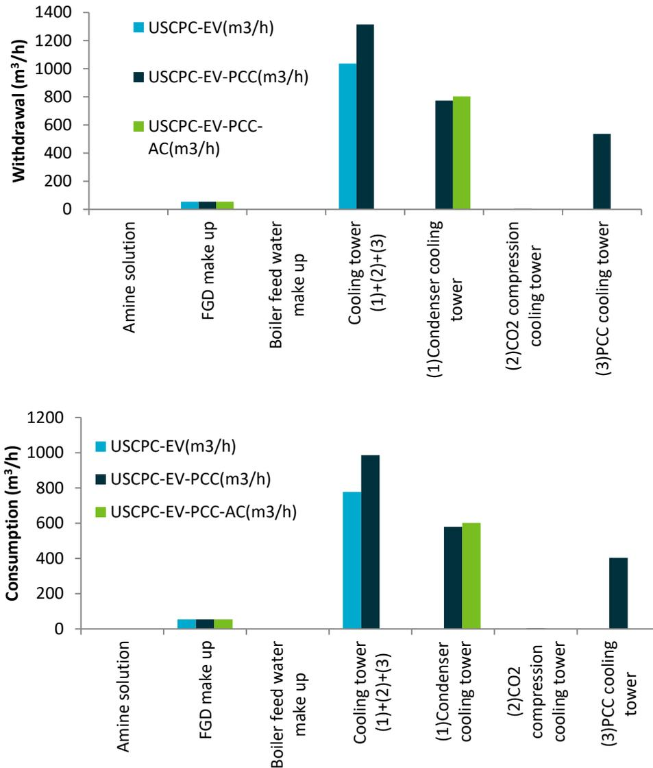
**Figure 3 Absolute water withdrawal and consumption rates for the USCPC using evaporative cooling systems (Cases 1.1A/B/C)**
