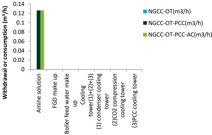
Figure 8 Absolute water withdrawal and consumption rates for the NGCC using once-through seawater cooling systems (Cases 2.3A/B/C)
