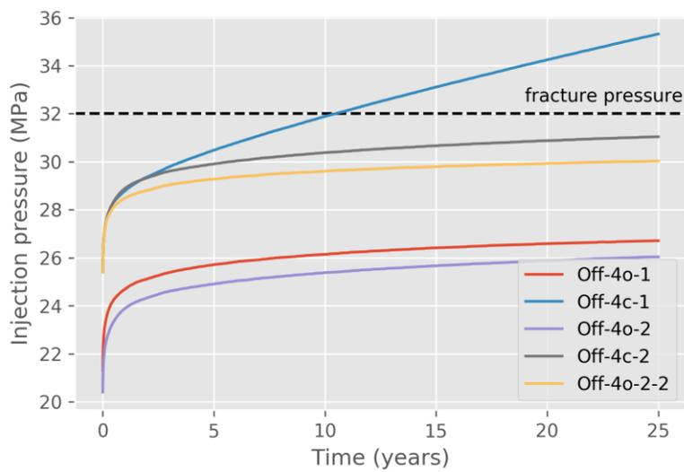
Apx Figure B.42 Bottomhole pressure for all 4 Mt/y injection scenarios for the offshore model
