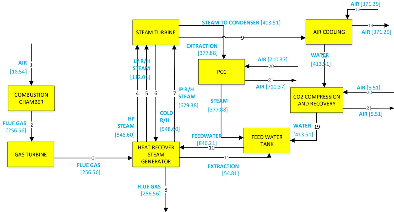
Apx Figure A.40 Water balance in tonnes/hour (t/h) for NGCC power plant with capture using air cooling (AC) (Case 2.3B: NGCC-AC-PCC)
