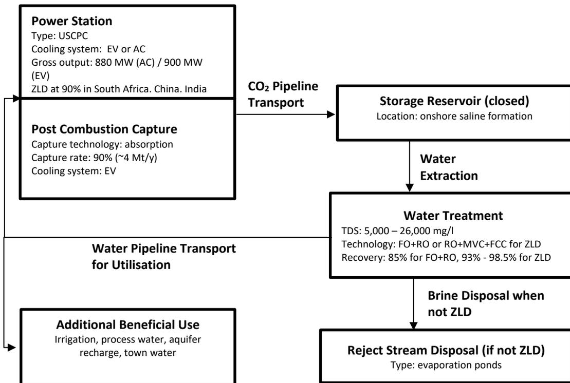
Figure 2 Flow diagram of the CCS-Water-Nexus Scenario with water treatment and utilisation in the power station with capture and other beneficial use (FO = forward osmosis, RO = reverse osmosis, MVC = mechanical vapour compression, FCC = forced circulation crystallizer, ZLD = zero liquid discharge)
