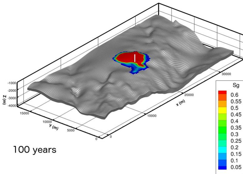
Figure 3-14 Onshore CO<sub>2</sub> injection of 4 Mt/y for 25 years (injection case On-4o-1). The plume extent at 10 years (top), 25 years (middle), and 100 years (bottom)
