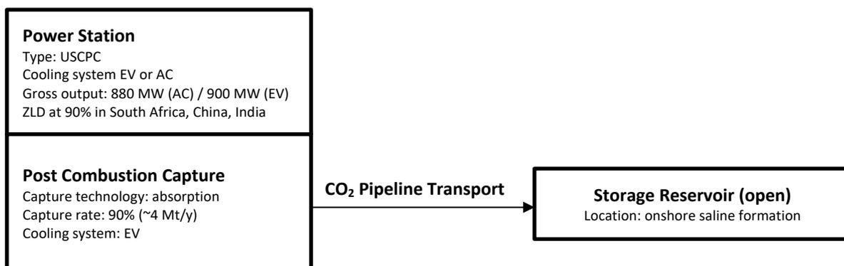
Figure 4-1 Flow diagram of the base case scenario: CCS in an open formation without water extraction. AC = air cooling, EV = evaporative cooling
