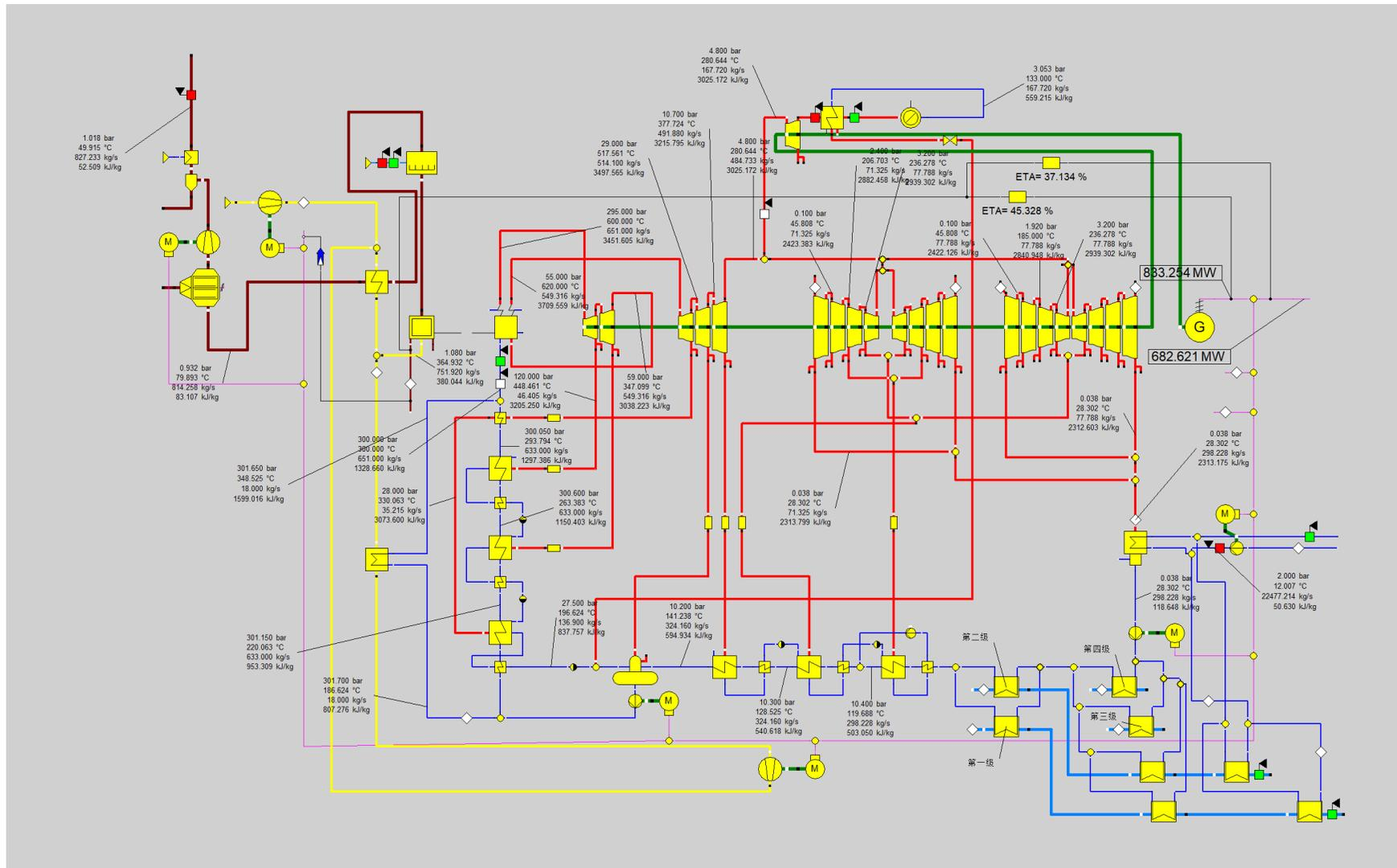
Apx Figure A.8 Flow diagram of the USCPC power plant with capture process using once-through (OT) cooling
