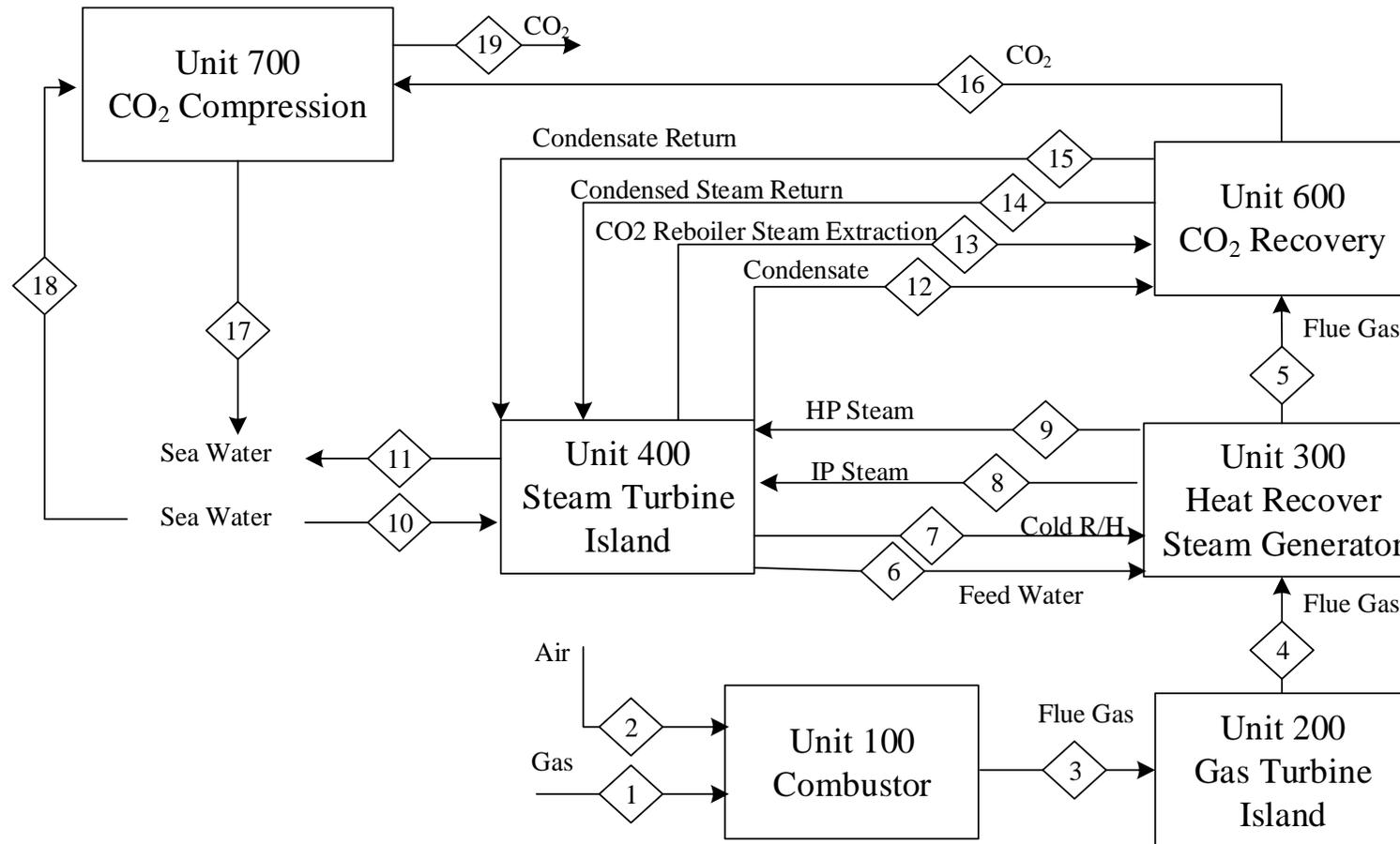
Apx Figure A.27 NGCC power plant with capture using once-through (OT) seawater cooling using same or air cooling for capture plant (Case 2.2B: NGCC-OT-PCC or Case 2.2C: NGCC-OT-PCC-AC)
