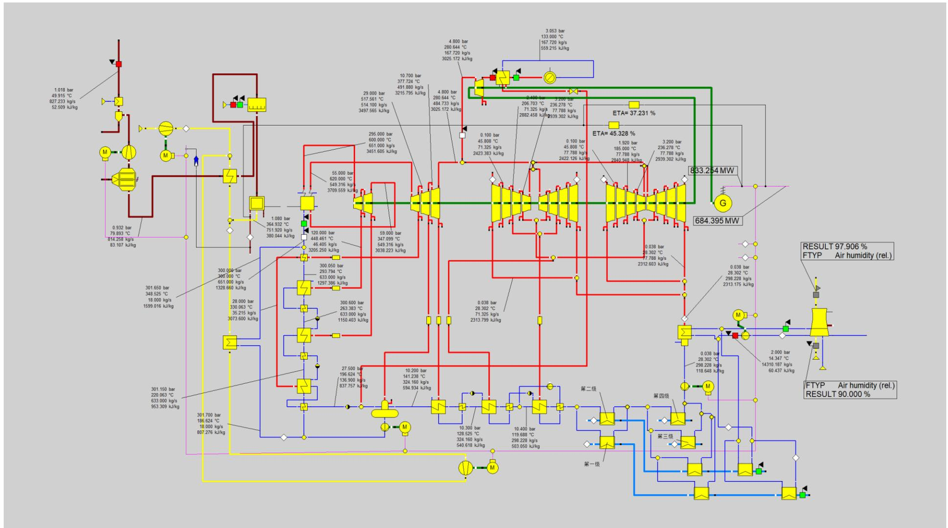
Apx Figure A.4 Flow diagram of the USCPC power plant process with capture using evaporative (EV) cooling
