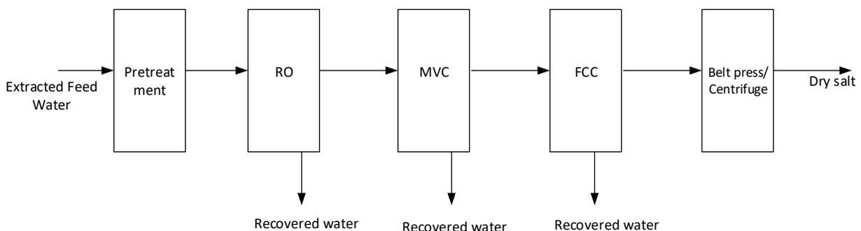
Figure 3-2 Process schematic for the ZLD treatment of extracted water from South Africa, China, and India
