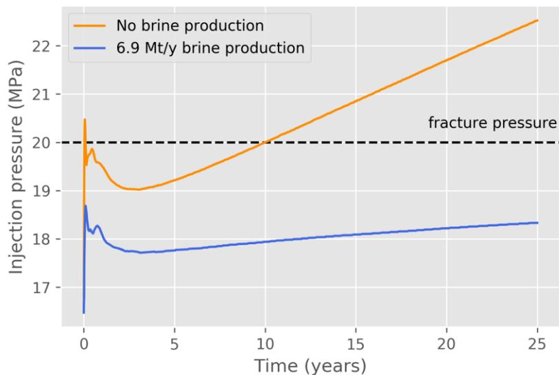
**Figure 3-20 Bottomhole pressure for the onshore model with closed boundary conditions comparing injection with brine production (injection case On-4c-2, orange curve) and without brine production (injection case On-4c-2-2, blue curve) for an injection rate of 4 Mt/y**
