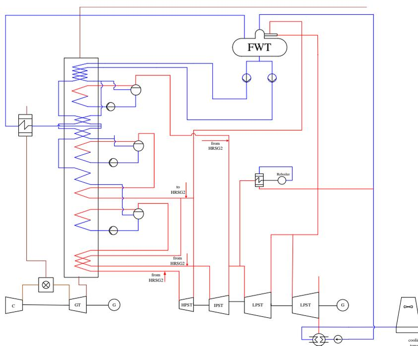
**Figure 2-9 Process flow diagram for a natural gas fired combined cycle power plant with integrated post-combustion capture**
