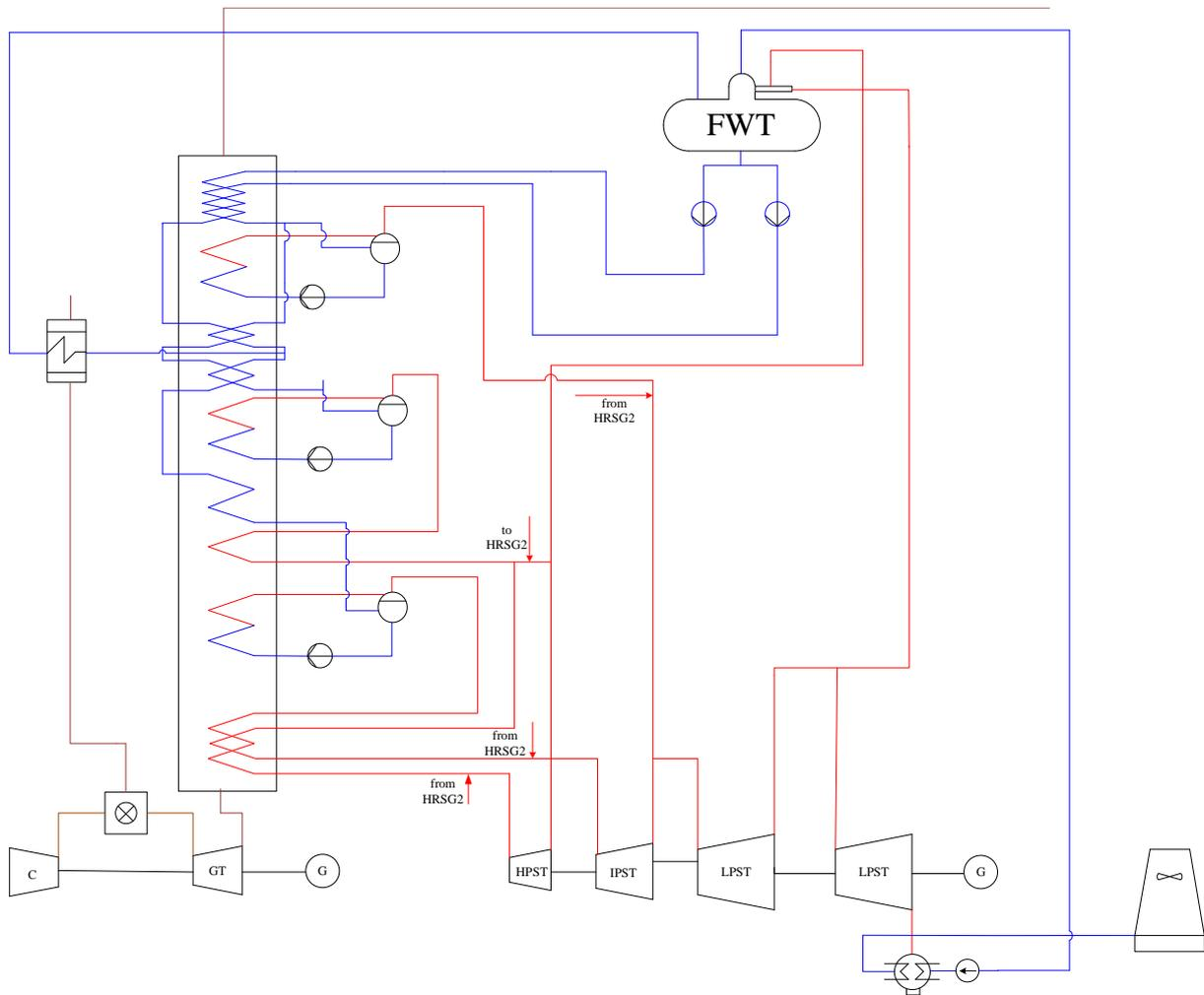
**Figure 2-8** Process diagram for natural gas fired combined cycle power plant
