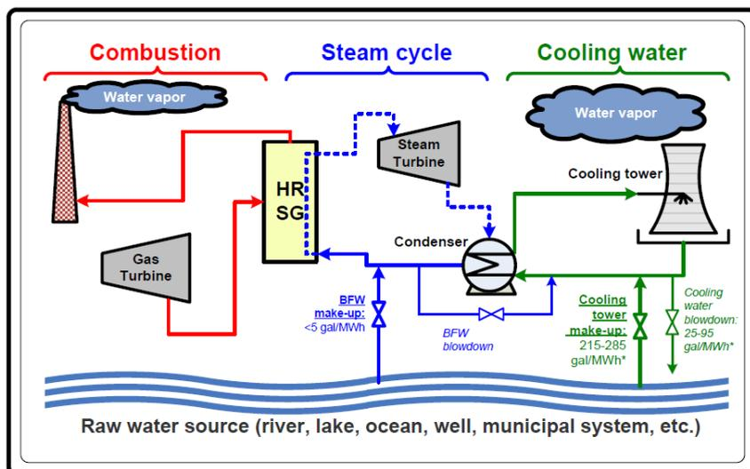
Figure 1-3 Water schematic at a NGCC plant (with wet cooling tower) (DOE-NETL, 2009)
