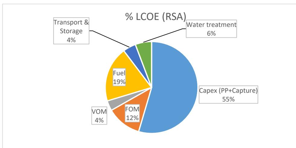
**Figure 7** Percentage breakdown of capital and operational costs for a USCPC power plant in the Republic of South Africa (RSA) with capture plant and incorporated water treatment facility. (PP= Power Plant, VOM = variable operational and maintenance, FOM = fixed operational and maintenance cost)
