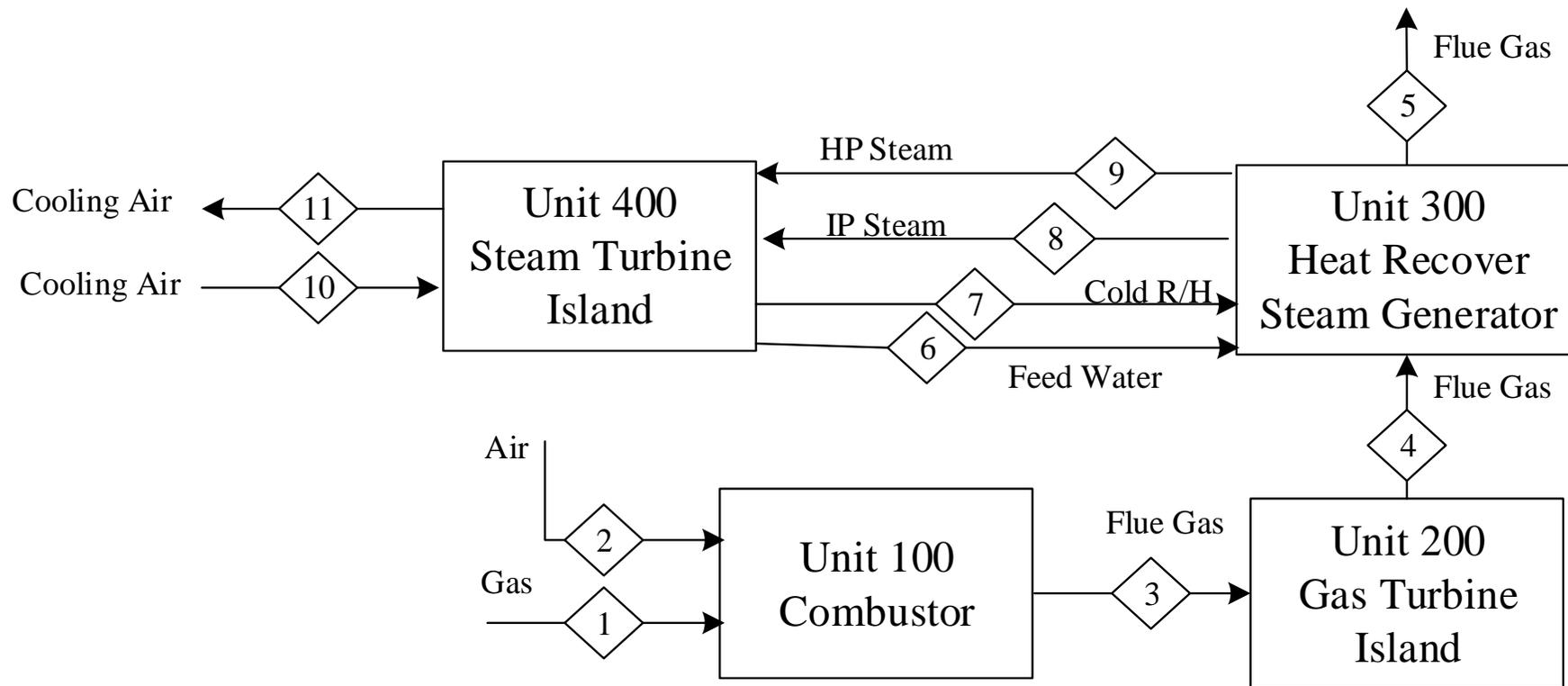
Apx Figure A.29 NGCC power plant using air cooling (AC) (Case 2.3A: NGCC-AC)
