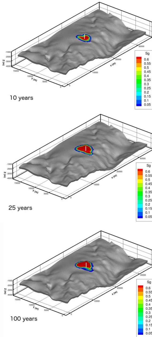
Figure 3-16 Onshore CO<sub>2</sub> injection of 2 Mt/y for 25 years (injection case On-2o-1). The plume extent at 10 years (top), 25 years (middle), and 100 years (bottom)
