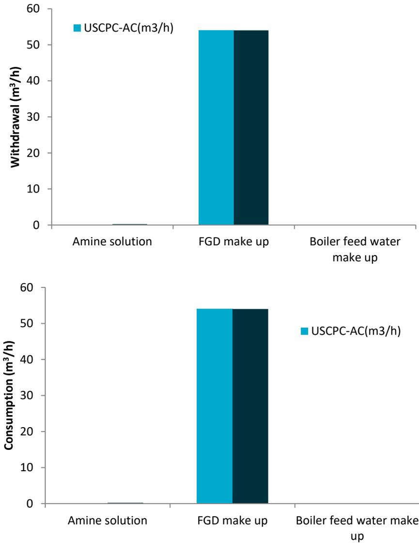
**Figure 2-6 Absolute water withdrawal and consumption rates for the USCPC using air cooling systems comparing Case 1.3A (USCPC-AC) and Case 1.3B (USCPC-AC-PCC)**
