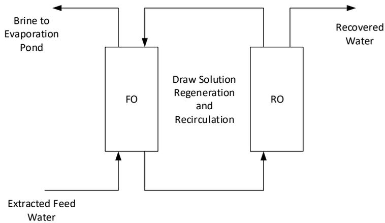
Figure 3-1 Schematic of combined FO-RO treatment for extracted water from Australia
