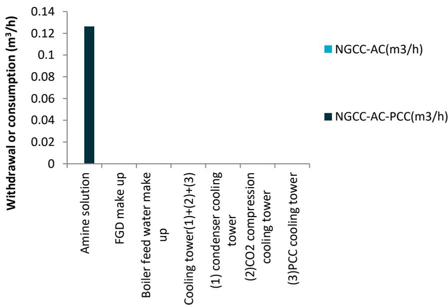
**Figure 2-13 Absolute water withdrawal and consumption rates for the NGCC using air cooling systems comparing Case 2.3A (NGCC-AC) and Case 2.3B (NGCC-AC-PCC)**
