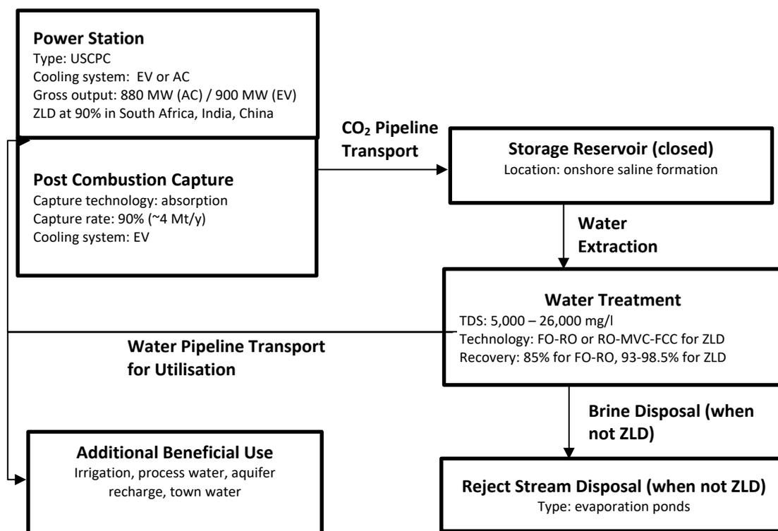
Figure 4-2 Flow diagram of the CCS-Water-Nexus Scenario with water extraction, treatment, and utilisation in the power station with capture and additional beneficial use options. AC = air cooling, EV = evaporative cooling, FCC = forced circulation crystalliser, FO-RO = forward osmosis – reverse osmosis, MVC = mechanical vapour compression, TDS = total dissolved solids, ZLD = zero liquid discharge
