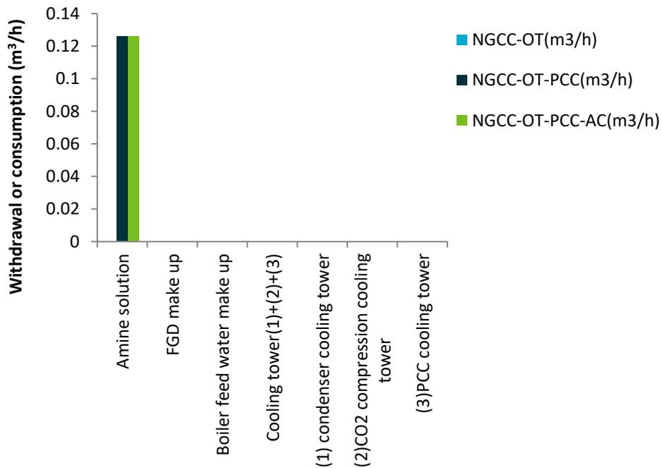
Figure 2-14 Absolute water withdrawal and consumption rates for the NGCC using once-through seawater cooling systems comparing Case 2.2A (NGCC-OT), Case 2.2B (NGCC-OT-PCC), and Case 2.2C (NGCC-OT-PCC-AC)
