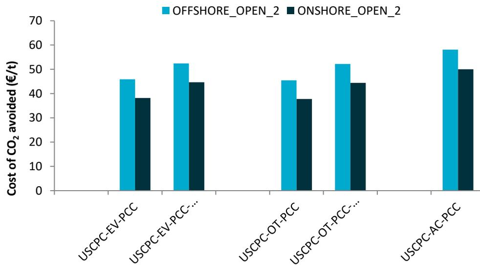
Figure 5-3 Cost of CO<sub>2</sub> avoided for USCPC power plants with CCS in saline formations with open reservoir boundaries onshore and offshore Netherlands, where the reference plant is the USCPC-EV (Case 1.1A)
