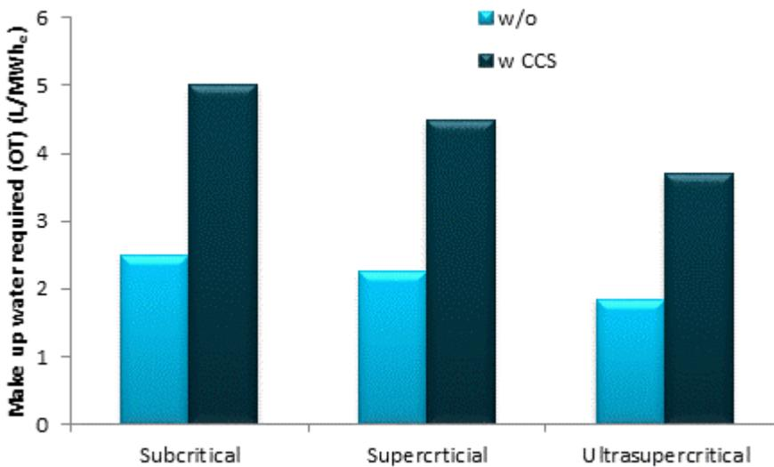
Figure 1-15 Water usage for different coal-fired power plant types with and without capture (adapted from Zhai and Rubin, 2016)
