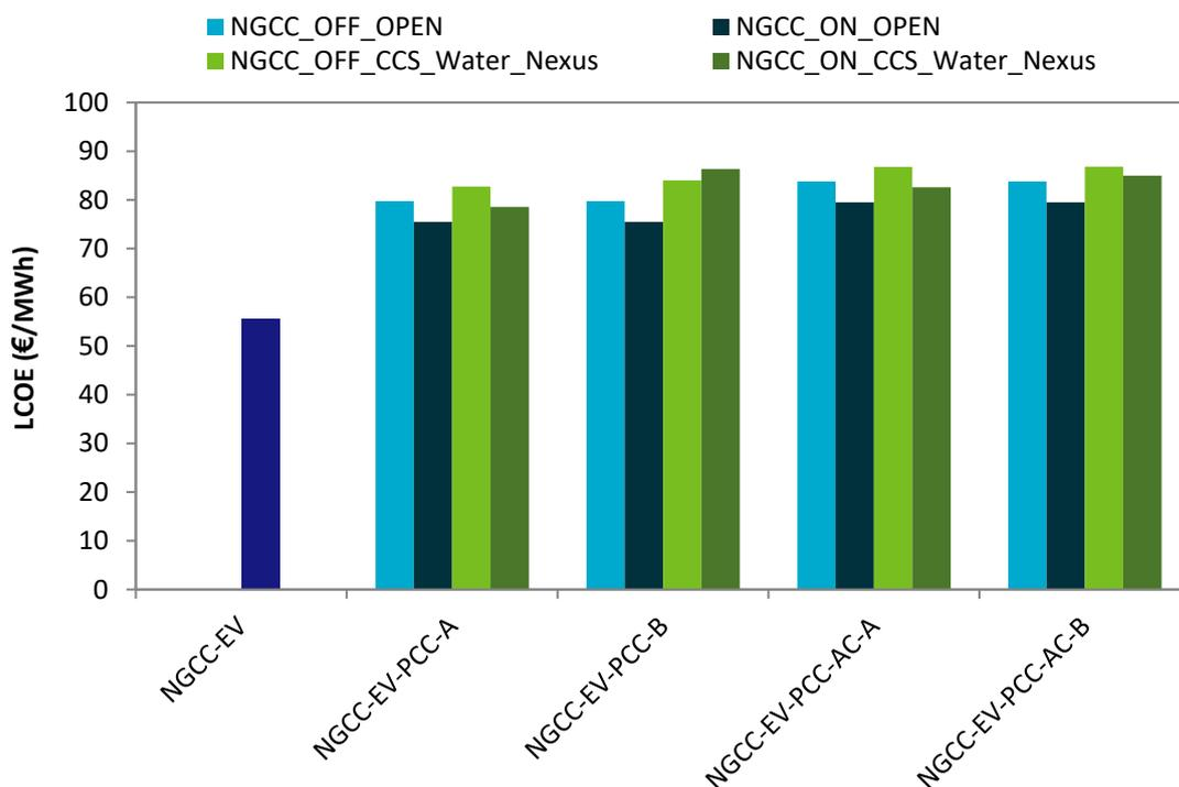
**Figure 5-13 Comparison of LCOE of NGCC power plants in the CCS-Water-Nexus Scenario (onshore [ON] and offshore [OFF] with water extraction and utilisation: NGCC\_CCS\_Water\_Nexus) with i.) a power plant without capture (NGCC-EV); and ii.) NGCC with CCS in open saline formations (no water extraction and management: NGCC\_OPEN)**
