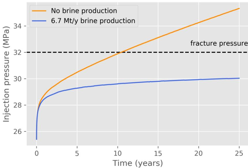
**Figure 3-12 Bottomhole pressure for the offshore model with closed boundary conditions comparing injection with brine production (injection case Off-4c-2-2, blue curve) and without brine production (injection case Off-4c-2, orange curve) for a CO<sub>2</sub> injection rate of 4 Mt/y**
