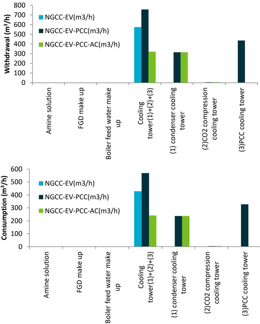
Figure 6 Absolute water withdrawal and consumption rates for the NGCC using evaporative cooling systems (Cases 2.1A/B/C)
