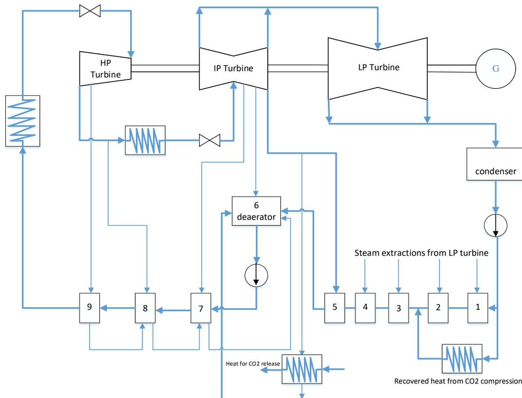
**Figure 2-2 Steam flow diagram for an ultra-supercritical pulverised coal fired power plant with integrated post-combustion capture process**
