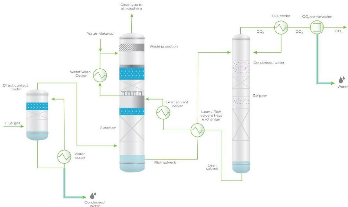
**Figure 1-11 Process flow diagram of a post-combustion capture system using chemical absorption indicating the main process coolers and water inflow/outflow streams (Global CCS Institute, 2016)**
