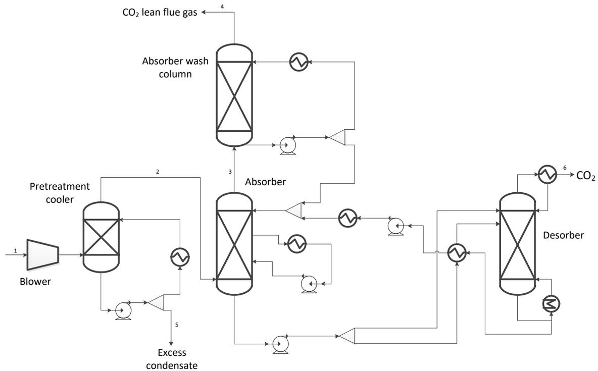
**Figure 2-3 Line diagram of CO<sub>2</sub> capture plant used in amine-based post-combustion capture simulations. The layout includes absorber intercooling and rich-split process modifications**
