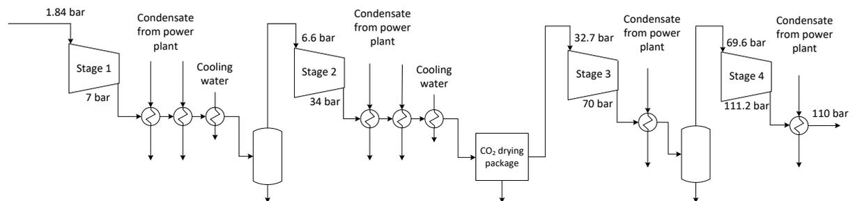
**Figure 2-11 Four-stage CO<sub>2</sub> compression flow diagram for natural gas fired combined cycle power plant**
