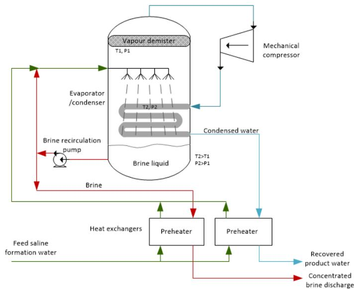
**Figure 3-24 Schematic of mechanical vapour compression process for desalination of saline formation water**
