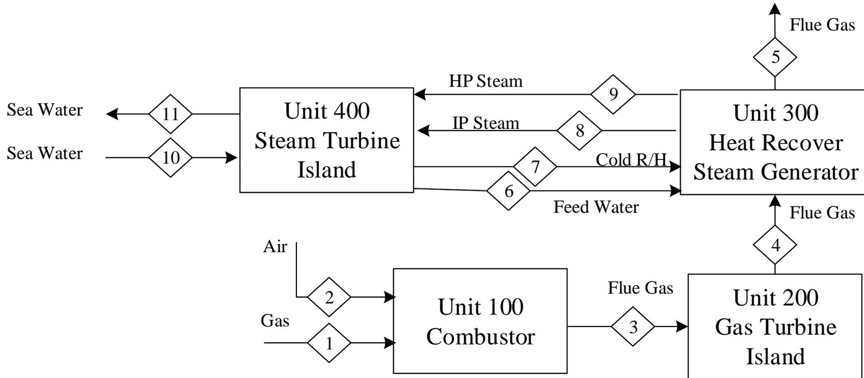
Apx Figure A.25 NGCC power plant without capture using once-through (OT) seawater cooling (Case 2.2A: NGCC-OT)
