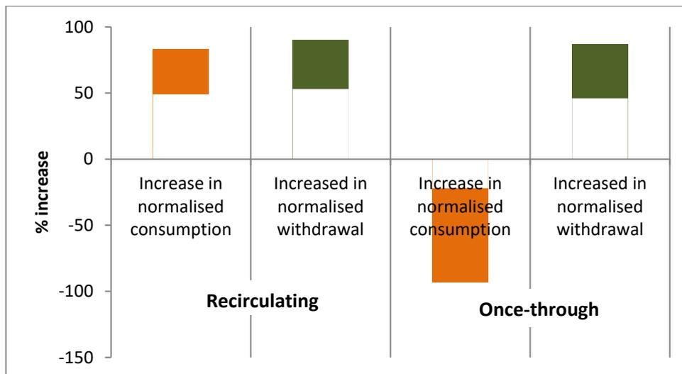
Figure 1-16 Range in increases in normalised consumption and withdrawal for recirculating and once-through cooling: coal fired power plant with post-combustion capture
