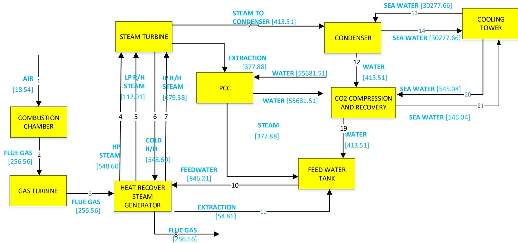
Apx Figure A.37 Water balance in tonnes/hour (t/h) for NGCC power plant with capture using once-through (OT) cooling (Case 2.2B: NGCC-OT-PCC)
