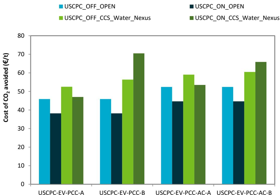
Figure 5-12 Comparison of CO<sub>2</sub> avoidance cost of USCPC power plants in the CCS-Water-Nexus Scenario (onshore [ON] and offshore [OFF] storage with water extraction and utilisation: USCPC\_CCS\_Water\_Nexus) with USCPC with CCS in open saline formations (no water extraction and management: USCPC\_OPEN)
