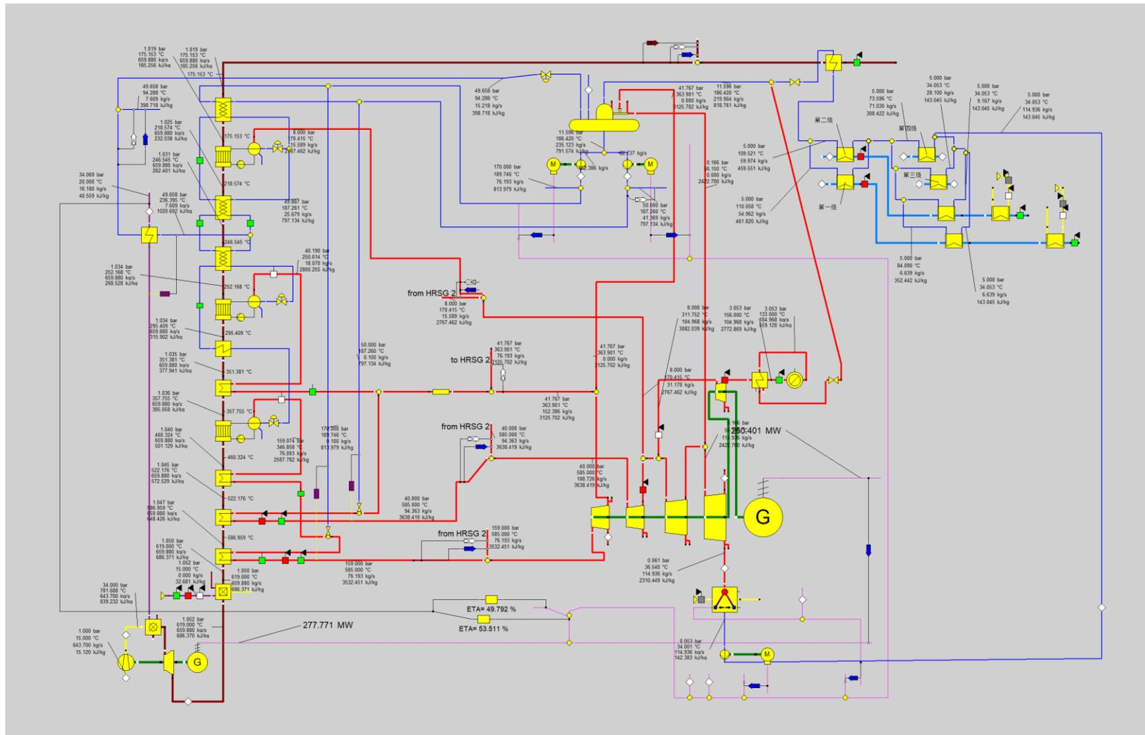
Apx Figure A.32 Flow diagram of the NGCC power plant process with capture using air cooling (AC)
