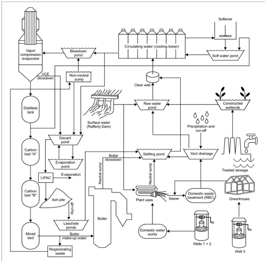
Figure 1-8 A schematic of the water balance at the Shand Power Station (from Quagraine, 2018)
