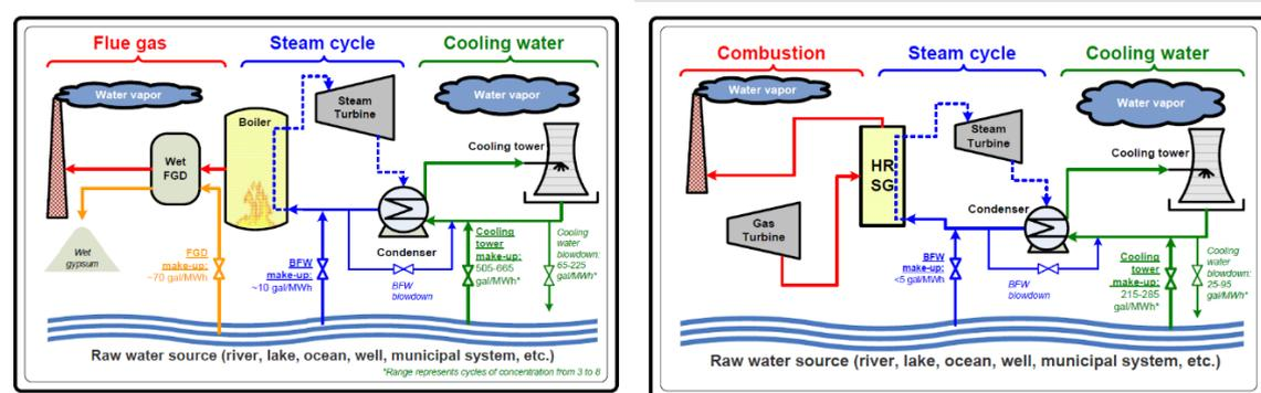
**Figure 1** Water schematic at coal fired (left) and NGCC (right) plants (DOE-NETL, 2009)
