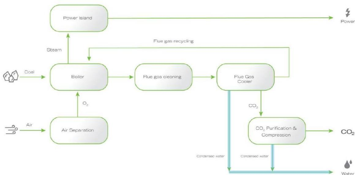
**Figure 1-13 Simplified process flow diagram of an oxy-combustion system indicating main water inflow/outflow streams (Global CCS Institute, 2016)**
