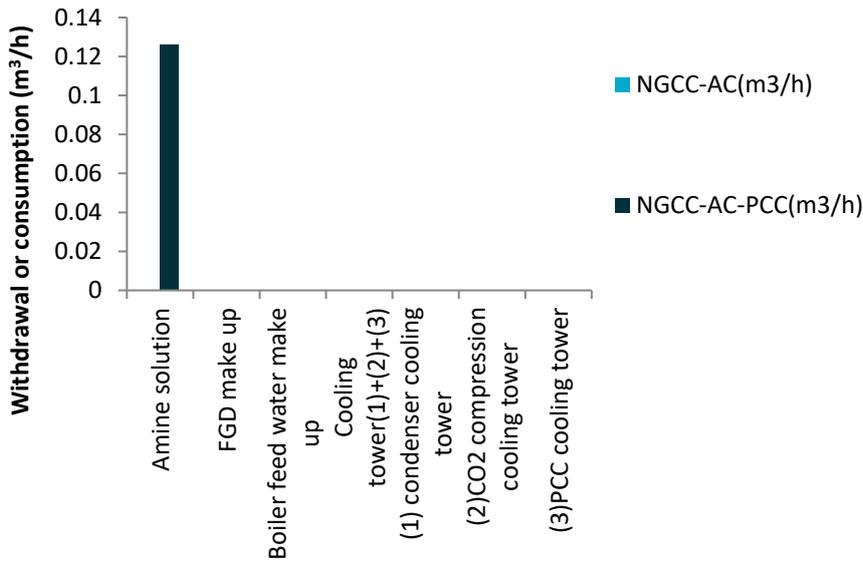
Figure 7 Absolute water withdrawal and consumption rates for the NGCC using air cooling systems (Cases 2.2A/B)
