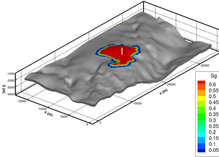
Figure 3-21 Injection of 4 Mt/y CO<sub>2</sub> for 40 years in the onshore model with open boundary conditions. The plume has begun to migrate away from the main structure
