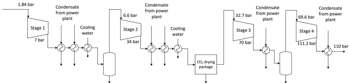
Figure 2-4 Four-stage CO<sub>2</sub> compression flow diagram
