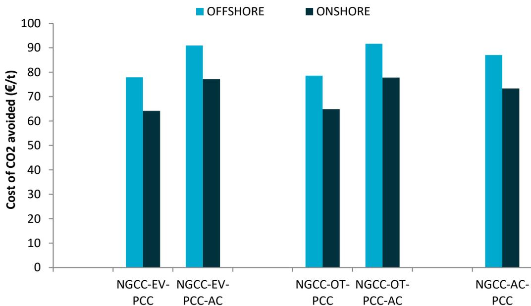
Figure 5-6 Cost of CO<sub>2</sub> avoided for NGCC power plants with CCS in saline formations with open reservoir boundaries onshore and offshore Netherlands where reference plant is the NGCC-EV (Case 2.1A)
