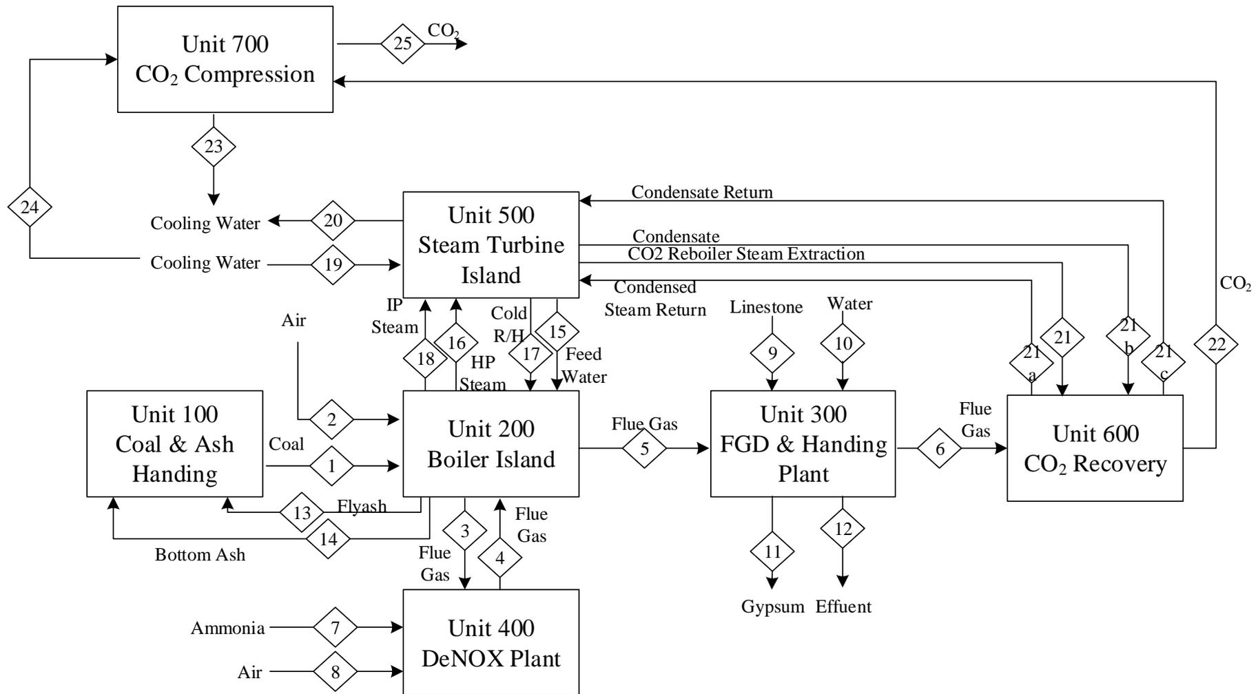
Apx Figure A.3 USCPC power plant with CO<sub>2</sub> capture with evaporative (EV) cooling and same or air-cooled (AC) capture plant (Case 1.1B: USCPC-EV-PCC or Case 1.1C: USCPC-EV-PCC-AC)
