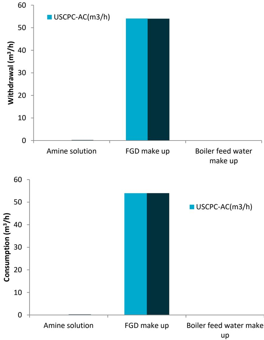
**Figure 4 Absolute water withdrawal and consumption rates for the USCPC using air cooling systems (Cases 1.3A/B)**
