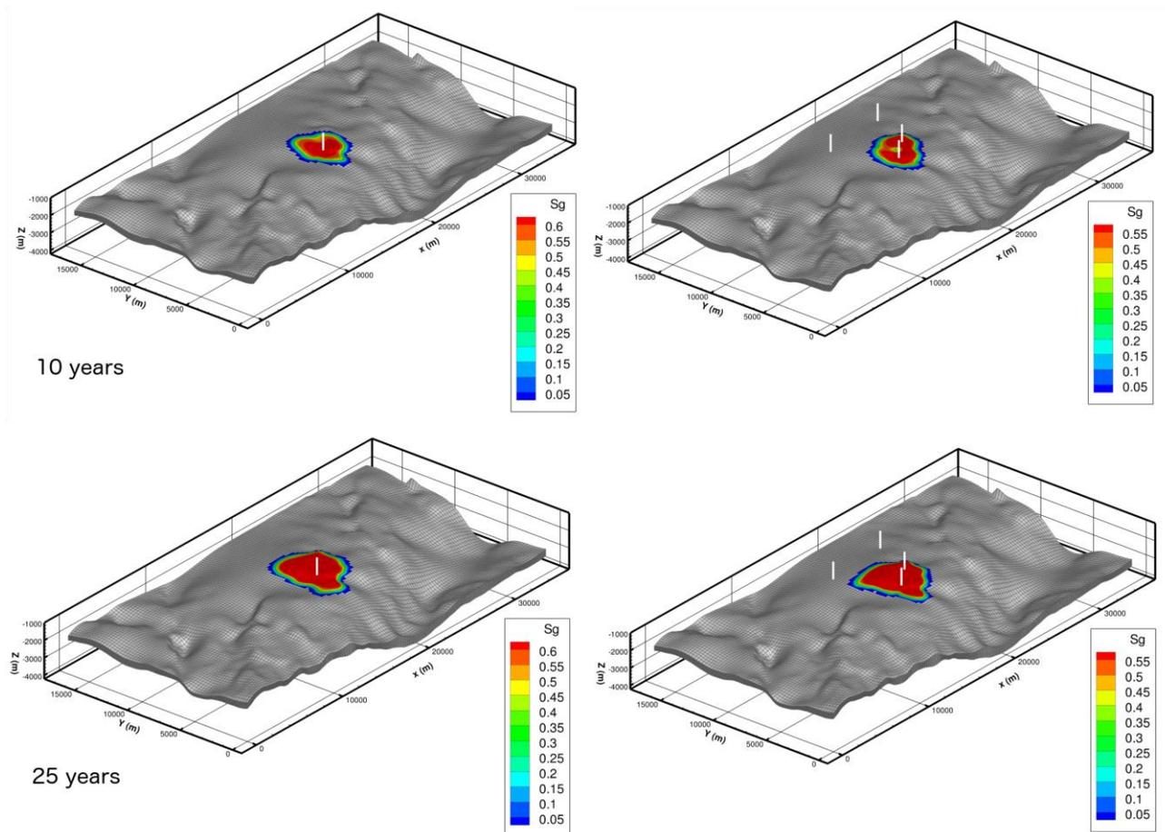
**Figure 3-15 Comparison of a single injection well and no production well (injection case On-4c-1, left), and two injection wells and two production wells (injection case On-4c-2-2-A, right) onshore after 10 years (top) and 25 years (bottom)**
