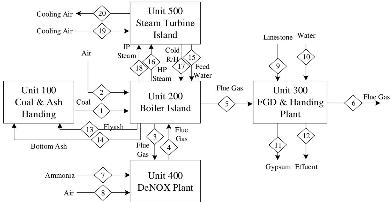
Apx Figure A.1 USPC power plant with evaporative (EV) cooling (Case 1.1A: USPC-EV)
