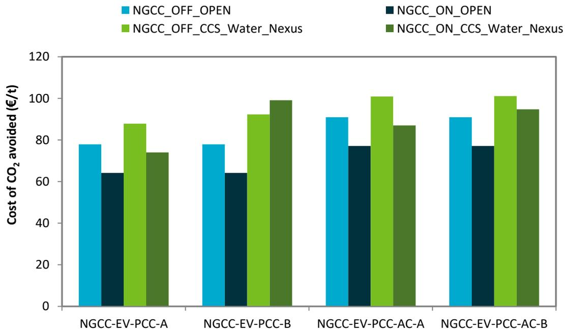
Figure 5-14 Comparison of cost of avoidance of NGCC power plants in the CCS-Water-Nexus Scenario (onshore [ON] and offshore [OFF] with water extraction and utilisation: NGCC\_CCS\_Water\_Nexus) with NGCC with CCS in open saline formations (no water extraction and management: NGCC\_OPEN)
