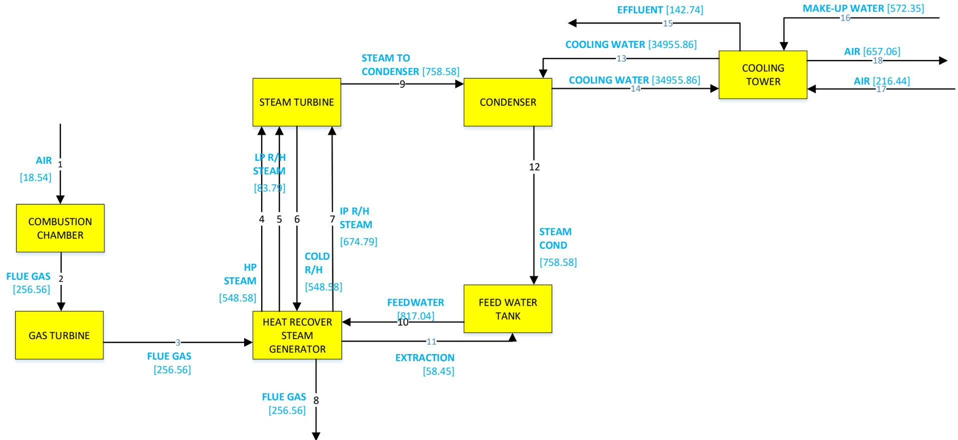
Apx Figure A.33 Water balance in tonnes/hour (t/h) for NGCC power plant without capture using evaporative (EV) cooling (Case 2.1A: NGCC-EV)
