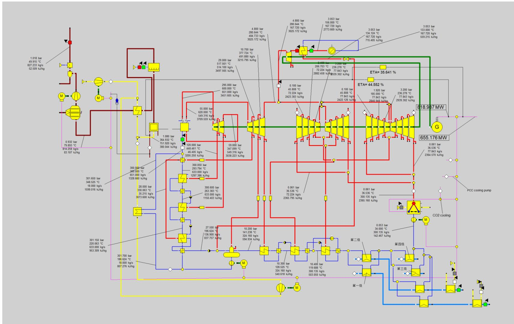
Apx Figure A.12 Flow diagram of the USCPC power plant with capture process using air cooling (AC)
