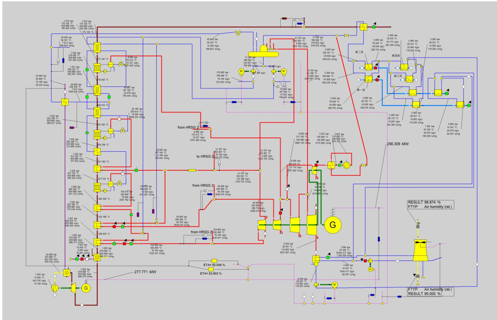
Apx Figure A.24 Flow diagram of the NGCC power plant process with capture using evaporative (EV) cooling
