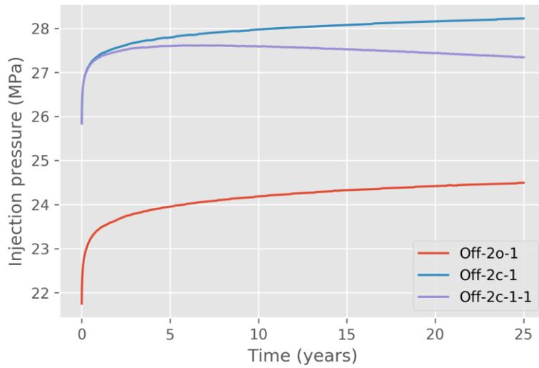
Apx Figure B.41 Bottomhole pressure for all 2 Mt/y injection scenarios for the offshore model
