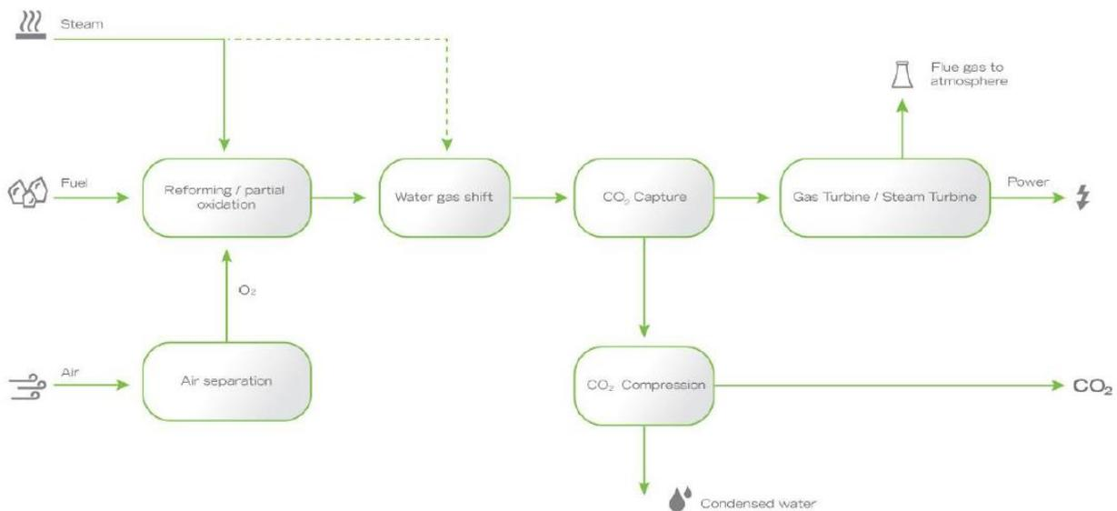
**Figure 1-12 Simplified process flow diagram of a pre-combustion capture system using absorption indicating the main process coolers and water inflow/outflow streams (Global CCS Institute, 2016)**
