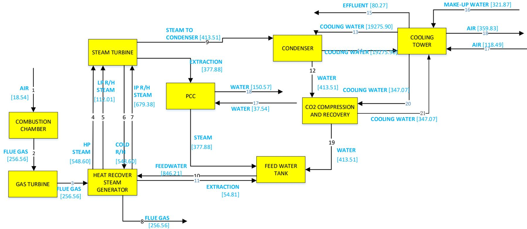
Apx Figure A.34 Water balance in tonnes/hour (t/h) for NGCC power plant with capture using evaporative (EV) cooling (Case 2.1B: NGCC-EV-PCC)
