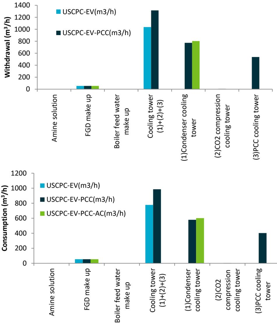
Figure 2-5 Absolute water withdrawal and consumption rates for the USCPC using evaporative cooling systems comparing Case 1.1A (USCPC-EV), Case 1.1B (USCPC-EV-PCC), and Case 1.1C (USCPC-EV-PCC-AV)
