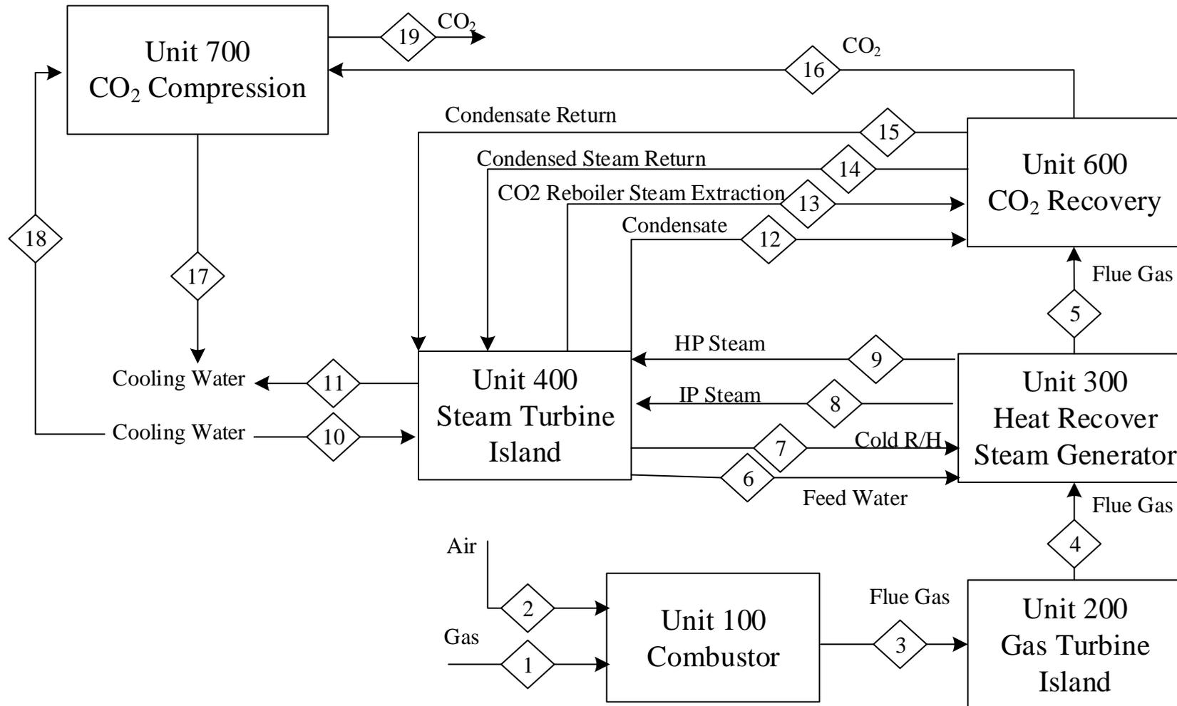
Apx Figure A.23 NGCC power plant with capture using evaporative (EV) cooling and same or air-cooled (AC) capture plan (Case 2.1B: NGCC-EV-PCC or Case 2.1C: NGCC-EV-PCC-AC)
