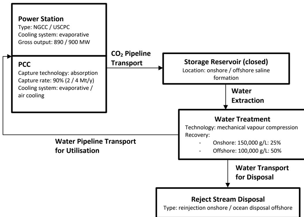
**Figure 2** Flow diagram of the CCS-Water-Nexus Scenario with water treatment (CCS-water-nexus scenario) and utilisation in the power station with capture
