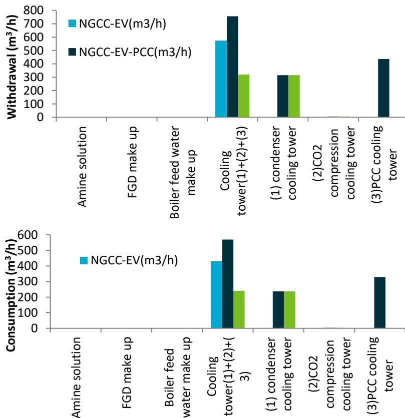
Figure 2-12 Absolute water withdrawal and consumption rates for the NGCC using evaporative cooling systems comparing Case 2.1A (NGCC-EV), Case 2.1B (NGCC-EV-PCC), and Case 2.1C (NGCC-EV-PCC-AC)
