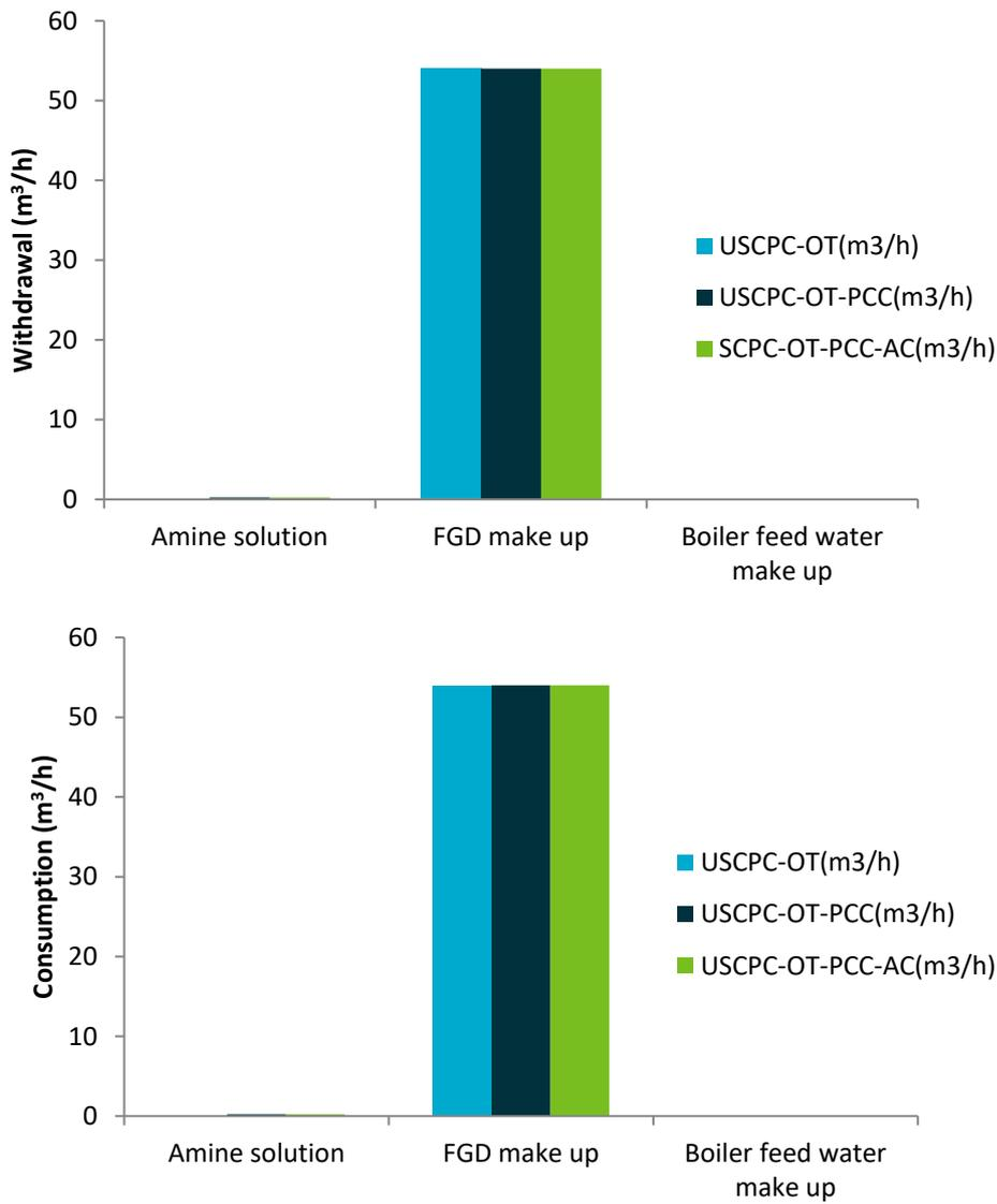
**Figure 5 Absolute water withdrawal and consumption rates for the USCPC using once-through seawater cooling systems (Cases 1.2A/B/C)**
