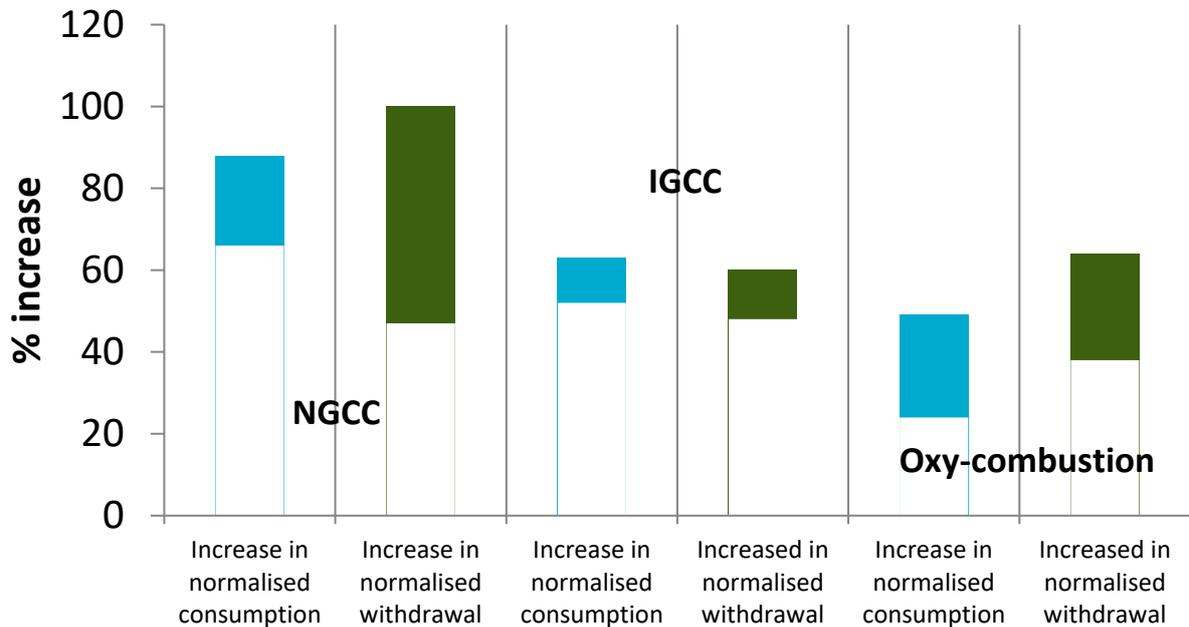
Figure 1-17 Range in increases in normalised consumption and withdrawal for recirculating cooling; NGCC, IGCC, oxy-combustion power plants with capture
