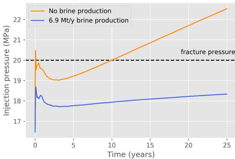
**Figure 10** Bottomhole pressure for the onshore model with closed boundary conditions comparing injection with brine production (injection case On-4c-2-2, blue curve) and without brine production (injection case On-4c-2, orange curve) for a CO<sub>2</sub> injection rate of 2 Mt/year
