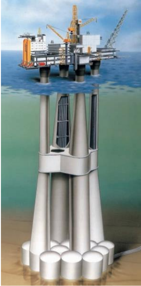
Figure 10-12 Troll A, Fixed Platform 374
