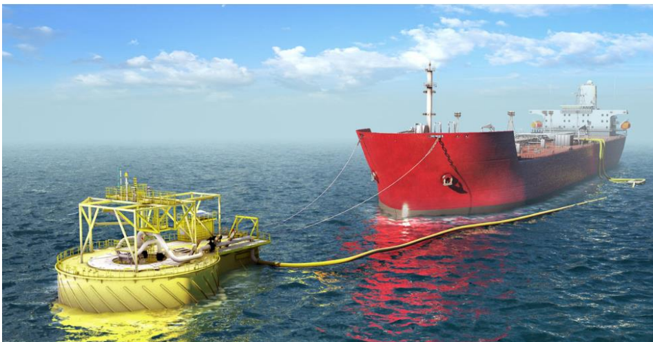
Figure 10-17 Turret Buoy Loading. 384
