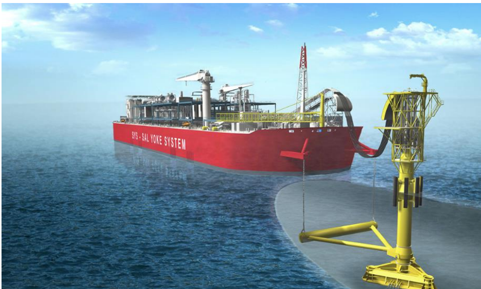
Figure 10-21 Soft Yoke System. 384
