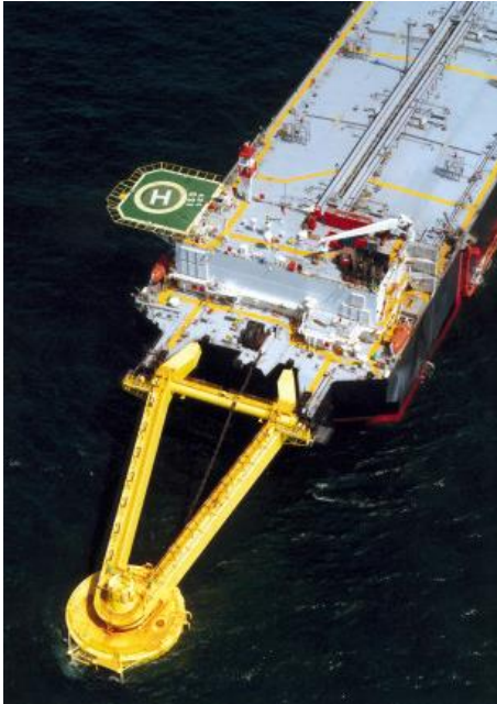
Figure 10-22 Rigid Arm System 385
