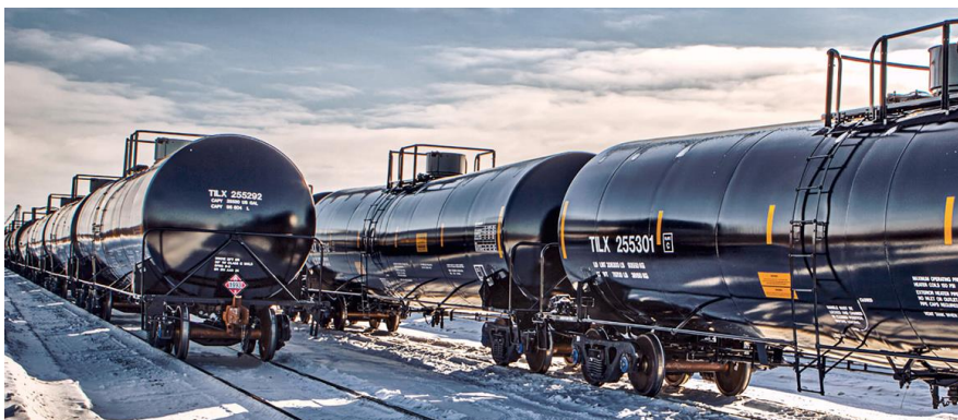
Figure 61: Transport of CO 2 via rail would be similar to existing LNG rail transport shown above 172
