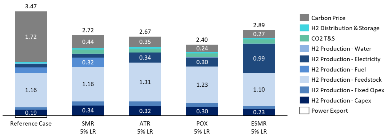
Figure 74: LCOH for natural gas based blue hydrogen production in the Netherlands compared against SMR without CCS reference case in 2050 (€/kgH 2 ) *CO 2 Price in the Netherlands in 2050 - €162.46/tCO 2
