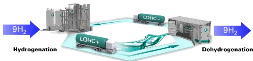
Figure 28: LOHC utilisation cycle 54
