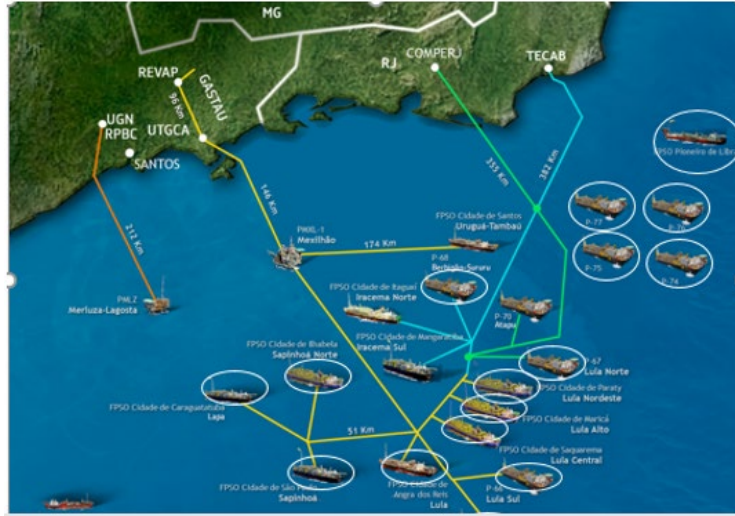
Figure 2.4. Petrobras' FPSOs with CO 2 separation & injection facilities for EOR in the Santos basin (Pre-Salt) offshore Brazil.
