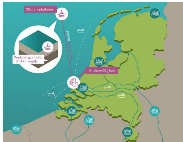
Figure 2.11. Map showing Aramis project location and concept for capture, transport, and storage.
