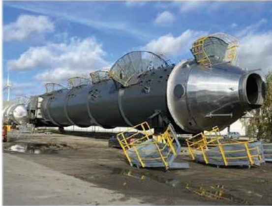
Absorber photographed at construction site in Holland
