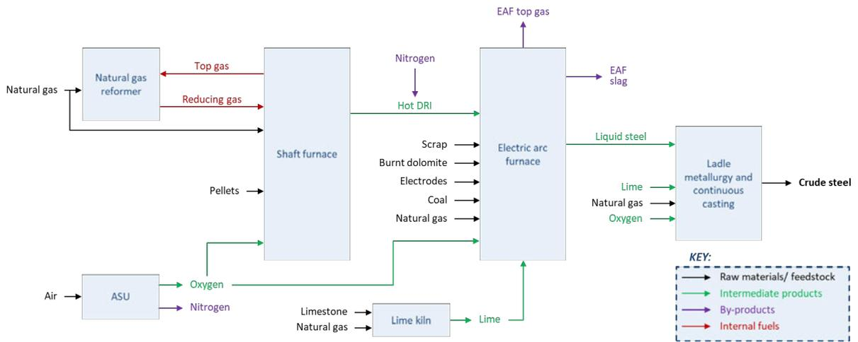
Figure 14: Natural gas-based direct reduction steel plant material process flow
