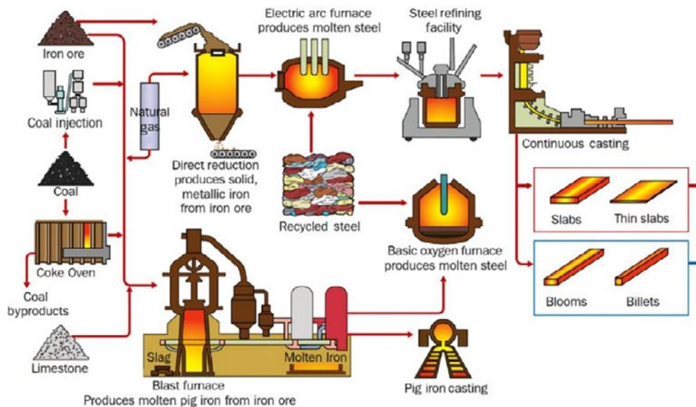
**Figure 4: Ironmaking and steelmaking flowsheet for different production routes (Yang, Raipala and Holappa, 2014)**
