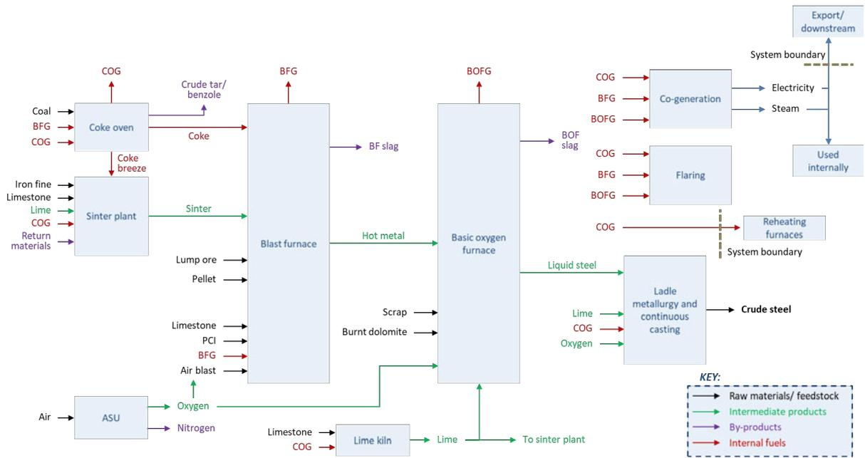
Figure 13: Integrated steel mill material process flow<sup>12</sup>
