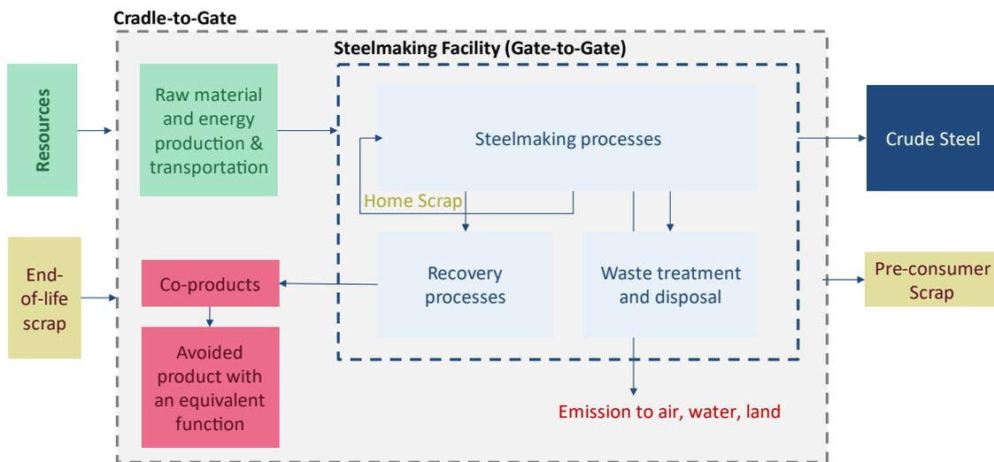
Figure 1: System Boundary for Cradle-to-Gate, adapted from World Steel Inventory
