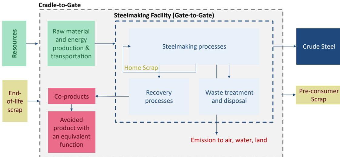
**Figure 35: System Boundary for Cradle-to-Gate. Adapted from World Steel Inventory (2017)**
