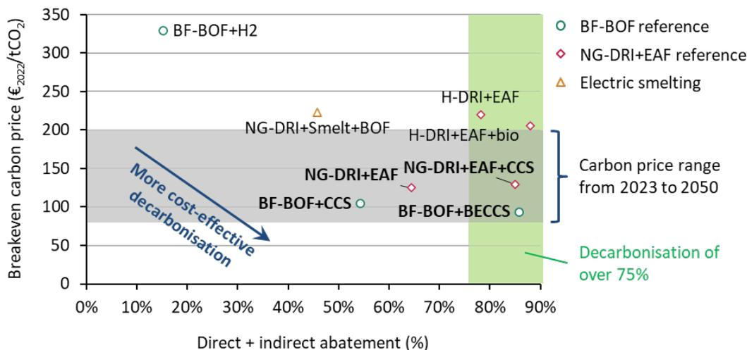
Figure 3: Breakeven carbon price and emissions intensity reduction for different steelmaking routes
