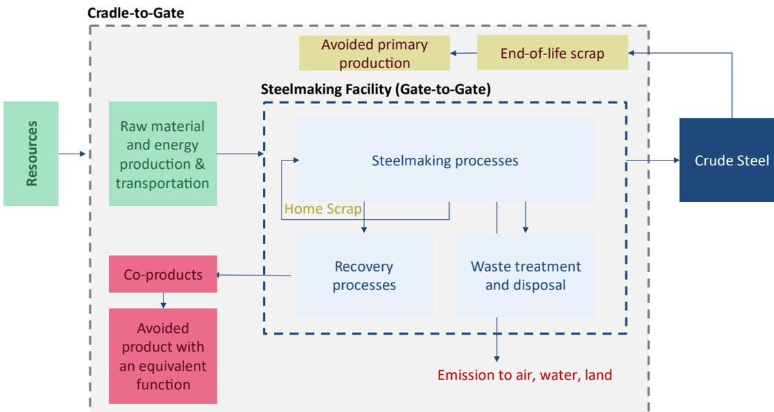
**Figure 36: System Boundary for Cradle-to-Gate with Recycling**
