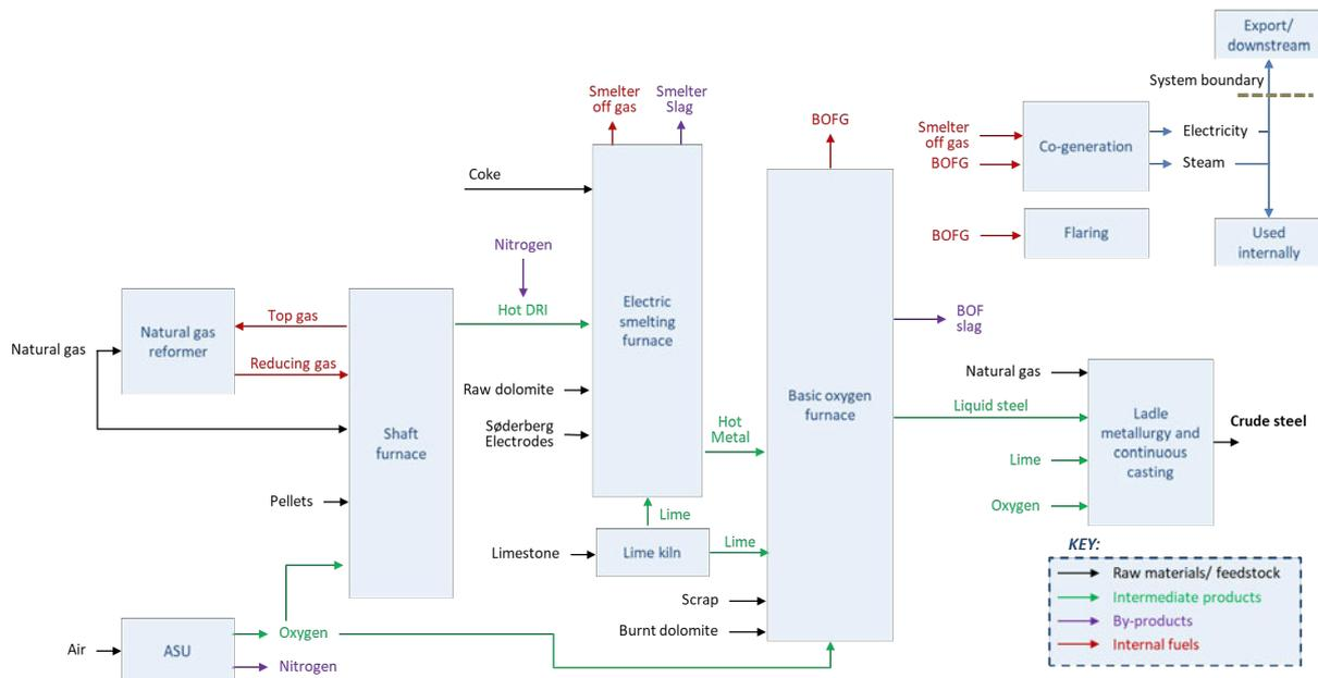
**Figure 15: Material process flow for a steel mill with a direct reduction plant and electric smelting furnace**
