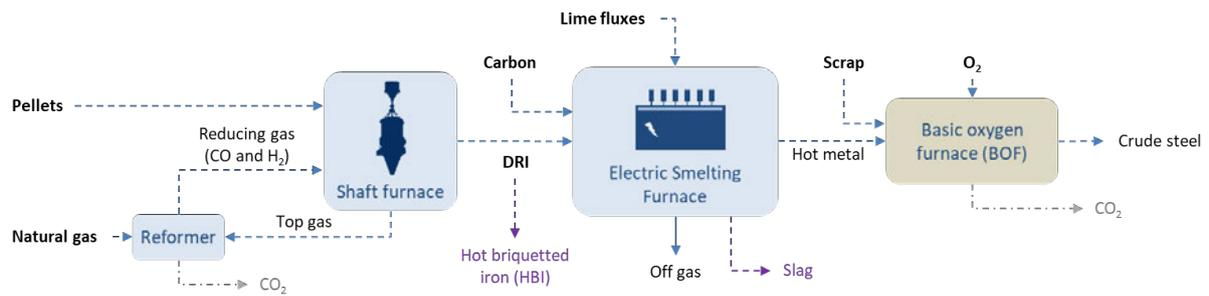
**Figure 9: Natural gas-based DRI with electric smelting furnace (ESF) and BOF pathway**
