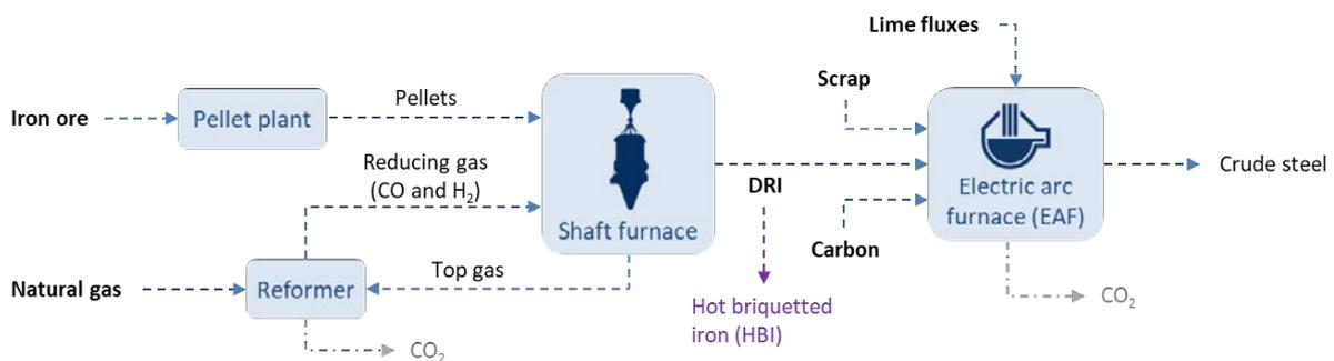
**Figure 7: Natural gas-based direct reduced iron (DRI) to electric arc furnace (EAF) pathway**
