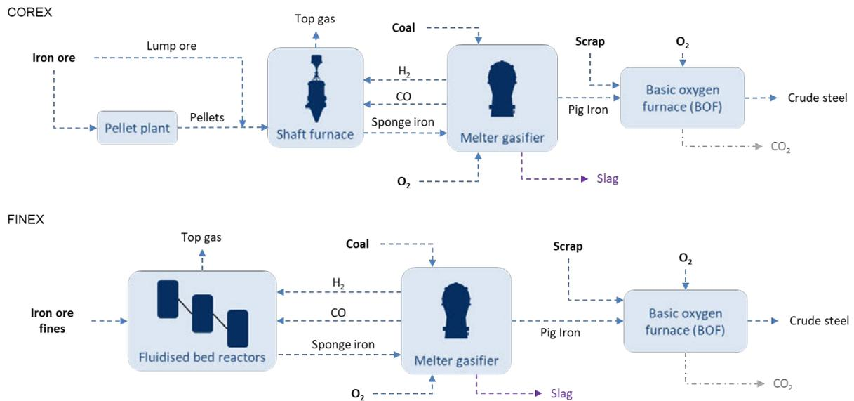
Figure 10: Smelting reduction pathways for Corex and Finex
