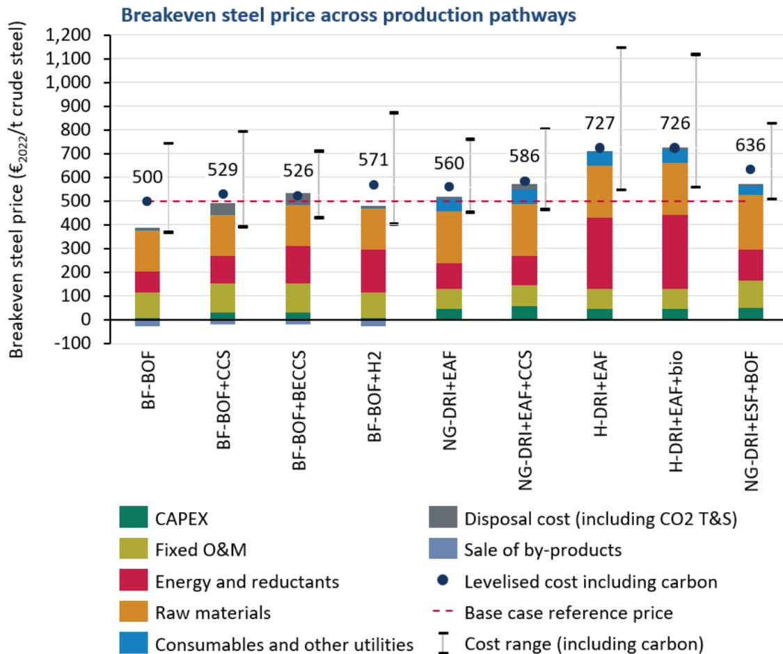
Figure 2. Breakeven steel price across production methods
