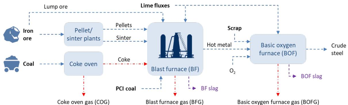
**Figure 6: Basic oxygen steelmaking (BOS) pathway**
