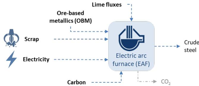
**Figure 8: Scrap-based EAF or secondary steel pathway**
