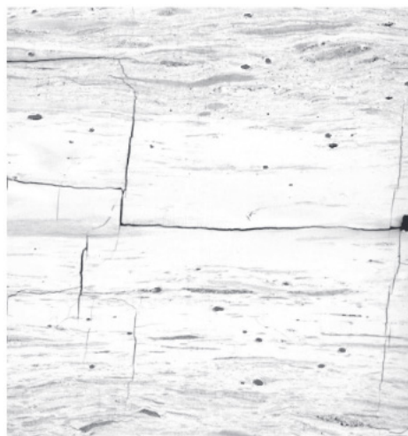
Figure 40: \mu CT image of connected porosity and fractures in a bituminous coal sample (Golab et al., 2012)
