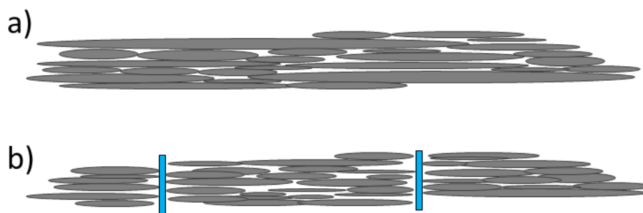
Figure 13: Schematic representation of a shale with all clay particles perfectly aligned along the bedding, which forms a very good seal (top) and a leaking seal (bottom). Leakage pipes or capillary pipes are represented in blue low aspect ratio connected pores across the bedding.
