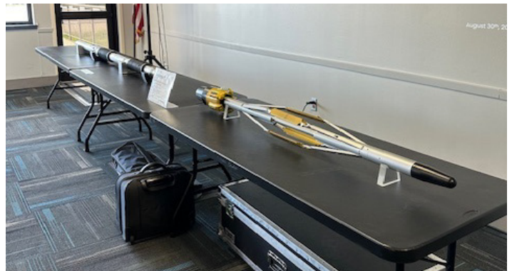
A selection of logging tools as demonstrated by Baker Hughes (Proxima and RCX Straddle Packer Microfrac)
